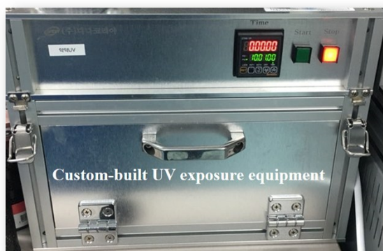
Figure S1. Camera image of Custom-built UV exposure equipment and UV exposure process to sandwich-like assembly of micro/nano molds.
