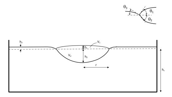
We will introduce now a similar analysis developed by Phan [19] to estimate the FC-72 lens thickness and how much it sinks inside the ethanol substrate. The floating condition for the lens Phan [19] requires that:
