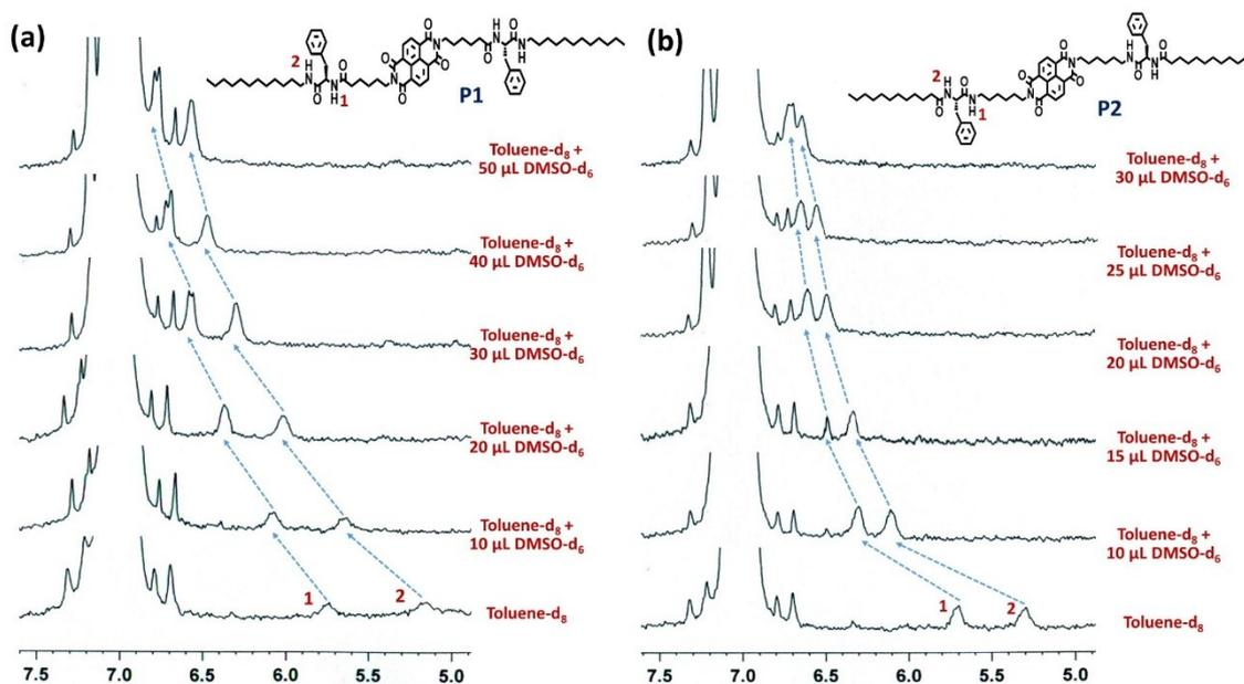
**Fig S12.** <sup>1</sup>H NMR spectrum of (a) **P1** and (b) **P2** (in toluene-d<sub>8</sub>) upon gradual addition of DMSO-d<sub>6</sub> (at 85 °C).
