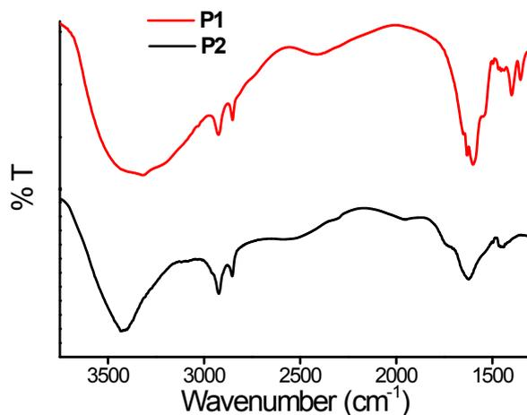
**Fig. S10** Extended FTIR spectra of xerogels **P1** and **P2** gels prepared from  $\text{CHCl}_3$ -MCH (5:95 v/v) mixture.
