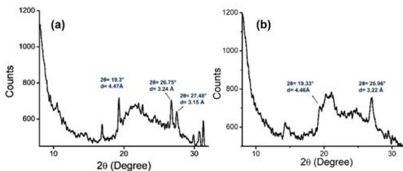
**Fig. S11** Powder X-ray diffraction pattern obtained from (a) **P1** and (b) **P2** xerogels prepared in gelling solvent (CHCl<sub>3</sub>:MCH= 5:95 v/v).
