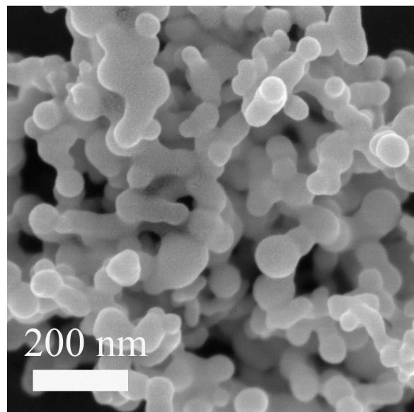
**Fig. S10** The SEM images of commercial Si nanoparticles with an average size of ~70 nm.
