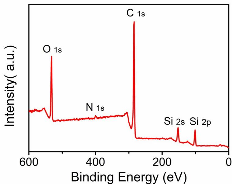
**Fig. S11** Survey XPS spectra of as-prepared Si/SiO<sub>x</sub>-DSHSs.
