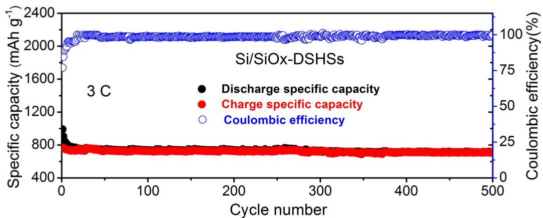
**Fig. S15** The cycling performance of Si/SiO<sub>x</sub>-DSHSs electrodes for 500 cycles at 3 C with a reversible capacity of around 750 mAh g<sup>-1</sup> and an excellent cycle retention of 94.5% after 500 cycles.
