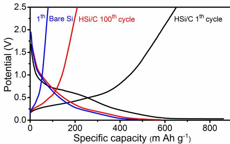
**Fig. S14** Charging/discharging profiles of bare Si and carbon coated hollow Si nanosphere (HSi/C) electrodes at different cycles at a high current rate of 5 C.
