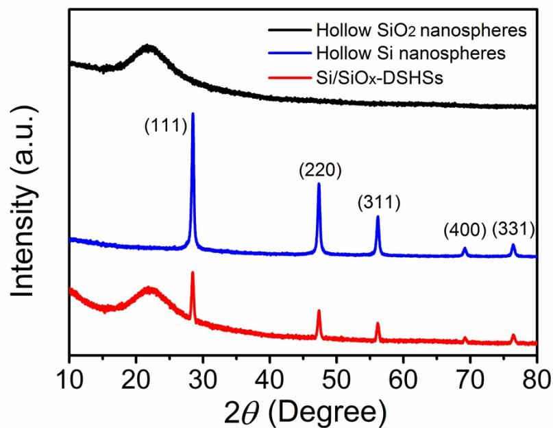
**Fig. S5** XRD patterns of Si hollow nanospheres, SiO<sub>2</sub> hollow nanospheres and Si/SiO<sub>x</sub>-DSHSSs.
