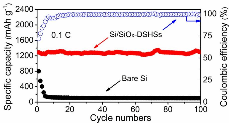
**Fig. S13** The cycling performance of bare Si and Si/SiO<sub>x</sub>-DSHSs electrodes for 100 cycles at 0.1 C.
