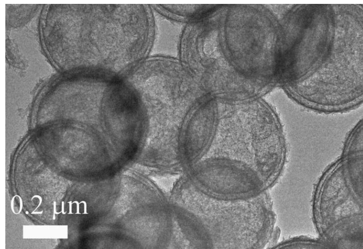
**Fig. S4** Low magnification TEM image of Si/SiO<sub>x</sub>-DSHSSs.
