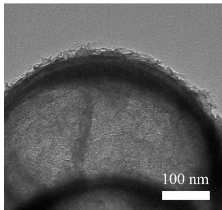
**Fig. S16** TEM image of cycled Si/SiO<sub>x</sub>-DSHSs electrode, showing structural integrity of carbon shell and thin SEI layer.
