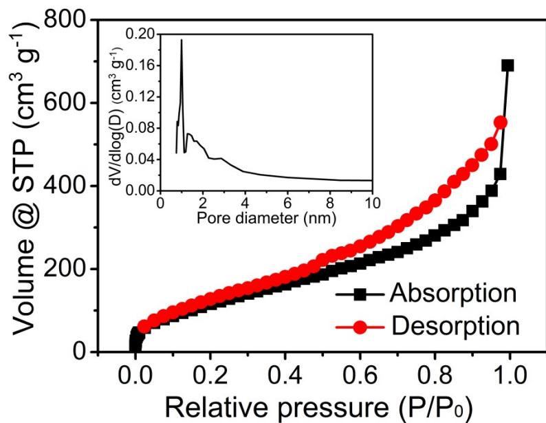
**Fig. S8** Nitrogen adsorption and desorption isotherm of the Si/SiO<sub>x</sub>-DSHSs alongside its porosity information.
