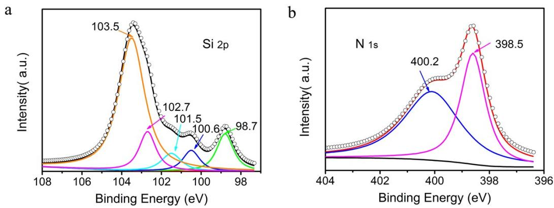
**Fig. S12** XPS spectra of the Si/SiO<sub>x</sub>-DSHSs (a) Si 2p signal and (b) N 1s signal.
