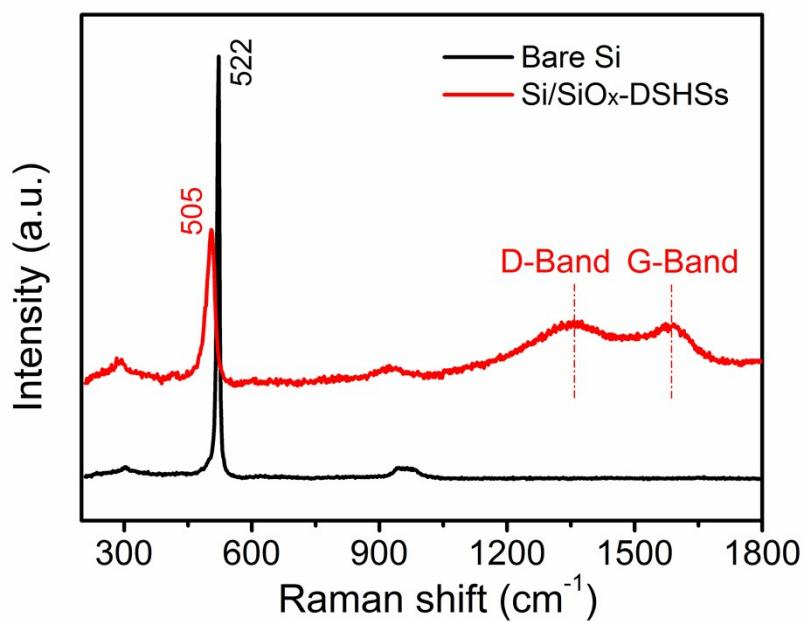
**Fig. S6** Raman spectra of the bare Si and Si/SiO<sub>x</sub>-DSHSs.
