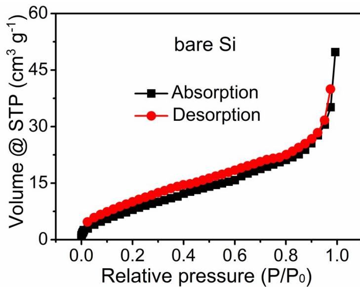
**Fig. S9** N<sub>2</sub> adsorption–desorption isotherm of commercial Si nanoparticles.
