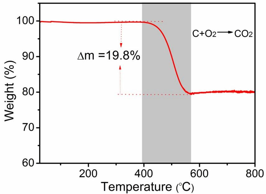
**Fig. S7** Thermogravimetric analysis curve of the Si/SiO<sub>x</sub>-DSHSs.
