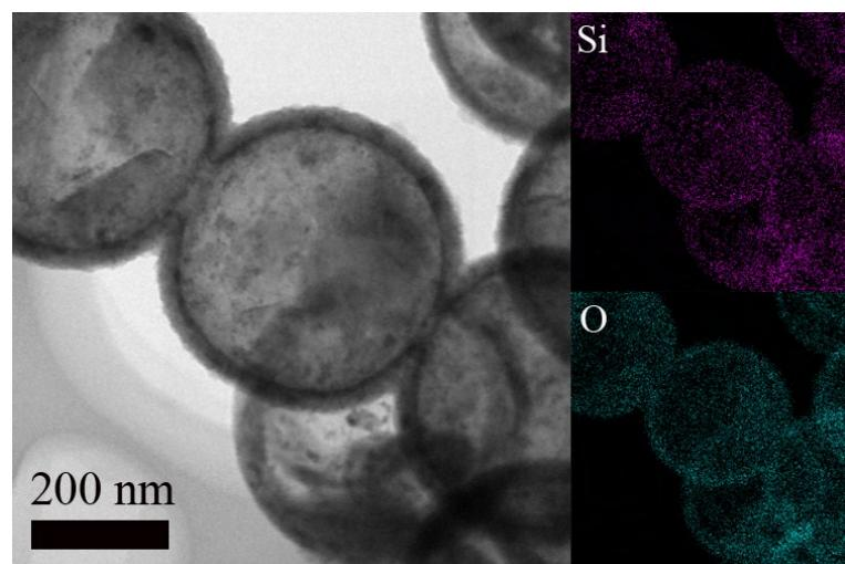
**Fig. S3** TEM image of Si/SiO<sub>2</sub> and its corresponding EDS elemental mapping.
