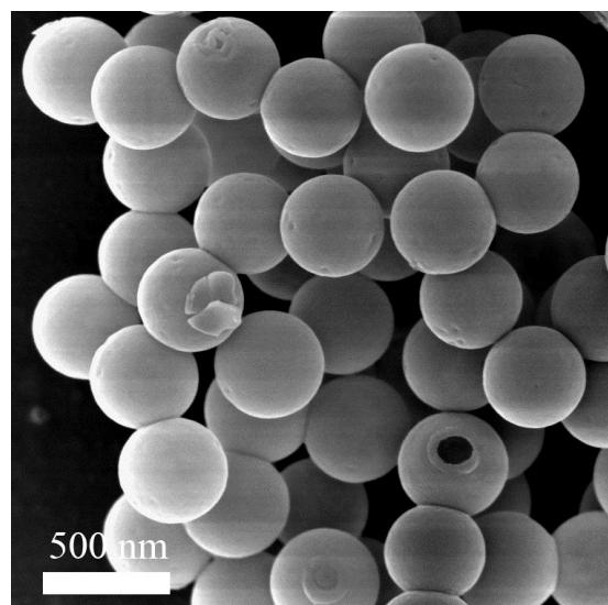
**Fig. S1** SEM image of SiO<sub>2</sub> hollow nanospheres with an average diameter of ~450 nm.
