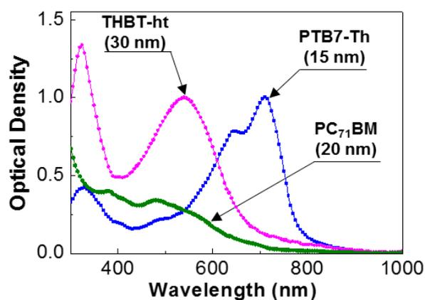
**Fig. S2.** Optical absorption spectra for the pristine films (PTB7-Th, PC<sub>71</sub>BM, and THBT-ht) coated on the quartz substrates. The thickness of each film is given below the name of material.
