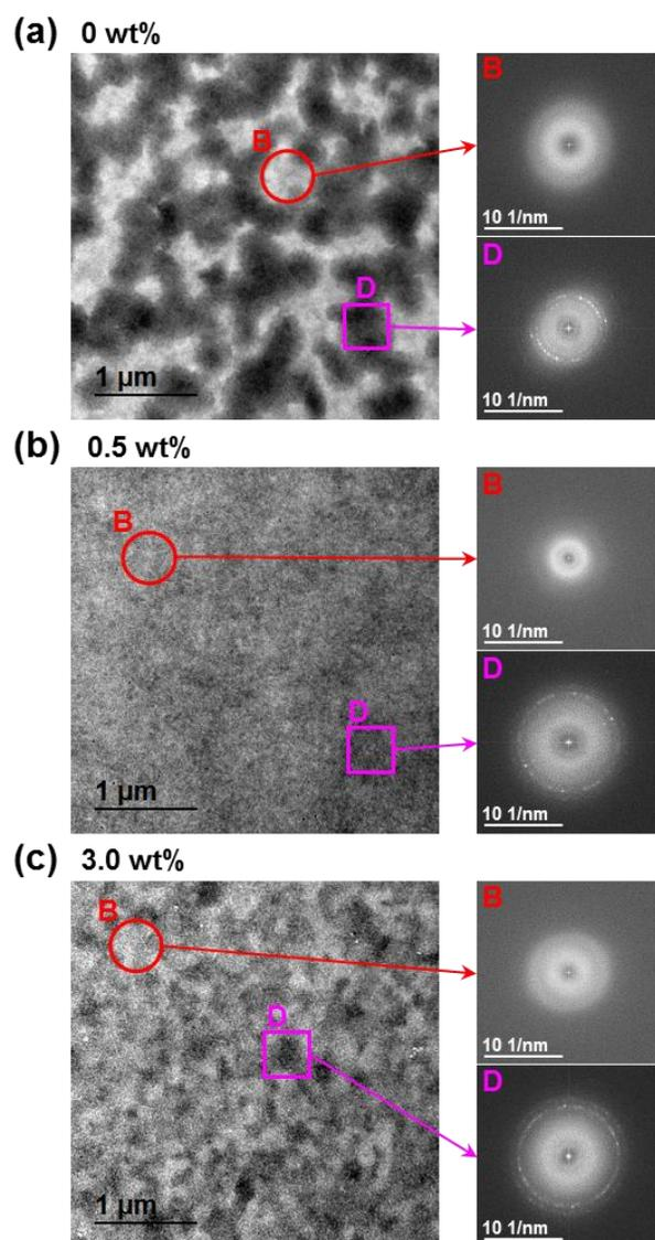
**Fig. S5.** TEM images, which were measured on the different position from Figure 5, for the BHJ (PTB7-Th:PC<sub>71</sub>BM) films with the THBT-ht additive. The selected-area electron diffraction (SAED) patterns (right) were measured by focusing on the bright (B) and dark (D) parts in the BHJ films.
