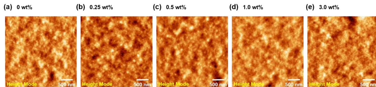
**Fig. S4.** 2D height-mode AFM images for the BHJ (PTB7-Th:PC<sub>71</sub>BM) layers with the THBT-ht additive, which were coated on the ZnO/ITO-glass substrates: (a) THBT-ht = 0 wt%, (b) 0.25 wt%, (c) 0.5 wt%, (d) 1.0 wt%, (e) 3.0 wt%. The scan size of the AFM images was 3  $\mu\text{m}$   $\times$  3  $\mu\text{m}$ .
