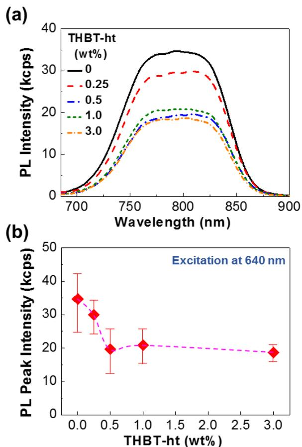
**Fig. S1.** (a) PL spectra for the binary blend (PTB7-Th:THBT-ht) films coated on the quartz substrates (excitation wavelength = 640 nm). (b) PL peak intensity as a function of the THBT-ht content for the binary blend (PTB7-Th:THBT-ht) films.
