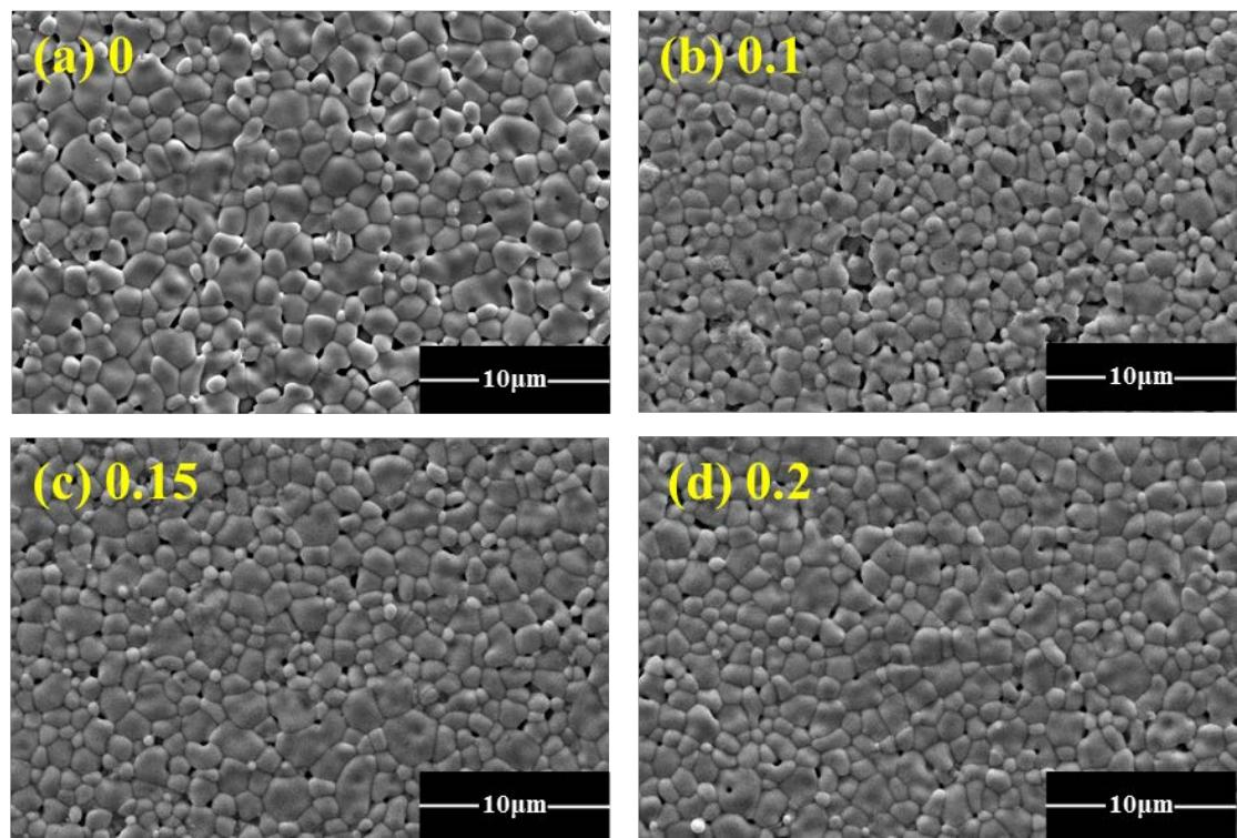
Fig.S5. SEM images of the samples PMN-PMS-PZT: xAlN:(a)  $x=0$ , (b)  $x=0.1$ , (c)  $x=0.15$ , (d)  $x=0.2$  wt.%.
