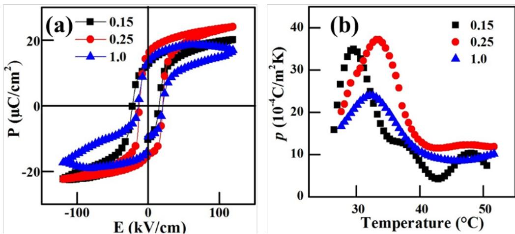
Fig.S8. (a) P-E loops of the samples with various AlN contents: 0.15, 0.25, 1.0 wt.%. (b) Temperature-dependent pyroelectric coefficient of the corresponding samples
