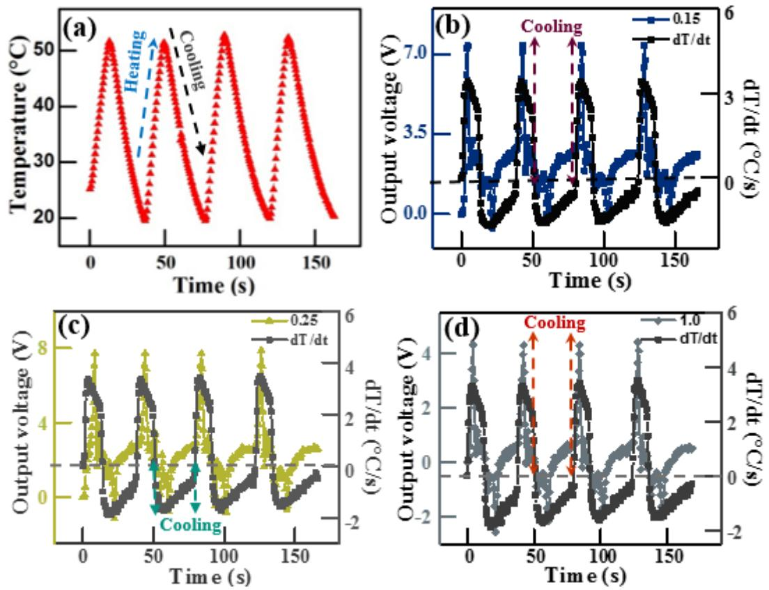
Fig.S10. (a) Temperature variation as a function of time along with corresponding output voltage and rate of temperature change for (b) 0.15 wt.%, (c) 0.25 wt.%, and (d) 1.0 wt.%, respectively, when they are under heating and cooling.
