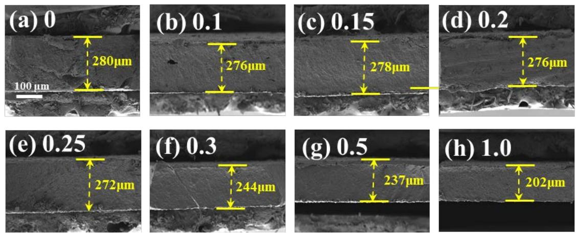
Fig.S9. The thickness of the samples PMN-PMS-PZT: xAlN:(a) x=0, (b) x=0.1, (c) x=0.15,(d) x=0.2, (e) x=0.25, (f) x=0.3, (g) x=0.5, (h) x=1.0 wt.%.
