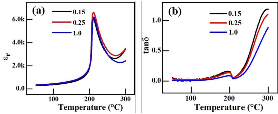
Fig.S7. Temperature-dependent dielectric properties of the materials with various AlN contents: 0.15, 0.25, 1.0 wt.%. (a) Relative permittivity (dielectric constant) and (b) dielectric loss of the corresponding materials at 1 kHz.
