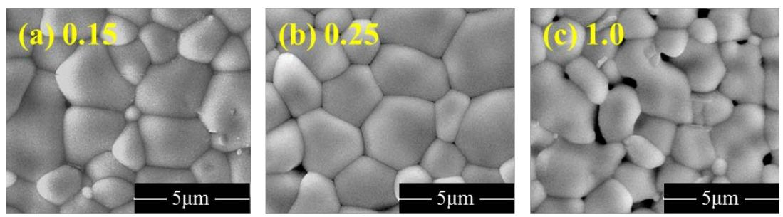
Fig.S4. SEM images of the samples PMN-PMS-PZT: xAlN:(a)  $x=0.15$ , (b)  $x=0.25$ , (c)  $x=1.0$  wt.%.
