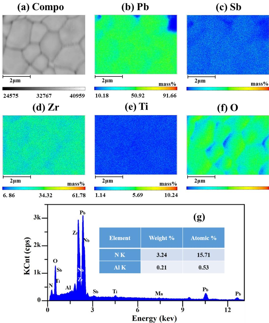
Fig.S6. SEM micrographs of the samples PMN-PMS-PZT: 0AlN. (a) Microstructural image of the composite. Scale bar is 2.0 $\mu$ m (b)-(f) the corresponding elemental distribution. (g) The energy-dispersive spectrum of the PMN-PMS-PZT: 0.2AlN sample.
