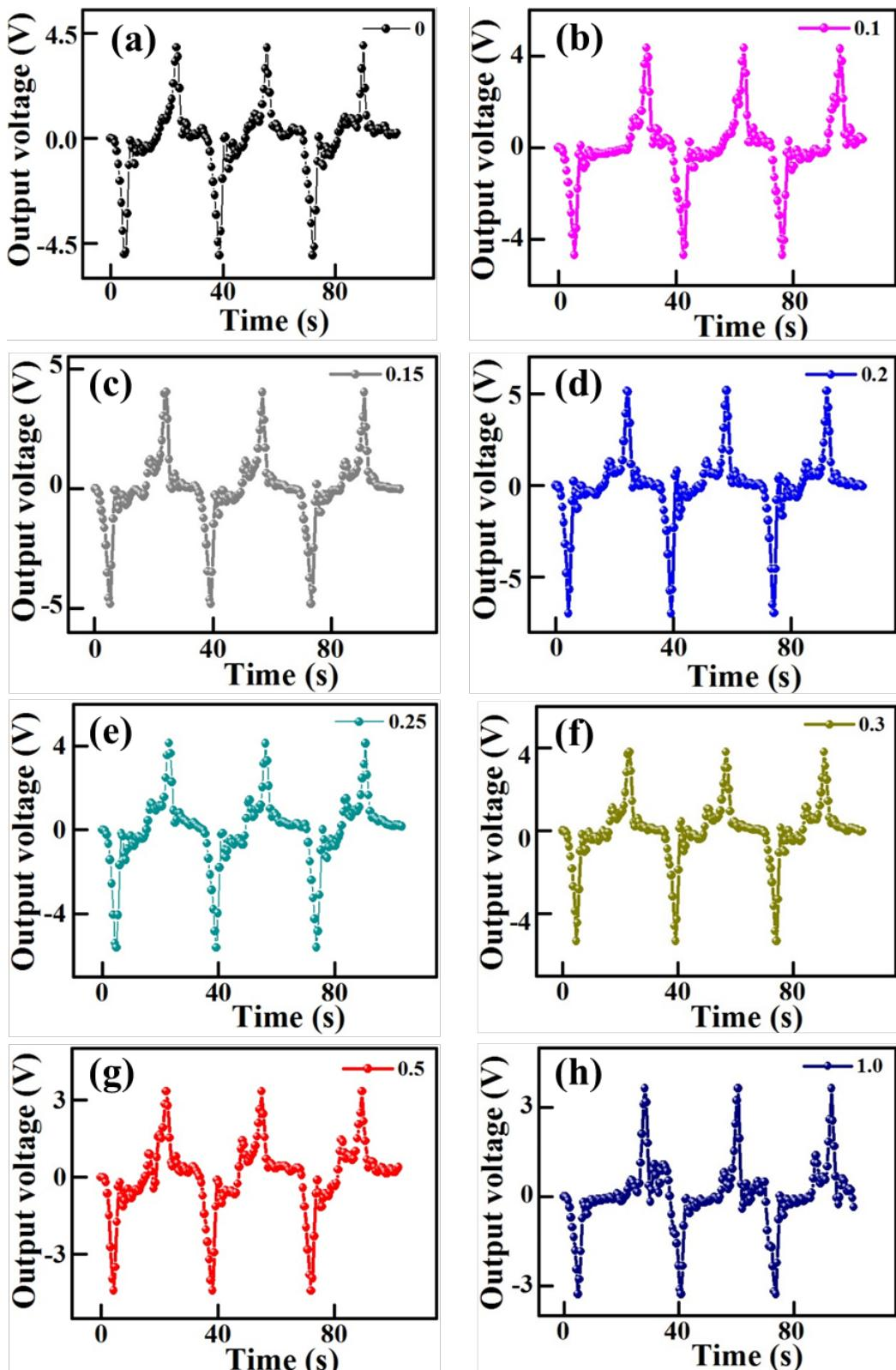
Fig.S11. (a) Output voltage for the samples with 0 wt.% (a), 0.1 wt.% (b), 0.15 wt.% (c), 0.2 wt.% (d), 0.25 wt.% (e) 0.3 wt.% (f), 0.5 wt.%, and 1.0 wt.% AlN contents, respectively, when the two electrodes of pyroelectric devices reversibly connecting to the circuits.
