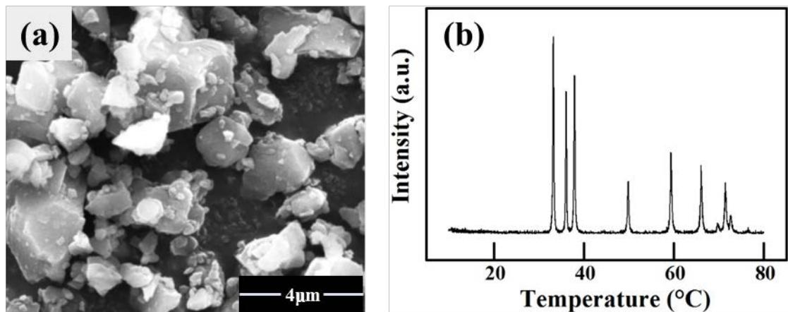
Fig.S2. (a) SEM image and (b) XRD spectrum for the initial AlN power
