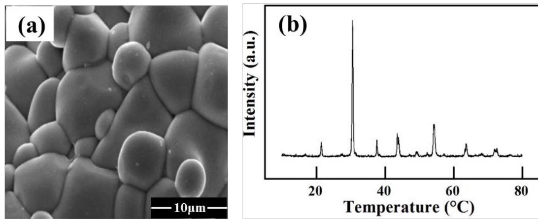
Fig.S1. (a) Scanning electron microscopy (SEM) and (b) X-ray diffraction (XRD) spectrum of the pure PMN-PMS-PZT sample after one-step sintering.
