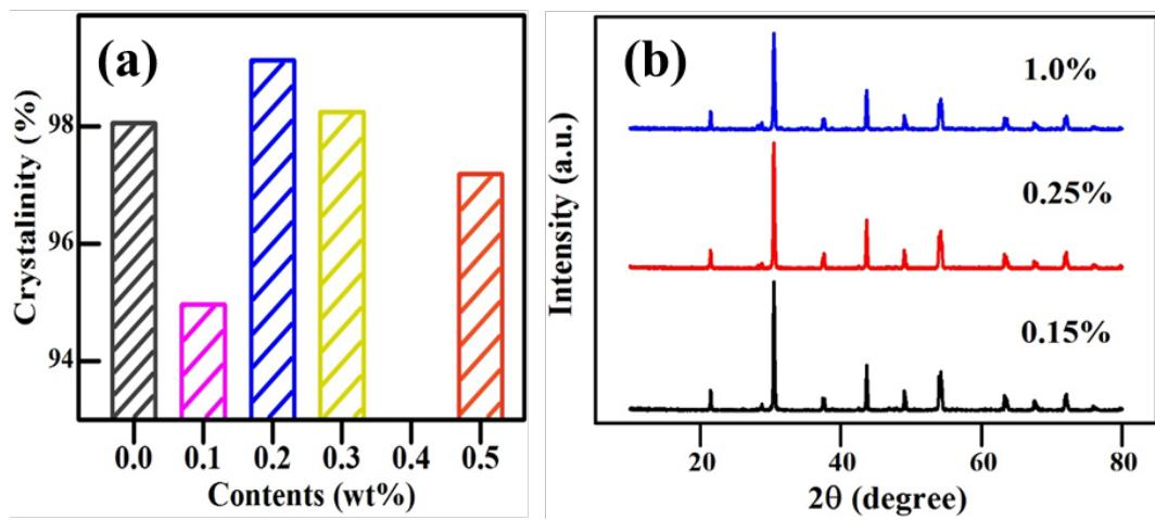
Fig. S3. (a) Crystallinity of the samples with a variation of AlN contents: 0, 0.1, 0.2, 0.3, 0.5 wt.%.
