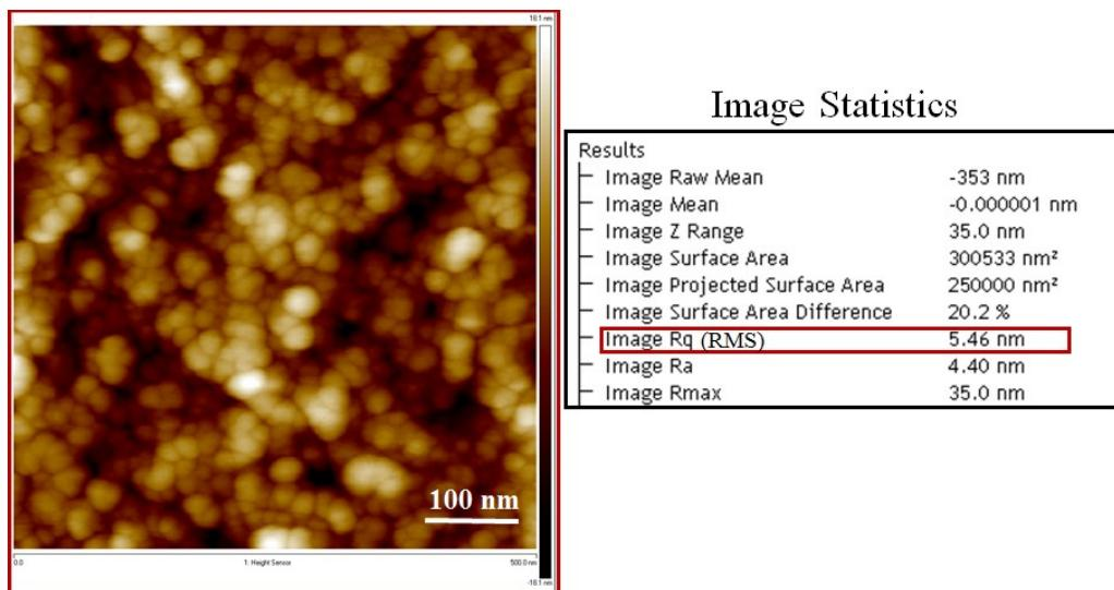
Fig. S2: Atomic force microscopy image of G-TiO<sub>2</sub> film spin-coated on ITO.
