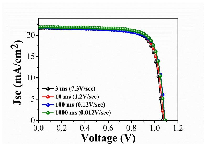
Fig. S5:  $J$ - $V$  curves of the G-TiO<sub>2</sub> based PSCs measured with different delay times.
