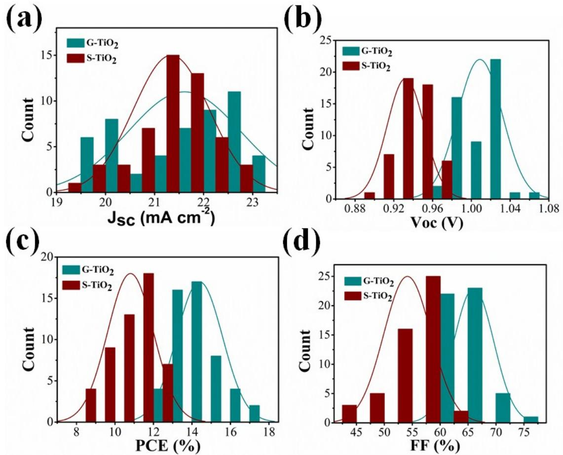
Fig. S8: Histograms of the performance (current-density, open-circuit voltage, power conversion efficiency, and fill factor) of 51 G-TiO<sub>2</sub> and S-TiO<sub>2</sub> devices, measured under 1 Sun light illumination (100 mW cm<sup>-2</sup>).
