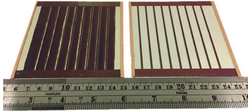
Fig. S6: Photograph of large-area ( $25.2\text{ cm}^2$ ) solar submodules incorporating G-TiO<sub>2</sub> as the ETL.
