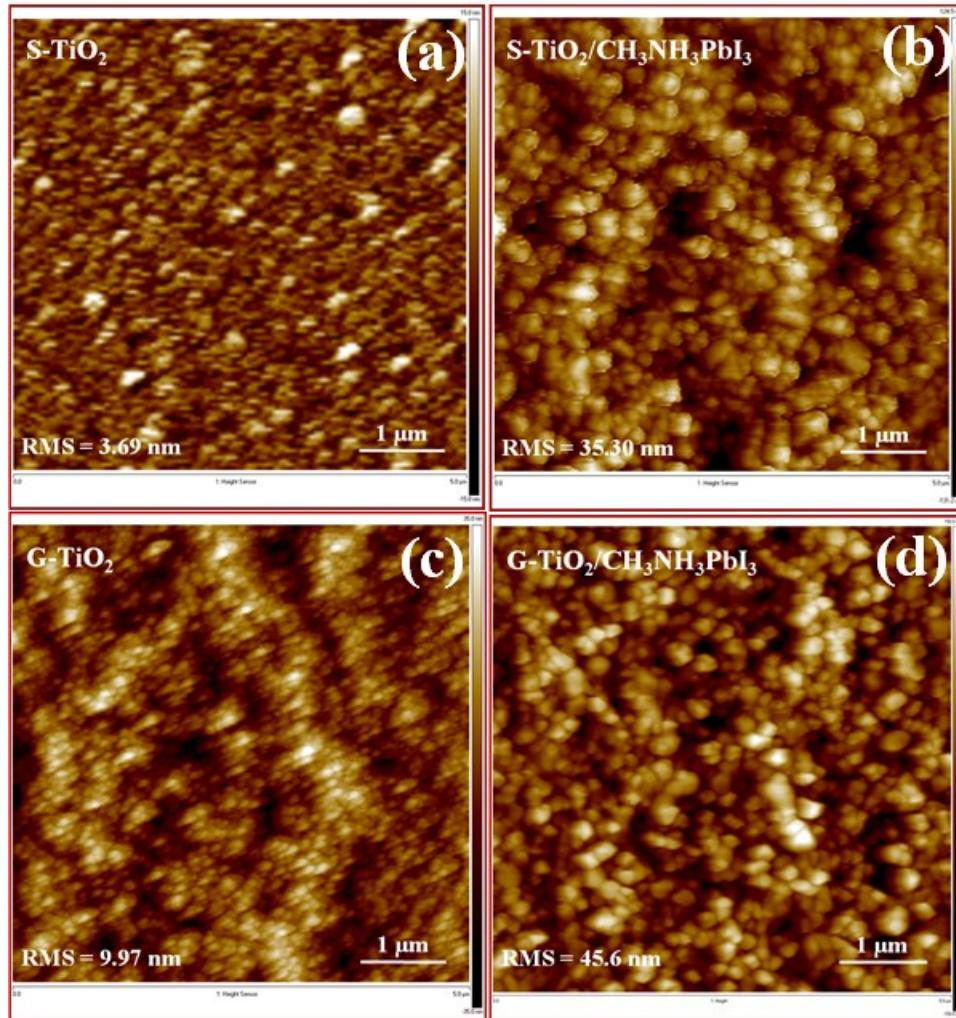
Fig. S10: AFM images of (a) glass/FTO/S-TiO<sub>2</sub>, (b) glass/FTO/S-TiO<sub>2</sub>/CH<sub>3</sub>NH<sub>3</sub>PbI<sub>3</sub>, (c) glass/ITO/G-TiO<sub>2</sub> and (d) glass/ITO/G-TiO<sub>2</sub>/CH<sub>3</sub>NH<sub>3</sub>PbI<sub>3</sub>.
