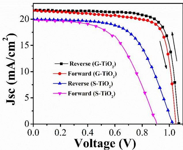
Fig. S4:  $J$ - $V$  curves of PSCs with the G-TiO<sub>2</sub> and S-TiO<sub>2</sub> as an electron transporting layers measured at reverse and forward scans.
