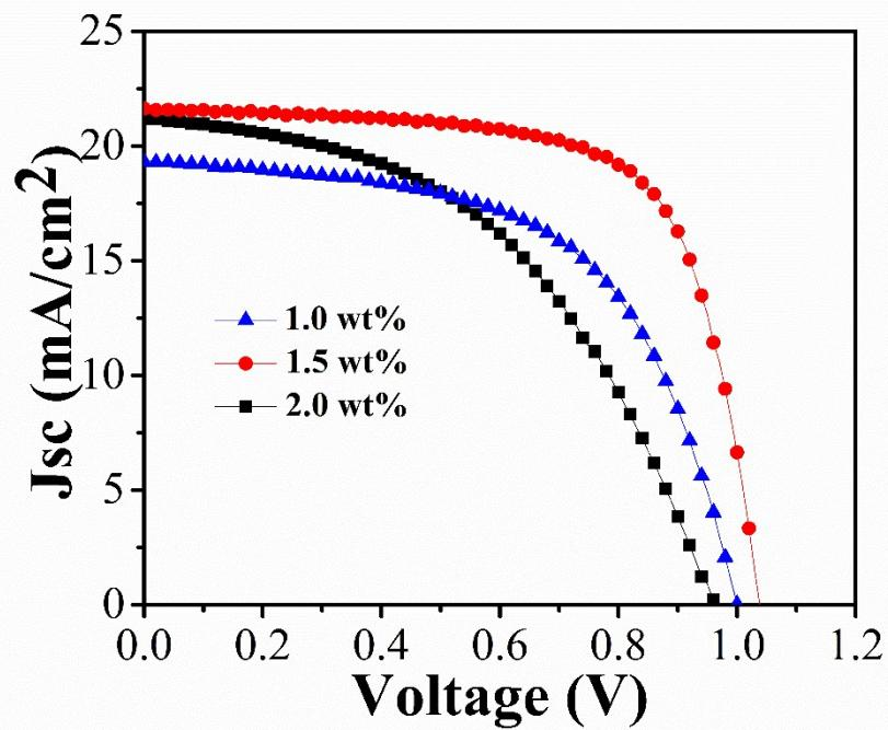
Fig. S11:  $J$ - $V$  curves of PSCs based on G-TiO<sub>2</sub> ETL with various thicknesses prepared from different concentrations of G-TiO<sub>2</sub> suspension.
