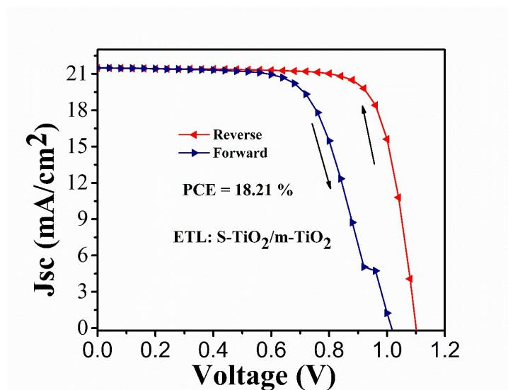
Fig. S3: *J-V* curve of PSCs with the device structure FTO/S-TiO<sub>2</sub>/m-TiO<sub>2</sub>/CH<sub>3</sub>NH<sub>3</sub>PbI<sub>3</sub>/spiro-MeOTAD/MoO<sub>3</sub>/Ag measured at reverse and forward scans.
