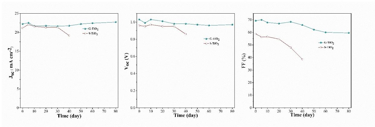
Fig. S7: Long-term stability tests of the best cell [ITO (or FTO)/G-TiO<sub>2</sub> (or S-TiO<sub>2</sub>)/CH<sub>3</sub>NH<sub>3</sub>PbI<sub>3</sub>/spiro-MeOTAD/MoO<sub>3</sub>/Ag] stored in a glove box under N<sub>2</sub>.
