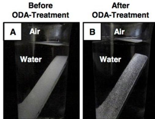
Fig. 53 A-B) Digital images of polymeric coating under water before (A) and after (B) covalent modification with octadecylamine (ODA). After covalent modification with ODA, the shiny interface of water/polymeric coating revealed the presence of metastable trapped air.
