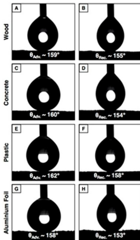
Fig. S6 A-H) Advancing (A,C,E,G) and receding (B,D,F,H) contact angle of beaded water droplets on polymeric coatings that are deposited on various substrates, including wooden block (A-B), concrete (C-D), plastic (E-F) and aluminium foil (G-H).
