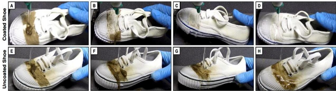
Fig. S5 Figure S5: A-H) Digital images illustrating the self-cleaning performance of the deposited dust on the superhydrophobic shoe (A-D) and uncoated shoe (E-H) under the stream of water.
