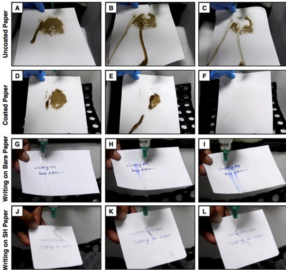
Fig. 54 A-F) Digital images illustrating the self-cleaning performance of deposited dust on uncoated (A-C) and superhydrophobic (D-F) printed paper (A-4 sized). G-L) Digital images showing the effect of exposures of manual write up to water stream, the write up on uncoated paper (G) was significantly damaged (H-I) with random spilling and spreading of ink, whereas no such spilling and spreading of ink was noted on superhydrophobic paper (J-L) under the stream of water.
