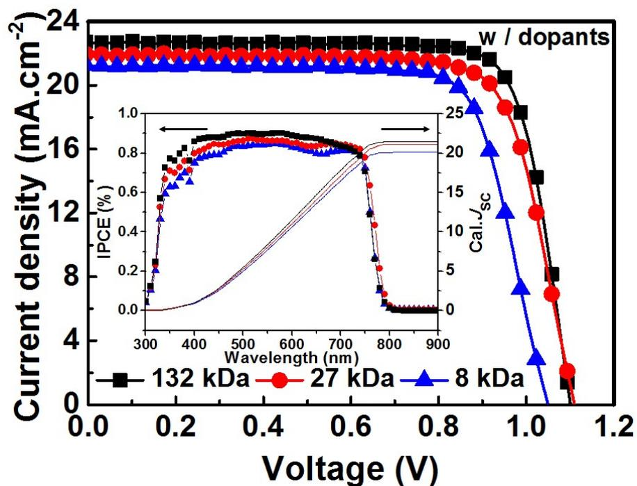
Fig. S5 J-V curve and IPCE of the perovskite solar cells with the series of doped asy-PBTBDTs
