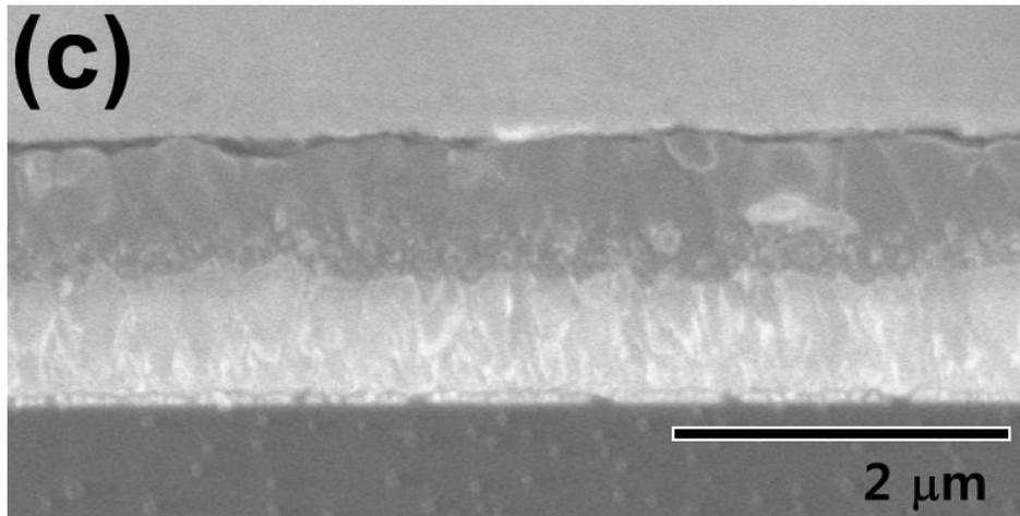
**Fig. S3** Cross-sectional scanning electron microscopy (SEM) image of perovskite solar cells employing the asy-PBTBDT of (a) 132 kDa, (b) 27 kDa, and (c) 8 kDa MW
