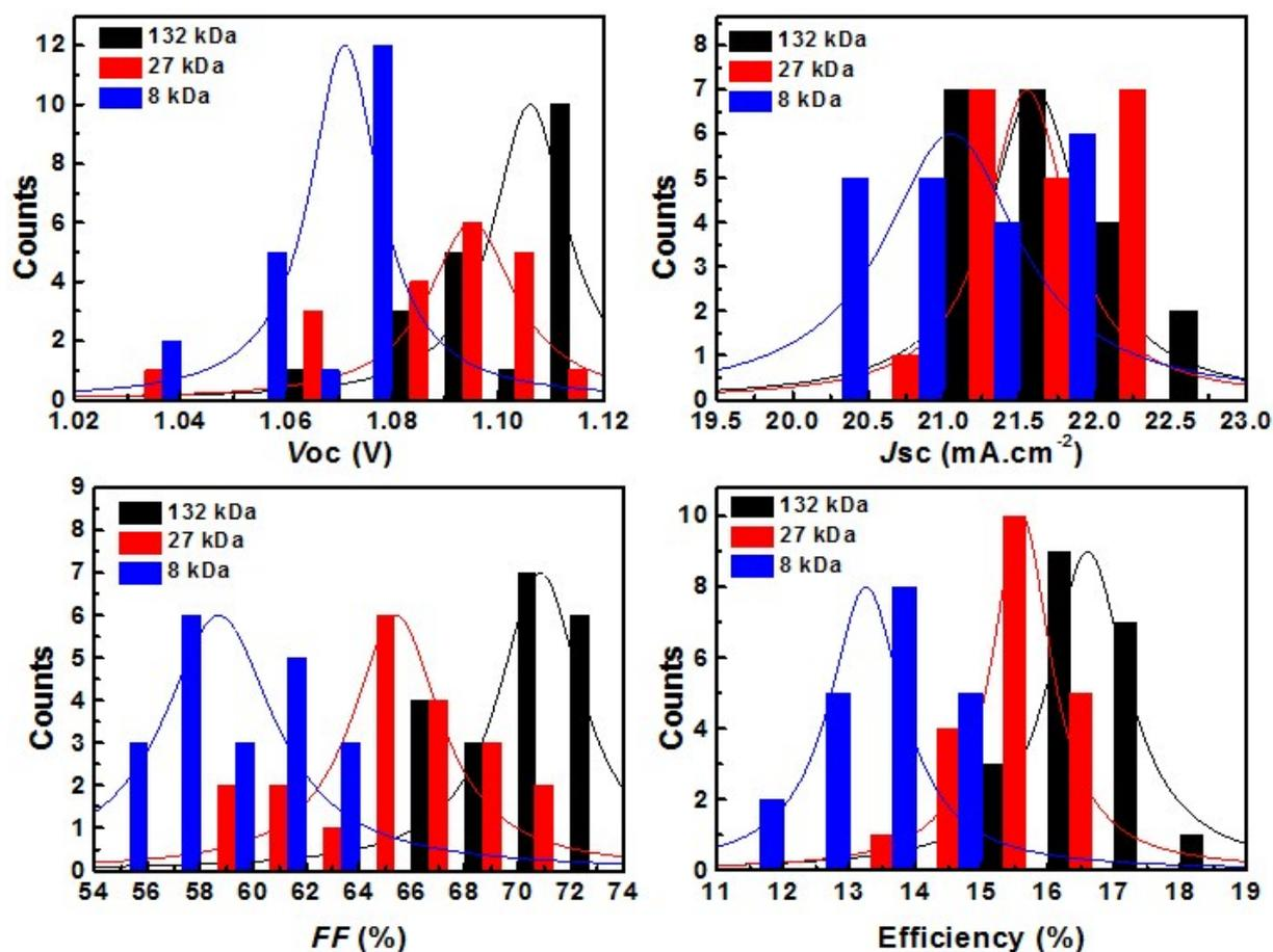
Fig. S4 Statics of perovskite solar cells devices for the series of dopant-free asy-PBTBDTs
