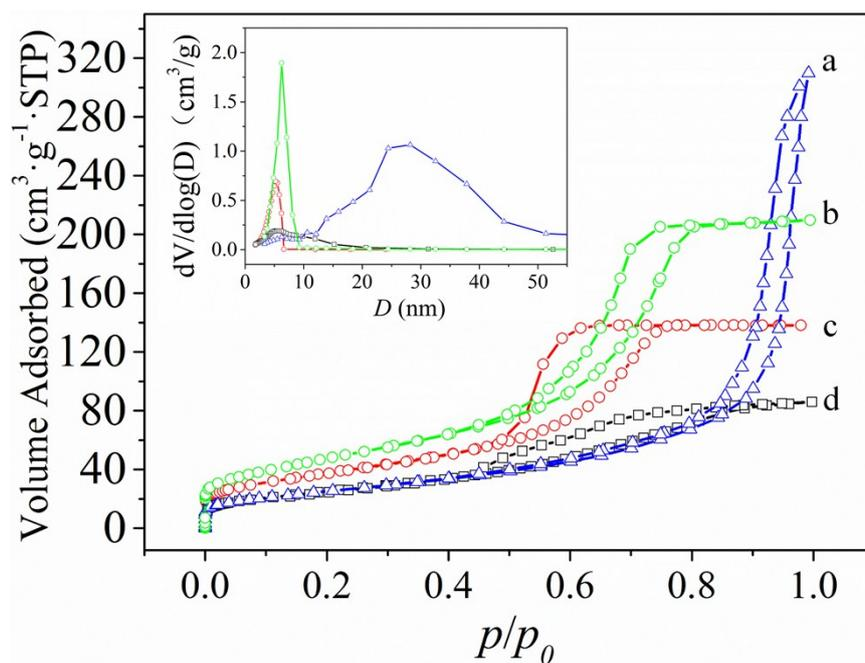
**Figure S5.** N<sub>2</sub> sorption isotherms and the inset corresponding pore size distribution curves of the control sample TiO<sub>2</sub>-NP (a), the control sample Meso-TiO<sub>2</sub>-EISA-350 (b), the representative sample UMWM-TiO<sub>2</sub>-150-350 (c), and the control sample UWM-TiO<sub>2</sub>-150-350 (d), respectively.
