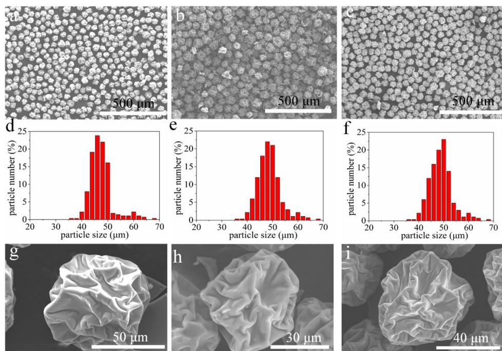
**Figure S1.** SEM images (a-c and g-i) and the corresponding particle size distributions (d-f) of the  $\text{TiO}_2$  samples obtained at a TTIP/F127 mass ratio of 2 : 6 (a, d, g), 3 : 6 (b, e, h), and 4 : 6 (c, f, i), respectively, with a drying temperature of 150 °C and a calcination of 350 °C.
