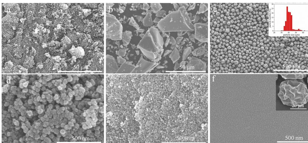
**Figure S4.** SEM (a-c) and HRSEM (d-f) images of the control sample  $\text{TiO}_2\text{-NP}$  (a, d), the control sample  $\text{Meso-TiO}_2\text{-EISA-350}$  (b, e), and the control sample  $\text{UWM-TiO}_2\text{-150-350}$  (c, f), respectively. Inset c is the corresponding particle size distribution. Inset f is a SEM image of an individual particle, the surface of which is partially shown in f.
