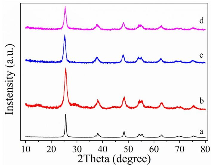
**Figure S3.** Wide-angle XRD patterns of the control sample  $\text{TiO}_2\text{-NP}$  (a), the control sample  $\text{Meso-TiO}_2\text{-EISA-350}$  (b), the representative sample  $\text{UMWM-TiO}_2\text{-150-350}$  (c), and the control sample  $\text{UWM-TiO}_2\text{-150-350}$  (d), respectively.
