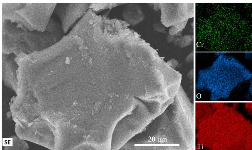
**Figure S2.** SEM image and the corresponding elemental maps of the representative sample UMWM-TiO<sub>2</sub>-150-350 after a typical adsorption process for Cr (VI).
