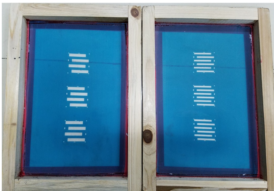
Fig. S12 Patterned screen meshes used to print the carbon electrode.
