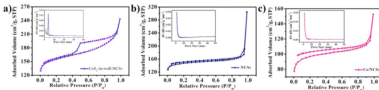
**Figure S3.** Nitrogen adsorption-desorption isotherms and insert: pore size distribution; a) CoS<sub>2</sub>-in-wall-NCSs, b) NCSs, and c) Co/NCSs.
