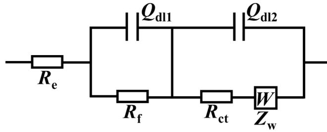
**Figure S5.** Equivalent series circuit for  $\text{CoS}_2$ -in-wall-NCSs samples as electrode materials for LIBs.  $R_e$ : Electrolyte resistance,  $R_f$ : Resistance of surface film on the electrodes,  $R_{ct}$ : Charge transfer impedance,  $Z_w$ : Warburg impedance,  $Q_{dl1}/Q_{dl2}$ : Constant phase element.
