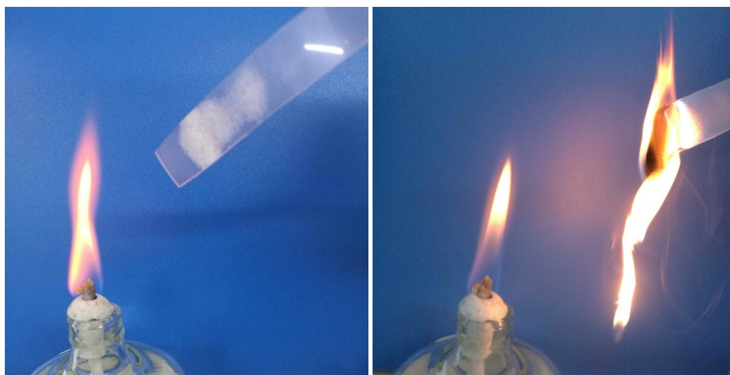
Fig. S10 Flaming behavior of a polypropylene plate.
