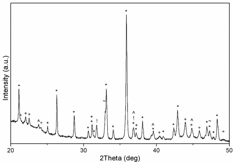
**Fig. S7.** XRD pattern of hydrogenated material after four absorption and three desorption cycles starting from the desorbed state.  $* = \text{Na}_2\text{Mg}_2\text{NiH}_6$ ;  $\sim = \text{NaMgH}_3$ ;  $! = \text{NaH}$ ;  $+ = \text{MgNi}_2$ .  $\lambda = \text{CuK}\alpha$ .
