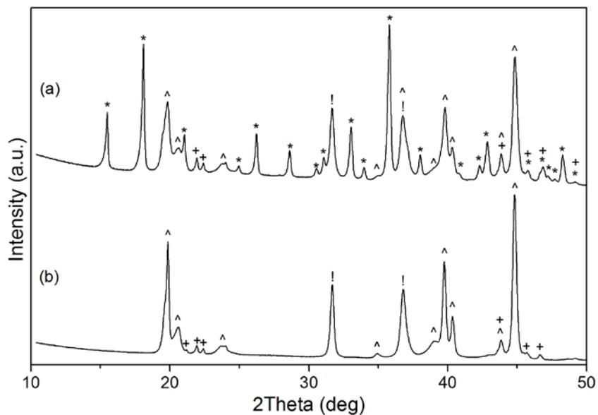
**Fig. S4.** Room temperature XRD patterns of Na<sub>2</sub>Mg<sub>2</sub>NiH<sub>6</sub> performed after heating to (a) 260 °C and (b) 330 °C *in vacuo* before quenching. \* = Na<sub>2</sub>Mg<sub>2</sub>NiH<sub>6</sub>; ^ = Mg<sub>2</sub>NiH<sub>0.3</sub>; ! = NaH; + = MgNi<sub>2</sub>. λ = CuK<sub>α</sub>.
