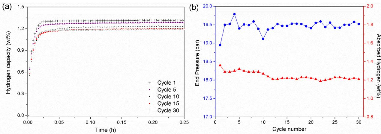
Fig. S8. (a) Absorption kinetics and (b) maximum hydrogen capacity of  $\text{Na}_2\text{Mg}_2\text{NiH}_6$  for 30 cycles measured inside a Sieverts apparatus.  $T_{des} = 400\text{ }^\circ\text{C}$  and  $0.7\text{ bar H}_2$ ;  $T_{abs} = 400\text{ }^\circ\text{C}$  and  $40\text{ bar H}_2$ . The blue circles (b) indicate the end pressure after the absorption step. The red triangles indicate the wt %  $\text{H}_2$  absorbed in each cycle.
