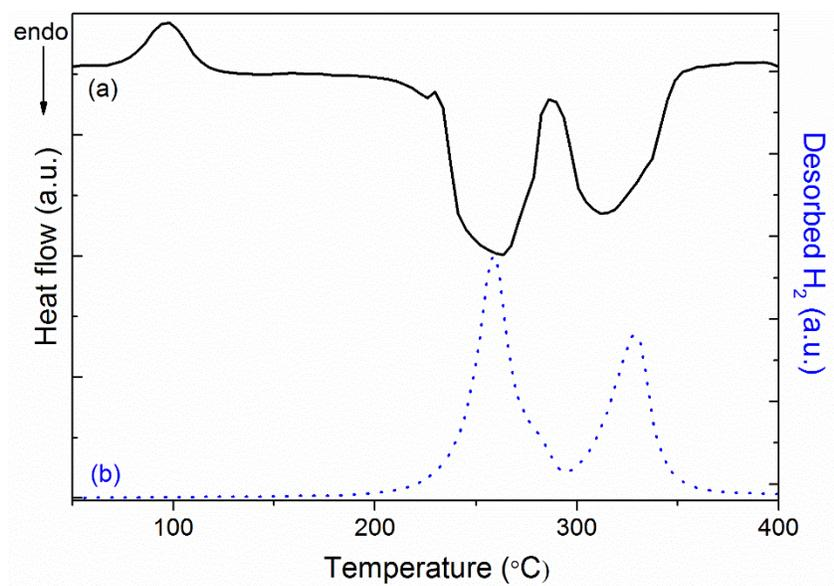
**Fig. S2.** DSC (a) and TPD-MS (b) analysis of  $\text{Na}_2\text{Mg}_2\text{NiH}_6$ .  $\Delta T/\Delta t = 2\text{ }^\circ\text{C}/\text{min}$ .
