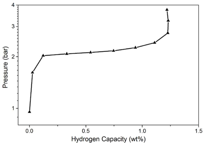
**Fig. S5.** PCI absorption measurement at 315 °C of previously decomposed Na<sub>2</sub>Mg<sub>2</sub>NiH<sub>6</sub>.
