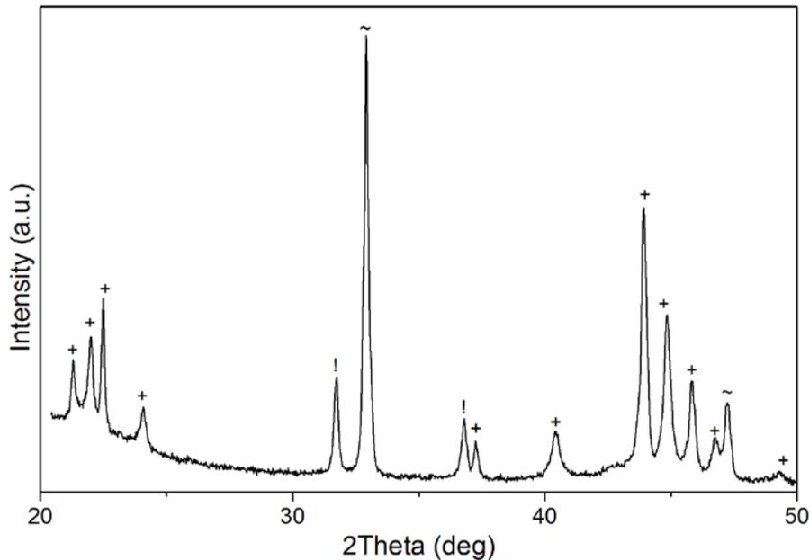
**Fig. S6.** Room temperature XRD pattern of material after a PCI absorption measurement at 315 °C of previously decomposed  $\text{Na}_2\text{Mg}_2\text{NiH}_6$ .  $\sim = \text{NaMgH}_3$ ;  $! = \text{NaH}$ ;  $+ = \text{MgNi}_2$ .  $\lambda = \text{CuK}\alpha$ .
