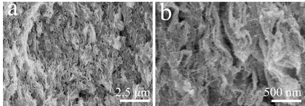
**Fig. S2.** The SEM images of the cross-sectional for DN-PGH/PANI<sub>PA</sub> hydrogel piece tensile samples.
