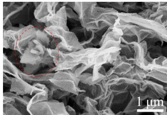
**Fig. S7.** The SEM image of double-crosslink network hydrogel with the aniline concentration of 0.25 M.
