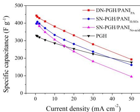
**Fig. S11.** The gravimetric specific capacitance of DN-PGH/PANI<sub>PA</sub>, SN-PGH/PANI<sub>H<sub>2</sub>SO<sub>4</sub></sub>, SN-PGH/PANI<sub>No-acid</sub> and PGH hydrogels.
