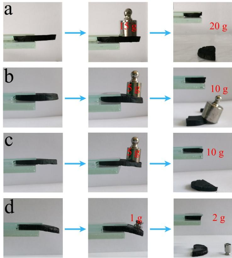
**Fig. S4.** The photographs of (a) DN-PGH/PANI<sub>PA</sub>, (b) SN-PGH/PANI<sub>H<sub>2</sub>SO<sub>4</sub></sub>, (c) SN-PGH/PANI<sub>No-</sub>acid and (d) PGH with a weight loading showing the stiffness. The distance between the center of weight and the center of hydrogel is calculated as ~8 mm.
