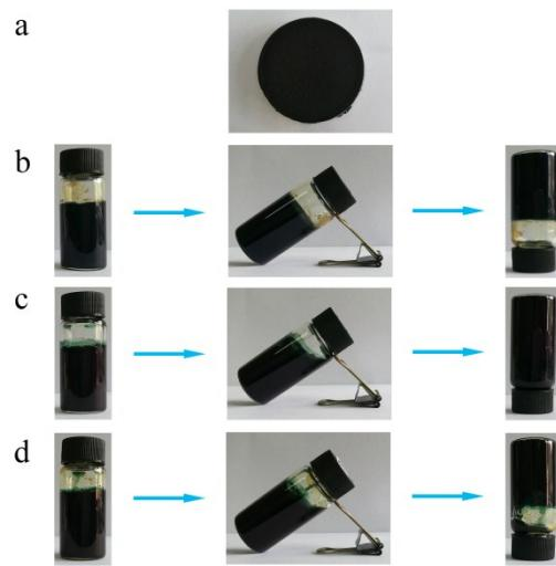
**Fig. S1.** The photographs of (a) functionalized graphene hydrogel (PGH) and (b-d) PANI synthesized at different conditions ((b). in PA aqueous solution, (c). in 1 M  $\text{H}_2\text{SO}_4$  aqueous solution, (d). in the deionized water).
