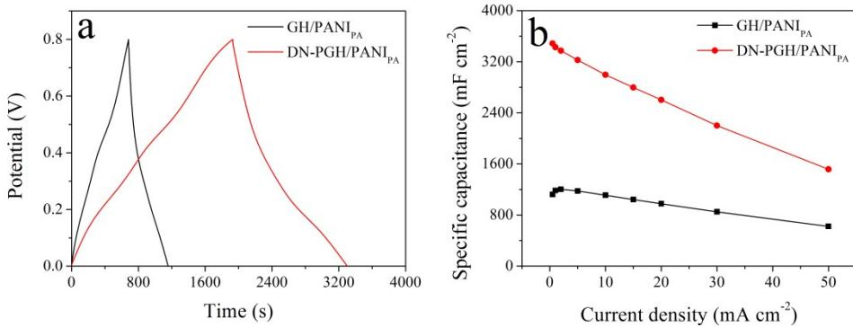
**Fig. S9.** (a) The galvanostatic charge/discharge curves at a current density of  $1 \text{ mA cm}^{-2}$ ; (b) the areal specific capacitance versus different current densities ( $0.5\text{--}50 \text{ mA cm}^{-2}$ ) for GH/PANI<sub>PA</sub> and DN-PGH/PANI<sub>PA</sub> hydrogel.
