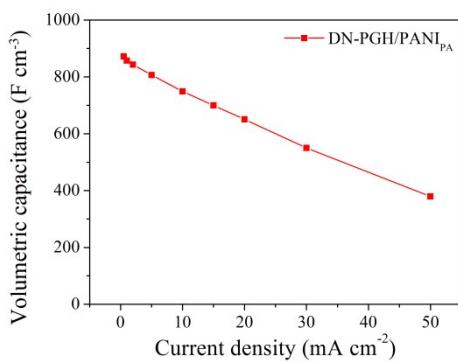
**Fig. S10.** The volumetric specific capacitance versus different current densities of DN-PGH/PANI<sub>PA</sub> hydrogel.
