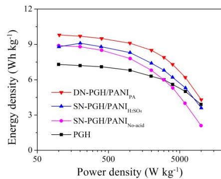
**Fig. S13.** Ragone plots of gravimetric energy density and power density of DN-PGH/PANI<sub>PA</sub>, SN-PGH/PANI<sub>H<sub>2</sub>SO<sub>4</sub></sub>, SN-PGH/PANI<sub>No-acid</sub> and PGH supercapacitor.
