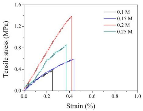
**Fig. S6.** The tensile stress-strain curves of double-crosslink network hydrogels with different aniline concentration (0.1 M, 0.15 M, 0.2 M (DN-PGH/PANI<sub>PA</sub>), and 0.25 M).
