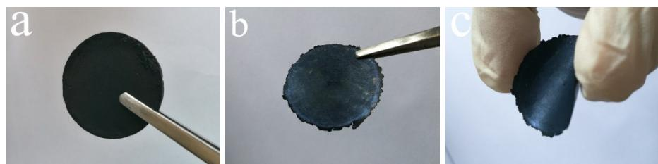
**Fig. S3.** The photographs of DN-PGH/PANI<sub>PA</sub> hydrogels in various states. (a) Without pressuring, (b) Under pressure in its initial state, and (c) Under pressure in its bending state.
