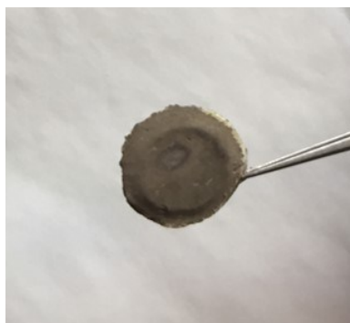
Fig. S4 Digital picture of the cycled lithium metal anode retrieved from the cell employing the SnS 2 -ND@G cathode.
