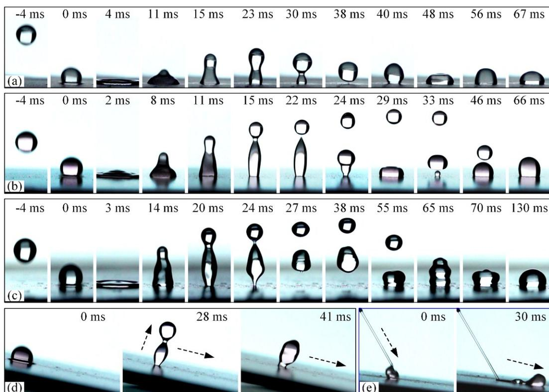
Fig. S1 (a-c) Time-lapse images of droplet impact dynamics on the SLIPS at a temperature of 0 °C, 27 °C and 100 °C (droplet volume,  $\sim 5 \mu\text{L}$ ). (d) Droplet impact dynamics on the inclined SLIPS. (e) The inclined SLIPS was impacted by a water jet.
