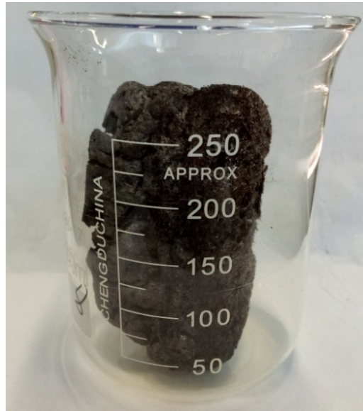
Fig. S2 The optical photo of the foam-like architecture from PMP precursor after thermal annealing at 500 °C for 2 hours.
