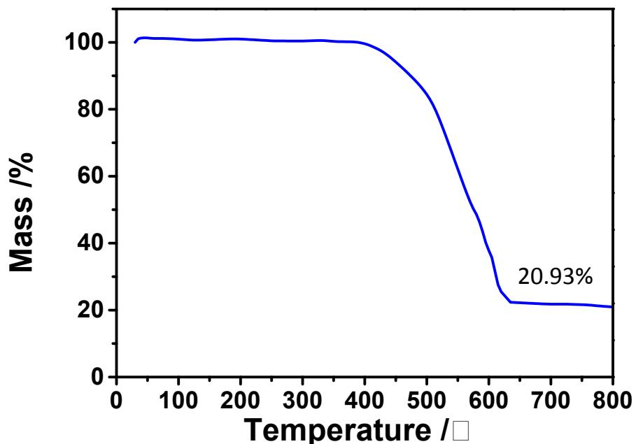
**Fig. S5.** TG curve of the CoTe<sub>2</sub>/G composite obtained in air atmosphere from room temperature to 800  $^\circ\text{C}$  at a rate of 10  $^\circ\text{C}/\text{min}$ .
