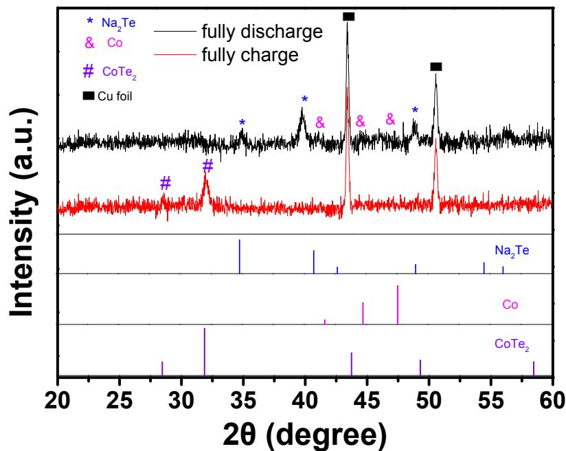
**Fig. S7.** Ex situ XRD patterns of the CoTe<sub>2</sub>/G composite electrode materials at the state of fully discharged to 0.01 V and charged to 2.8 V during the first cycle process, respectively.
