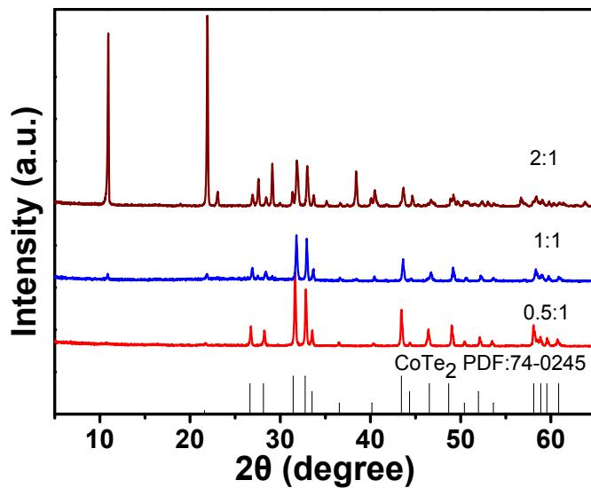
**Fig. S2.** XRD patterns of the CoTe<sub>2</sub> obtained at the molar ratio of Co(AC)<sub>2</sub> and Na<sub>2</sub>TeO<sub>3</sub> is 0.5:1, 1:1, 2:1.
