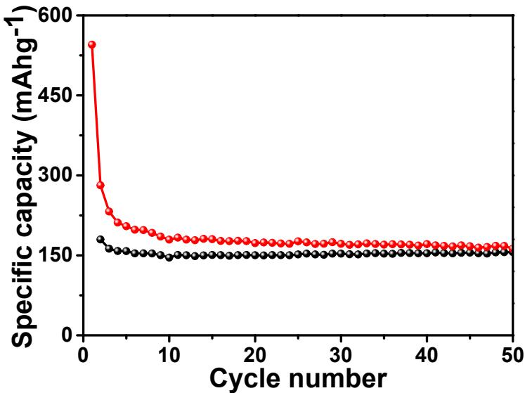
**Fig. S8.** Cycle properties of graphene nanosheets obtained by removal of CoTe<sub>2</sub> in the CoTe<sub>2</sub>/G composite of SIBs at 0.05 A g<sup>-1</sup>.
