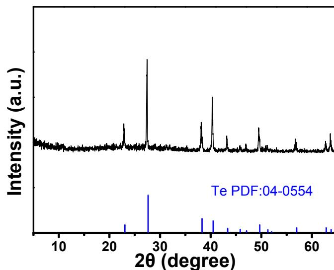
**Fig. S1.** XRD pattern of the intermediates obtained at the molar ratio of  $\text{Co}(\text{AC})_2$  and  $\text{Na}_2\text{TeO}_3$  is 0.5:1 at 180 °C for 3h.
