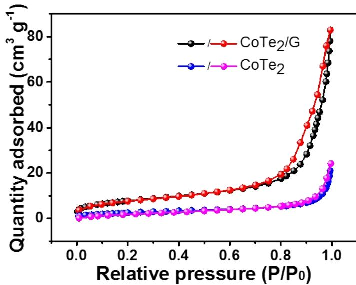
**Fig. S4.**  $N_2$  adsorption-desorption isotherms of and CoTe<sub>2</sub> and CoTe<sub>2</sub>/G composite.
