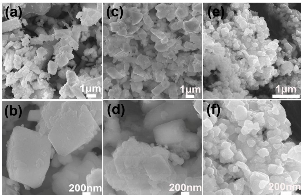
**Fig. S3.** SEM images of the CoTe<sub>2</sub> obtained at the molar ratio of Co(AC)<sub>2</sub> and Na<sub>2</sub>TeO<sub>3</sub> a,b) 2:1; c,d) 1:1; e,f) 0.5:1.
