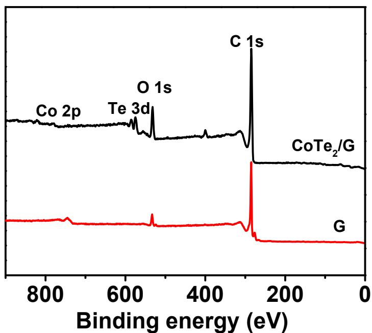
**Fig. S6.** XPS survey spectra of the CoTe<sub>2</sub>/G composite and graphene.
