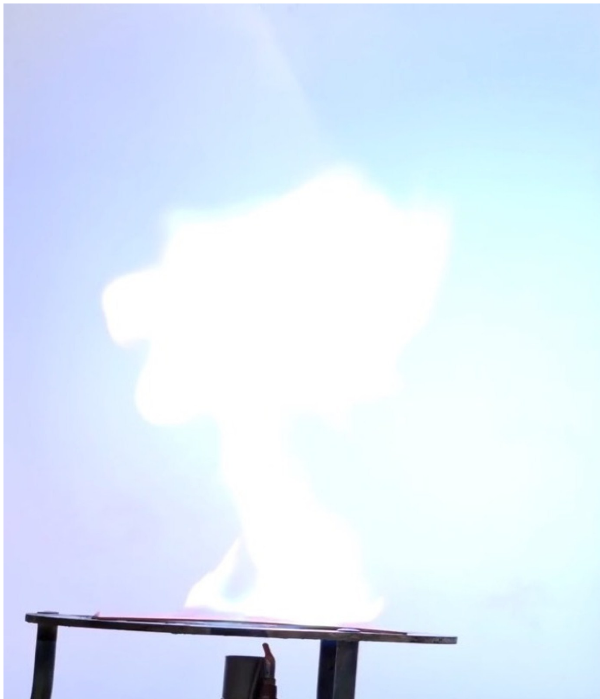
Figure S16 Moment of deflagration of complex 11 during the hot plate test.
