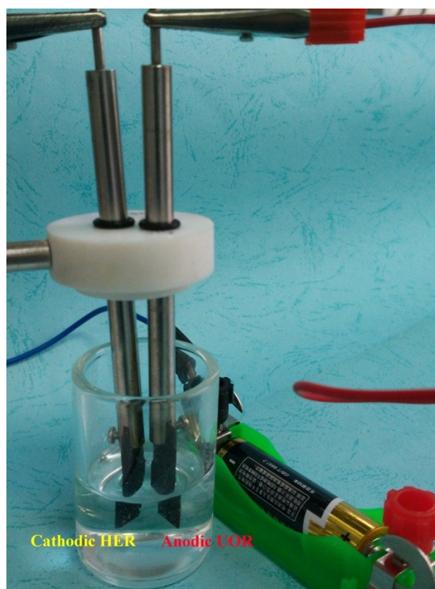
Figure S14. Digital images to show the Mo-Ni 2 P/NF (+) || Co-Fe 2 P/NF (–) urea electrolyzer powered by a single cell AAA battery with a nominal voltage of 1.5 V for UOR.
