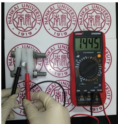
Fig. S15 Open circuit potential of a liquid Zn-air battery with MnO@Co-N/C catalysts.
