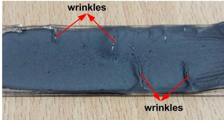
**Figure S4.** The picture of the graphene composite prepared without pre-stretch process.
