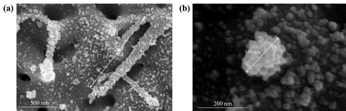
**Fig. S-2** (a) SEM image of submicro-nano rods. (b) SEM image of nanoparticle.
