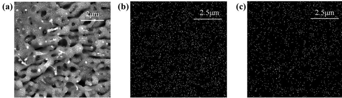
**Fig. S-5** (a) SEM image of microstructure in the micropit after 9 kg water impinging test. (b) EDS element mapping of fluorine before water drop impact test. (c) EDS element mapping of fluorine after 9 kg water impinging test.
