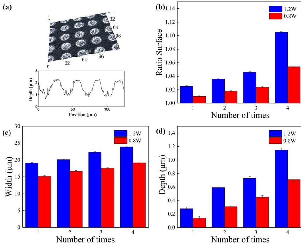
**Fig. S-1** (a) Microstructure of optimal designed glass surface under a laser scanning confocal microscope and its 2D topography. (b) Changes of ratio surface of the ablated glass surface by variation of laser ablation times, the blue parts correspond to the using laser power of 1.2 W and the red parts correspond to laser power of 0.8 W. (c) Changes of diameter of the micropits by variation of laser ablation times. (d) Changes of depth of the micropits by variation of laser ablation times.
