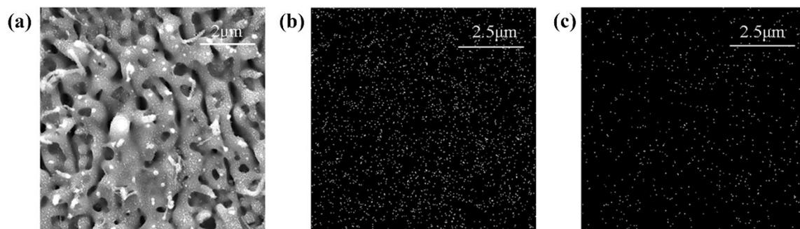
**Fig. S-7** (a) SEM image of microstructure in the micropit after 600°C heating treatment. (b) EDS element mapping of fluorine before thermal treatment. (c) EDS element mapping of fluorine after 600°C heating treatment.
