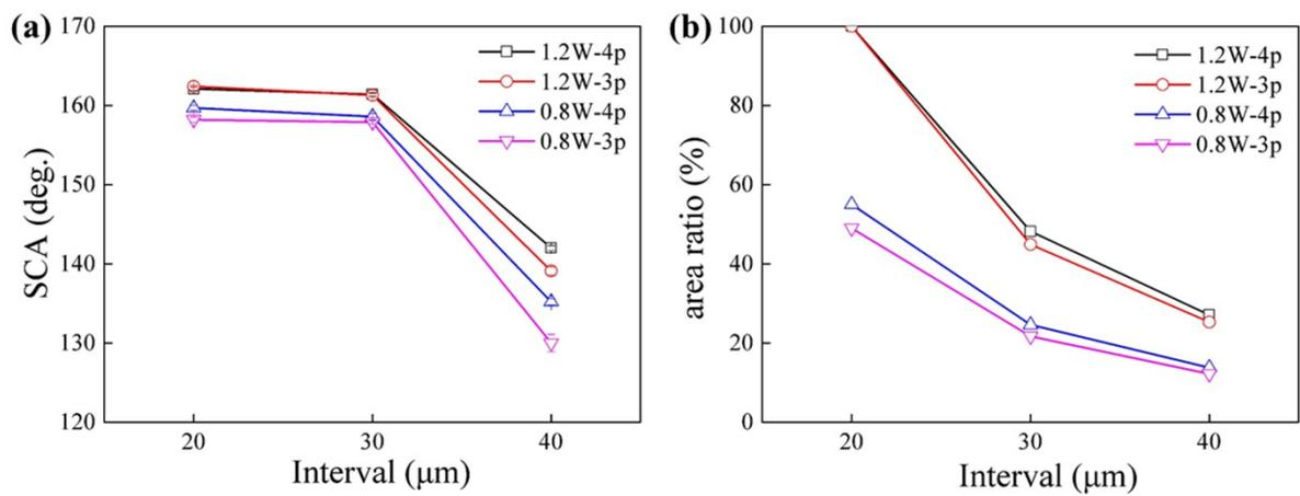
**Fig. S-4** (a) Changes of SCA by variation of interval between micro-pit array. (b) Changes of processed area ratio by variation of interval between micro-pit arrays.
