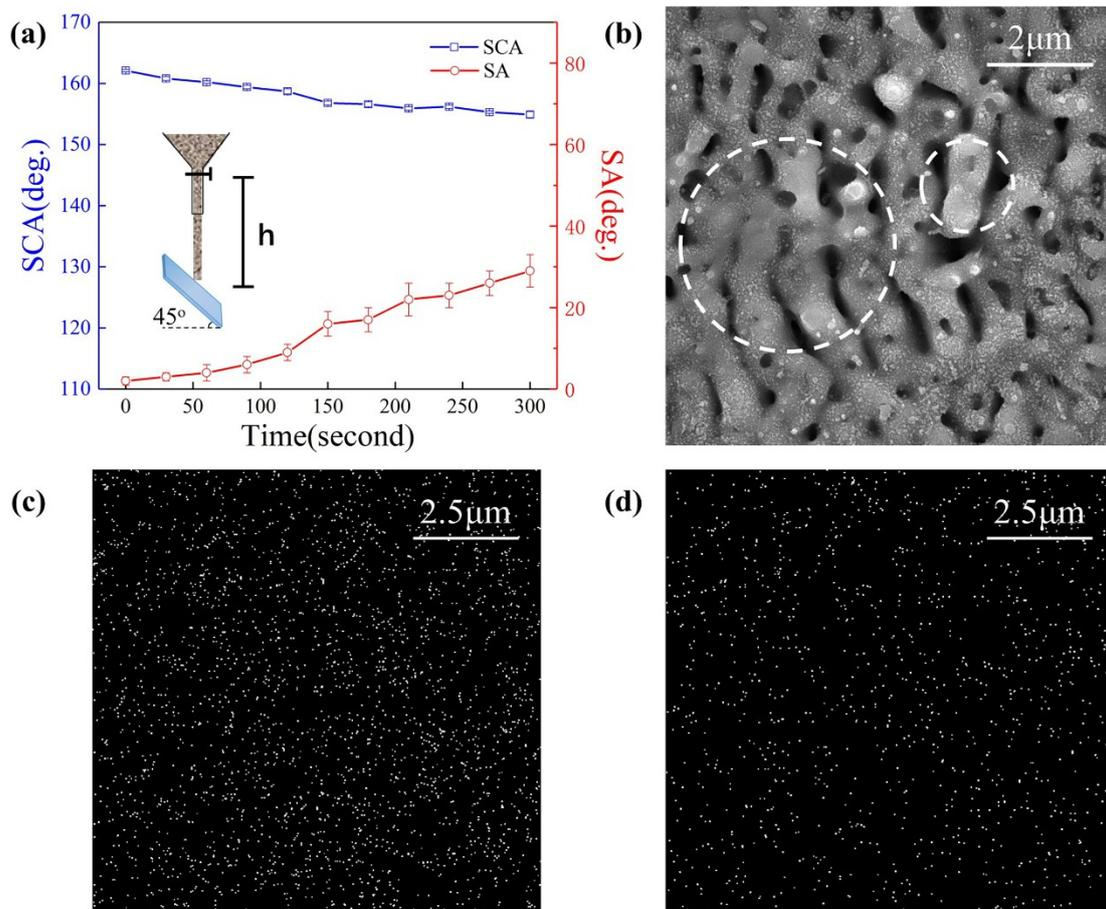
**Fig. S-6** (a) Changes of SCAs&SAs after sand abrasion test in 300 s, inset is the schematic illustration of the sand abrasion test. The sizes of sand varied from 100  $\mu\text{m}$  to 300  $\mu\text{m}$ , the velocity is about 30 g/min and the height is 20 cm. (b) SEM image of microstructure in the micropit after 150 g sand abrasion test. (c) EDS element mapping of fluorine before sand abrasion test. (d) EDS element mapping of fluorine after 150 g sand abrasion test.
