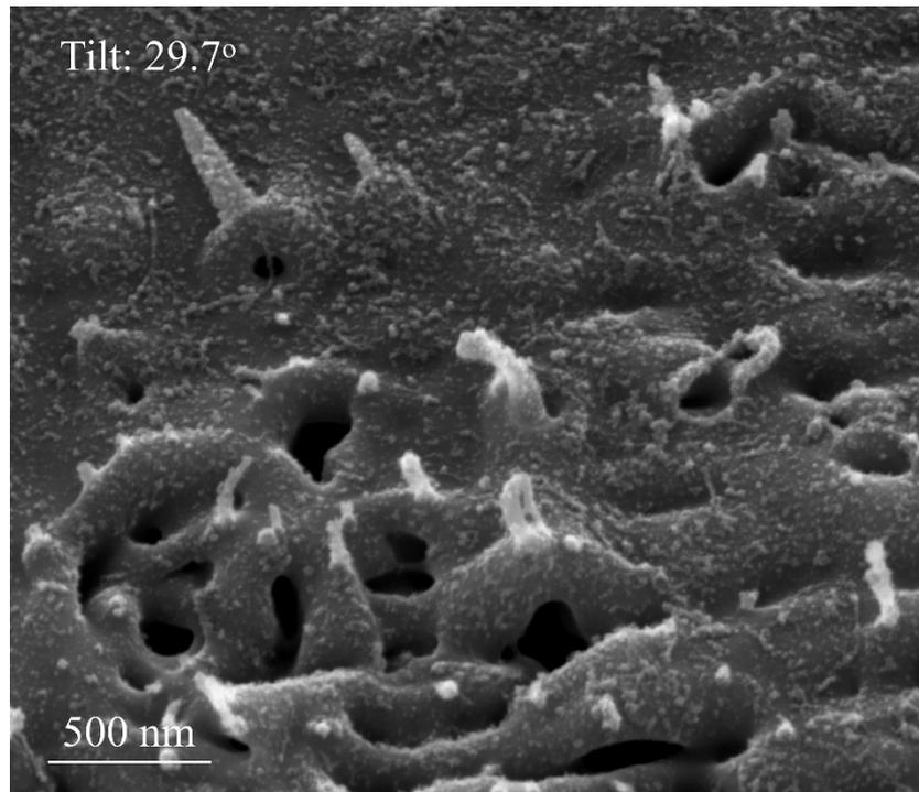
**Fig. S-3** SEM image of the side-view of the texture inside the micropit with type-3 laser treatment.
