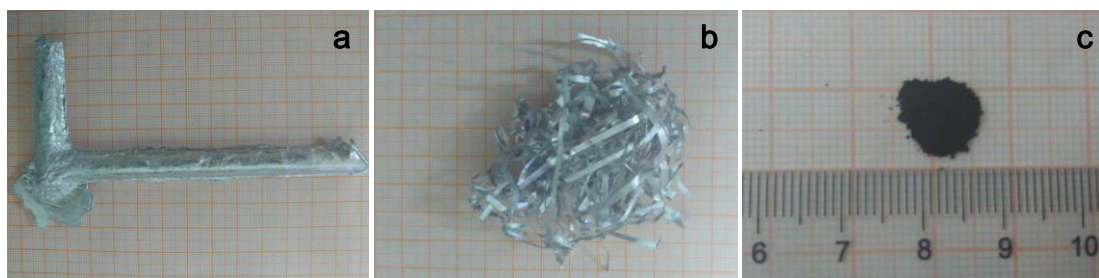
Figure S1. Photographs of (a) \text{Al}_{97.7}\text{Ni}_2\text{Pd}_{0.2}\text{Pt}_{0.1} alloy ingot, (b) \text{Al}_{97.7}\text{Ni}_2\text{Pd}_{0.2}\text{Pt}_{0.1} alloy ribbons, and (c) PdPtNi NPNWs catalyst after dealloying.
