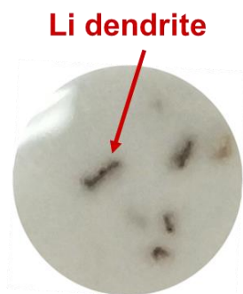
Figure S3. The photo of a bare LLZNO pellet having suffered the formation of lithium dendrite after cycling at a current density of 0.5 \text{mA cm}^{-2} under RT. This serious consequence indicates that the contact and wetting performance between garnet and lithium is one of the principle hurdles hindering the development of SSBs.
