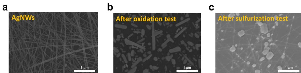
**Fig. S7.** SEM images of the AgNWs electrode (a) before oxidation and sulfurization and (b, c) after oxidation and sulfurization for 60 min, respectively.
