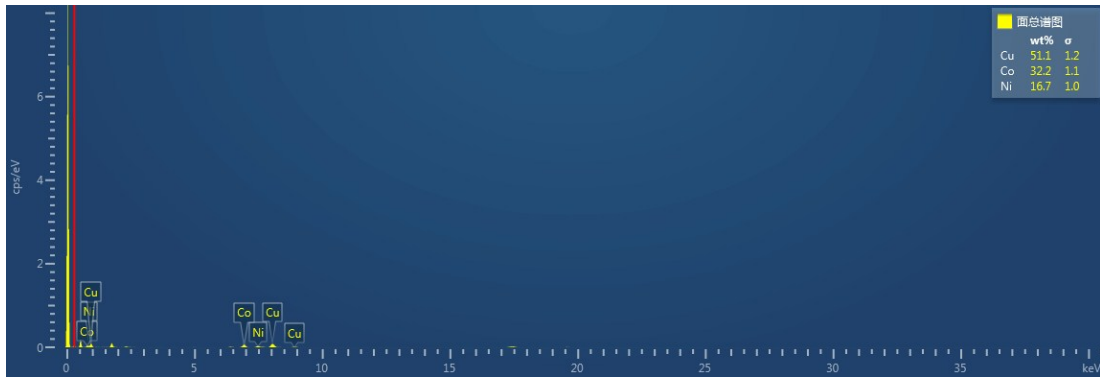
Figure S10 EDS content of \text{Cu}(\text{OH})_2@ \text{CoNiCH} NTs.
