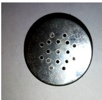
Figure S14. Photo of cathodic shell of coin-type cell used in the Li-CO 2 battery test.
