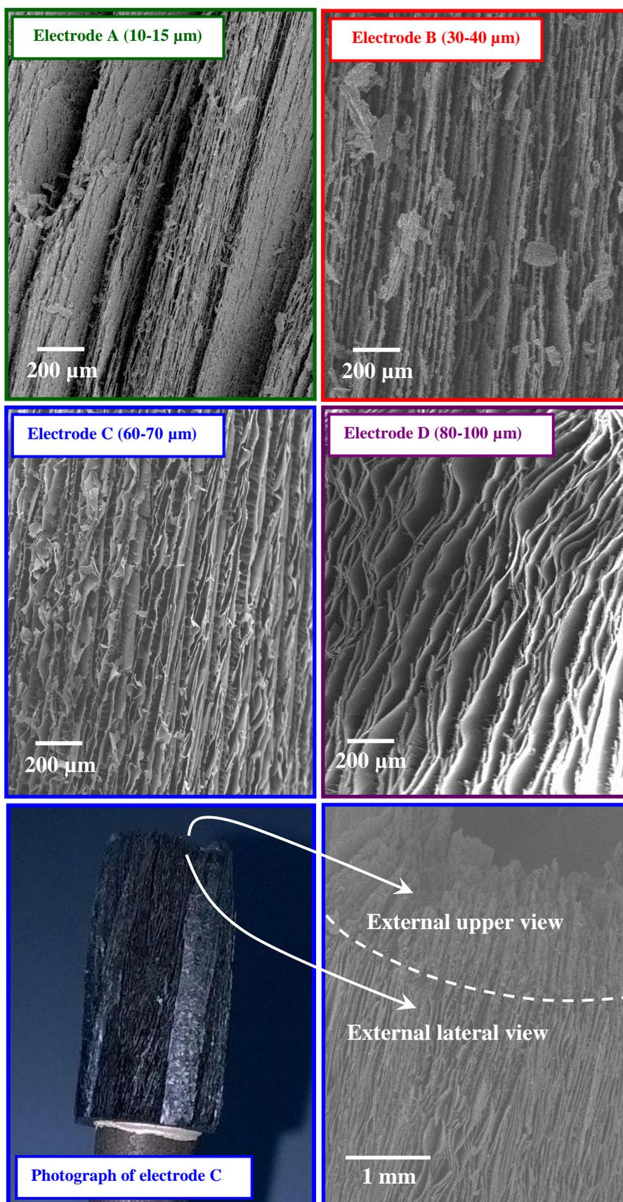
**Fig. S4 - Scanning electron micrographs of ITTC bio-anodes. Bottom left: photograph of the electrode C and a SEM image of its external features. The dashed line indicates (as a guide to the eye) the separation between the**
