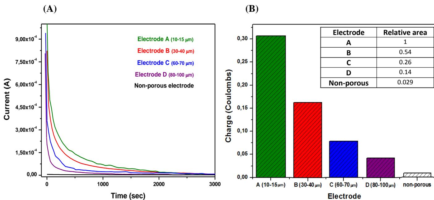
**Fig. S3 - (A)** Current discharged in time corresponding to the tested electrodes. The area under the curves represents the accumulated charge at the electrode surface/solution interface. **(B)** Bar chart depicting the accumulated charge as a function of layer-to-layer distance for each electrode. The total charge is proportional to the anode surface area. The inset table depicts the resulting relative electrode areas.
