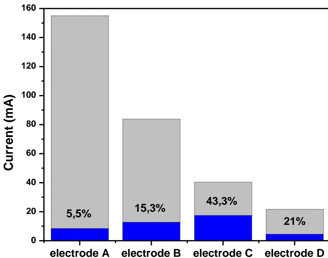
**Fig. S5** - Grey-colored bars represent the current that could be ideally reached if scaling the surface current density of the non-porous anode ( $2 \text{ mA}\cdot\text{cm}^{-2}$ ) to each porous electrode according to their relative areas. Blue-colored bars account for the obtained electrical currents.
