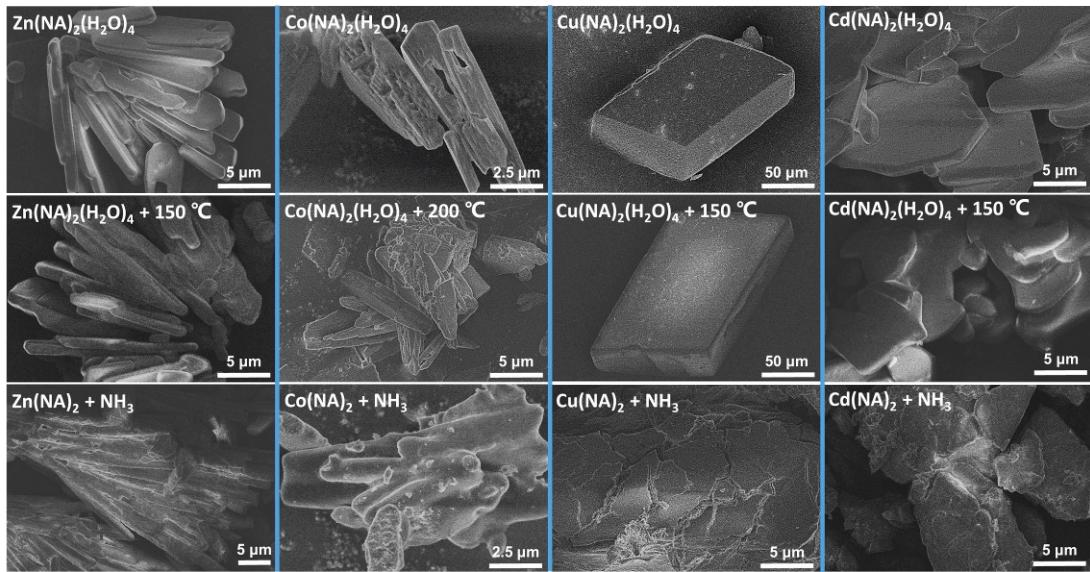
**Fig. S4** The SEM images of the as-synthesized  $M(NA)_2(H_2O)_4$  ( $M = Zn, Co, Cu, Cd$ ) samples, and their SEM images after activated or adsorbing  $NH_3$ .
