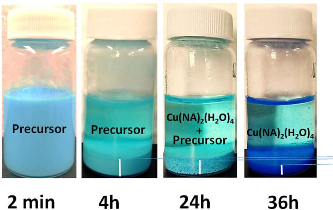
**Fig. S1** Evolution of the precursor transformed to crystals in the synthesis of  $\text{Cu}(\text{NA})_2(\text{H}_2\text{O})_4$ .
