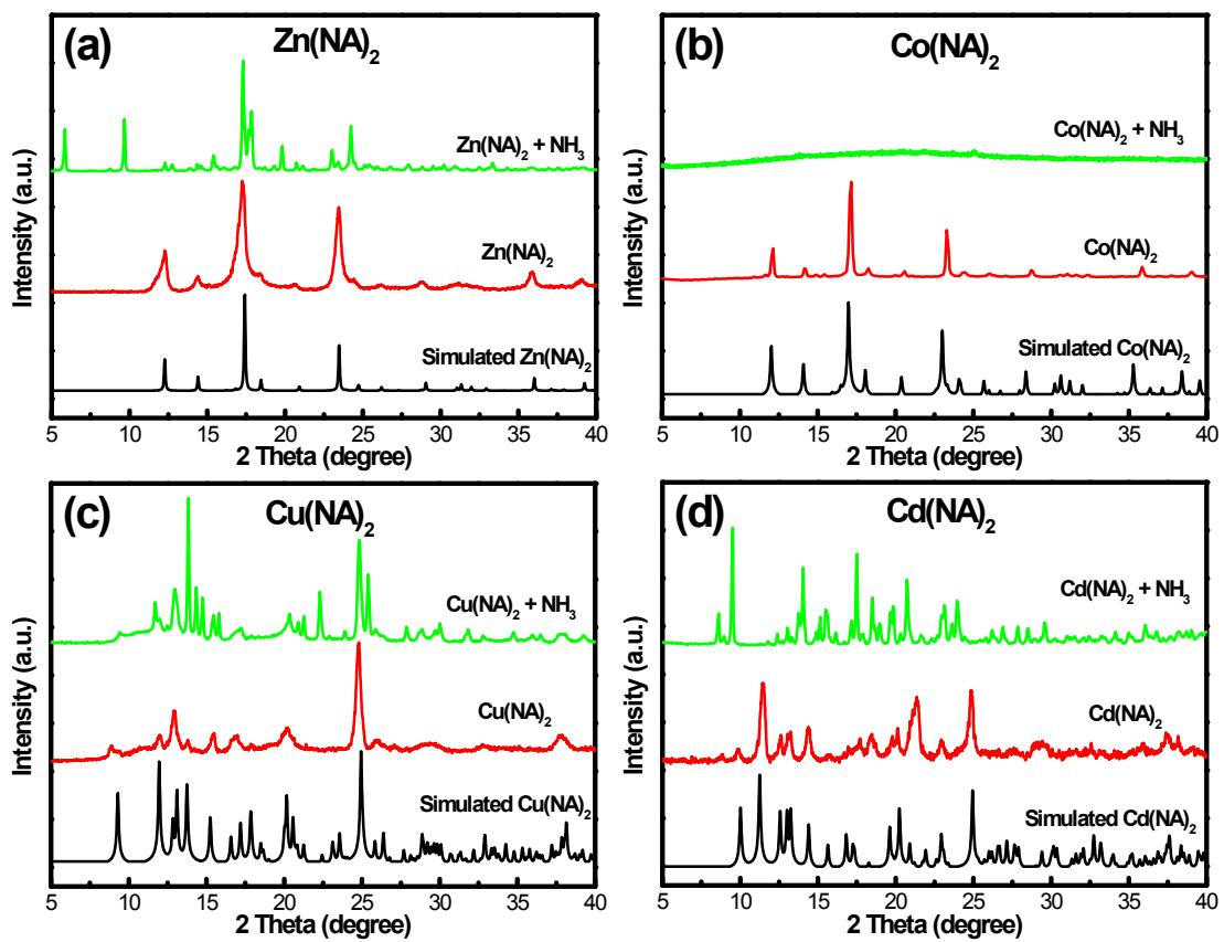
**Fig. S7** Compared PXRD patterns for  $M(NA)_2$  ( $M = Zn, Co, Cu, Cd$ ) and they were adsorbed  $NH_3$ .
