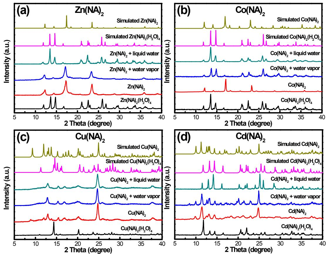
**Fig. S2** The compared PXRD patterns of  $M(NA)_2$  ( $M = Zn, Co, Cu, Cd$ ) adsorbed  $H_2O$  in liquid or steam condition.
