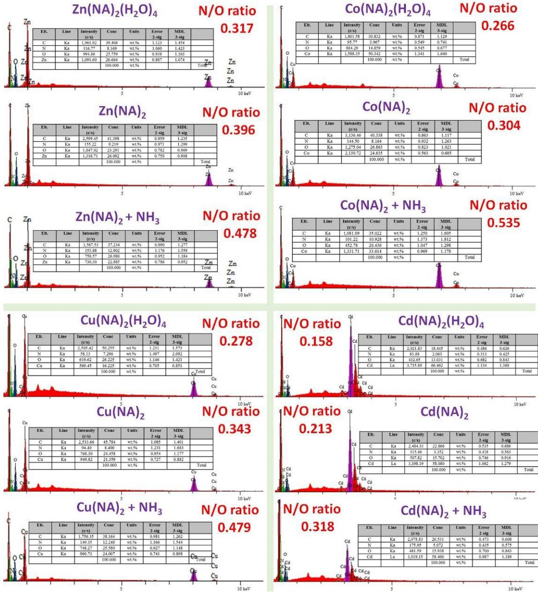
**Fig. S5** EDS spectra of M(NA)<sub>2</sub>(H<sub>2</sub>O)<sub>4</sub> (M = Zn, Co, Cu, Cd) that as-synthesized, activated and adsorbed NH<sub>3</sub>.
