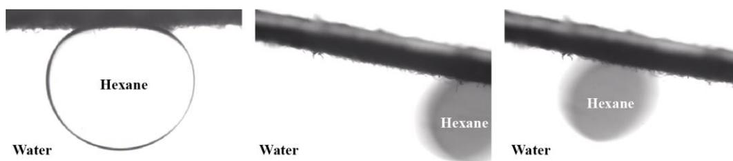
**Figure S9.** A hexane droplet in water on the surface of the prepared fabric modified with 0.2 mM 1H,1H,2H,2H-perfluorodecanethiol. The hexane droplet easily rolls along the inclined surface of the modified fabric.
