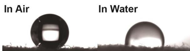
**Figure S7.**  $\theta^*_w$  and  $\theta^*_{ow}$  of CuO-coated fabric modified with 0.2 mM n-octadecylthiol.
