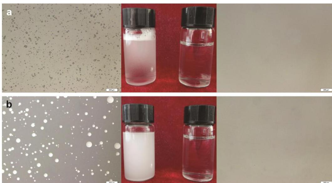
**Figure S54.** Photographs of hexane-in-water (a) and toluene-in-water (b) emulsions before (left) and after (right) separation using the dual superlyophobic SSM.
