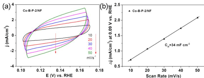
**Fig. S16** (a) CV curves recorded at different scan rates between 0.10 and 0.17 V for Co-B-P-2/NF. (b) Capacitive currents on the basis of scan rate for Co-B-P-2/NF. Calculation of ECSA is given below:
