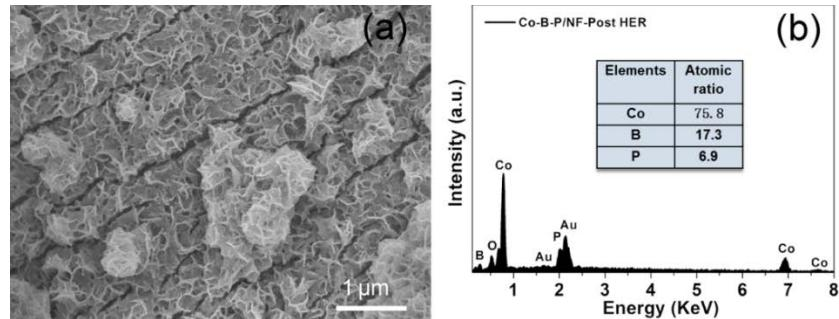
**Fig. S20** (a) The SEM image and (b) EDS spectrum and elemental composition (inset) of Co-B-P/NF after the HER measurement at an overpotential of 88 mV for 20 h. The loading of Co-B-P on the Ni foam substrate before ( $5.12 \text{ mg cm}^{-2}$ ) and after ( $4.96 \text{ mg cm}^{-2}$ ) HER durability test was nearly maintained, indicating the good mechanical stability of the in-situ grown Co-B-P catalysts even at large working current density.
