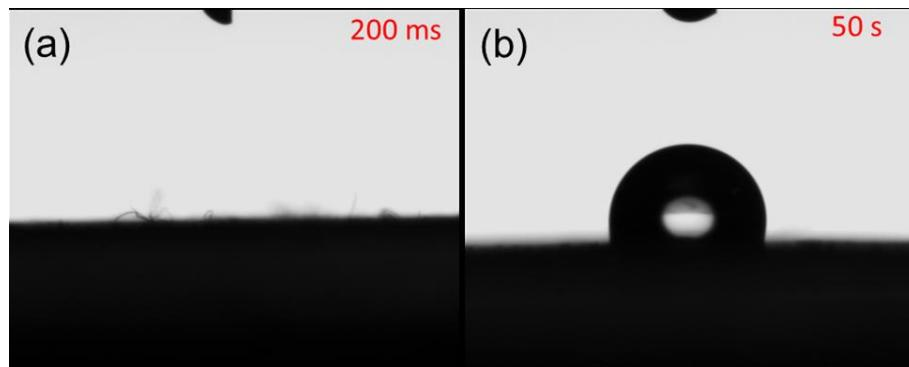
**Fig. S3** The wettability test of Co-B-P nanosheet arrays (a) and Co-B-P nanospheres (b) deposited on Ni foil, respectively.
