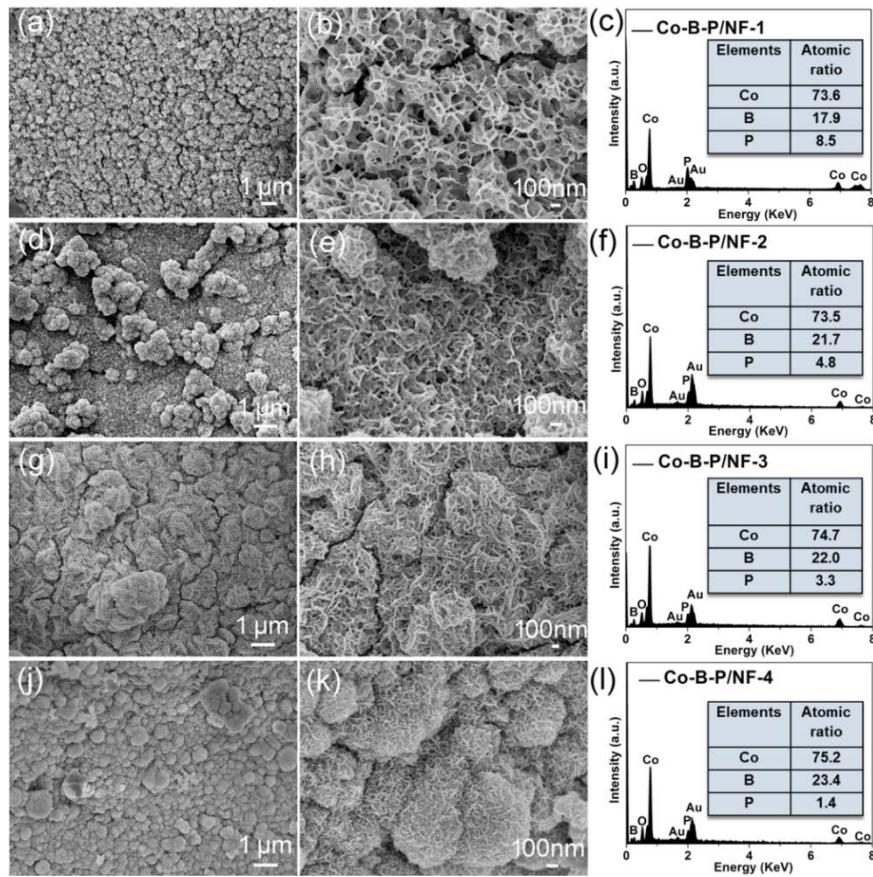
**Fig. S6** SEM images, SEM-EDS spectroscopies and elemental composition analysis of (a-c) Co-B-P/NF-1, (d-f) Co-B-P/NF-2, (g-i) Co-B-P/NF-3, (j-l) Co-B-P/NF-4. The elemental compositions of Co-B-P/NF-1, Co-B-P/NF-2, Co-B-P/NF-3 and Co-B-P/NF-4 from EDS analysis were  $\text{Co}_{2.80}\text{B}_{0.68}\text{P}_{0.32}$ ,  $\text{Co}_{2.77}\text{B}_{0.82}\text{P}_{0.18}$ ,  $\text{Co}_{2.95}\text{B}_{0.87}\text{P}_{0.13}$  and  $\text{Co}_{3.03}\text{B}_{0.94}\text{P}_{0.06}$ , respectively.
