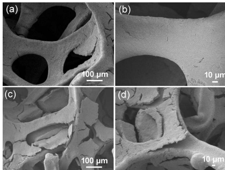
**Fig. S22** The SEM images of Pt/C (20 wt%) loaded on Ni foam before (a,b) and after (c,d) the HER measurement.
