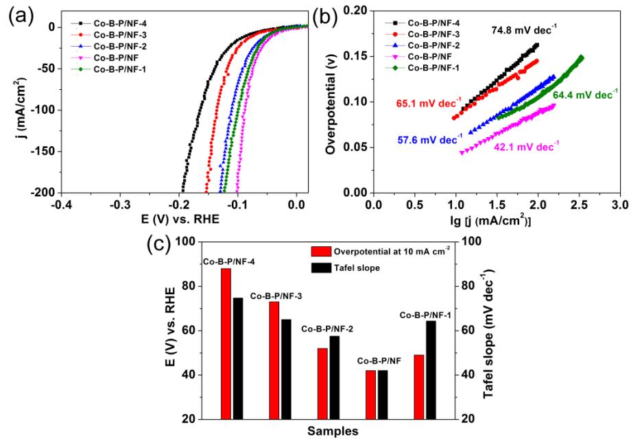
**Fig.S9** (a) Polarization curves of Co-B-P/NF-1, Co-B-P/NF, Co-B-P/NF-2, Co-B-P/NF-3 and Co-B-P/NF-4 in 1 M KOH electrolyte. (b) Tafel plots derived from (a). (c) Comparison of the overpotentials at  $10 \text{ mA cm}^{-2}$  and Tafel slopes of the Co-B-P/NF-1, Co-B-P/NF, Co-B-P/NF-2, Co-B-P/NF-3 and Co-B-P/NF-4.
