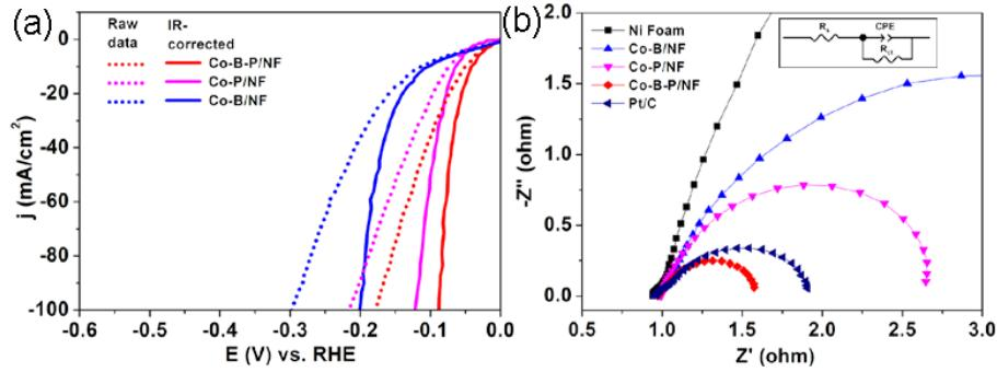
**Fig. S10** (a) Original and iR-corrected polarization curves of Co-B-P/NF, Co-P/NF and Co-B/NF. (b) EIS Nyquist plots of Ni Foam, Co-B/NF, Co-P/NF, Co-B-P/NF and Pt/C recorded at overpotential of 100 mV.
