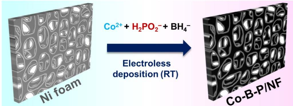
**Fig. S1** Schematic illustration of the synthesis of Co-B-P supported on Ni foam.
