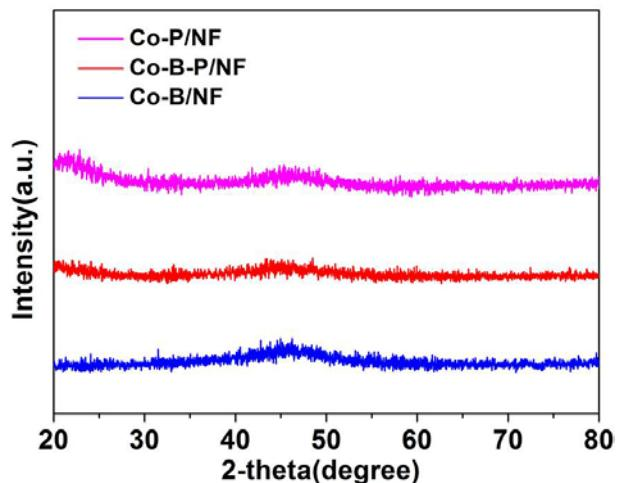
Fig. S5 XRD patterns of Co-P/NF, Co-B-P/NF and Co-B/NF.
