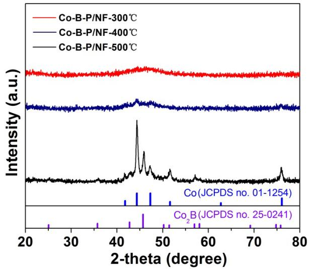
**Fig. S14** The XRD patterns of Co-B-P/NF after thermal treatment at different temperatures for 2 h.
