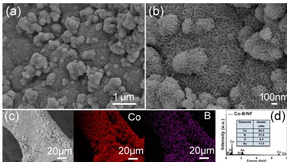
**Fig. S7** (a) Low- and (b) high-magnification SEM images of Co-B/NF. (c) SEM image and EDS elemental mapping of Co and B. (d) The corresponding EDS spectrum and elemental composition analysis (inset).
