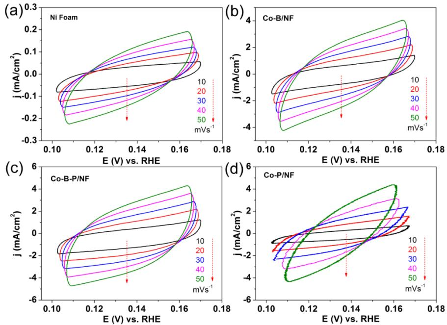
**Fig. S11** CV curves recorded at different scan rates between 0.10 and 0.17 V for (a) Ni foam, (b) Co-B/NF, (c) Co-B-P/NF and (d) Co-P/NF.
