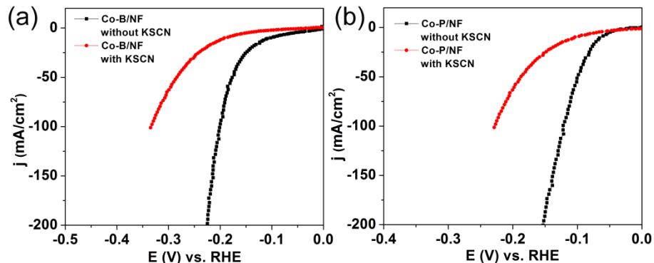
**Fig. S13** (a) Polarization curves of Co-B/NF in 1 M KOH solution with or without 10 mM KSCN. (b) Polarization curves of Co-P/NF in 1 M KOH solution with or without 10 mM KSCN.
