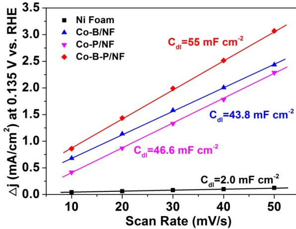
**Fig. S12** Capacitive currents on the basis of scan rate for Ni foam, Co-B/NF, Co-P/NF and Co-B-P/NF at 0.135 V.
