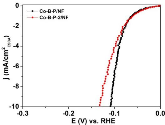
**Fig. S17** ECSA-normalized initial polarization curves from Fig. 5a.
