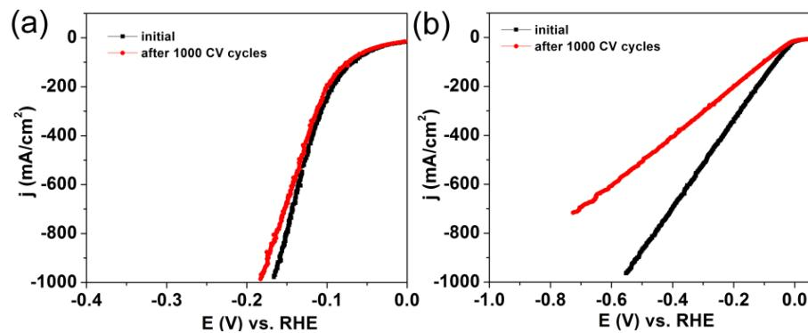
**Fig. S19** Polarization curves of Co-B-P/NF (a) and Pt/C (b) in 1 M KOH before and after 1000 cycles at a scan rate of  $100 \text{ mV s}^{-1}$ .
