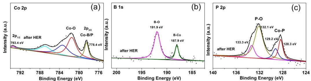
**Fig. S21** High-resolution XPS spectra of (a) Co 2P, (b) B 1s and (c) P 2p after the HER measurement at an overpotential of 88 mV for 20 h.
