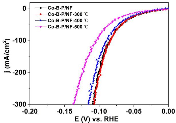
**Fig. S15** The polarization curves of Co-B-P/NF after thermal treatment at different temperatures.
