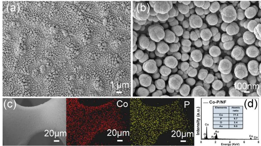
**Fig. S8** (a) Low- and (b) high-magnification SEM images of Co-P/NF. (c) SEM image and elemental mapping of Co and P. (d) The corresponding EDS spectrum and elemental composition analysis (inset).
