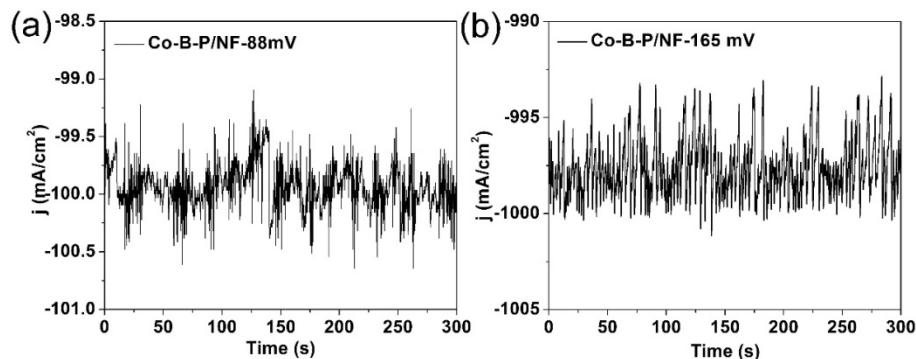
**Fig. S18** Magnified chronoamperometry curves of Co-B-P/NF at overpotentials of 88 mV (a) and 165 mV (b).
