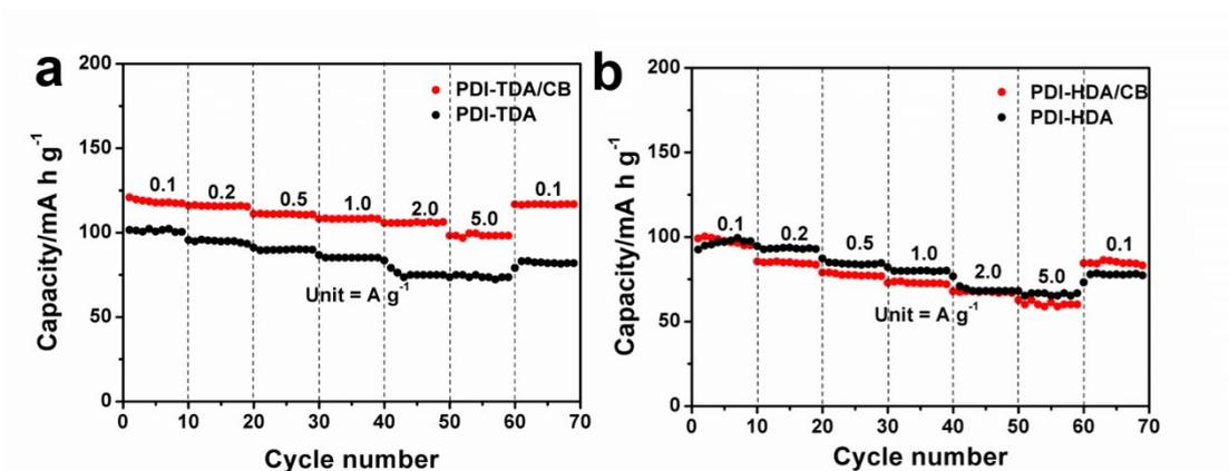
**Figure S9.** a) The rate capabilities of PDI-TDA and PDI-TDA/CB as LIB cathodes with the current densities ranging from 0.1 – 5.0 A g<sup>-1</sup>; b) the rate capabilities of PDI-HDA and PDI-HDA/CB as LIB cathodes with the current densities ranging from 0.1 – 5.0 A g<sup>-1</sup>.
