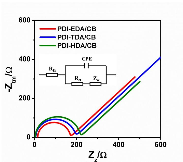
**Figure S6.** The fitted EIS spectra of the PDI-DA/CB composites.
