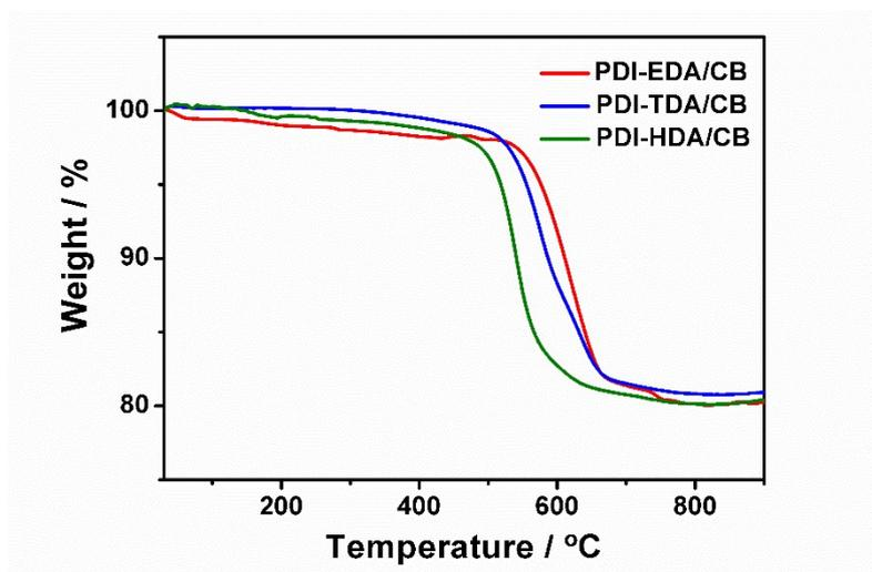
**Figure S5.** TGA curves of the PDI-DA/CB composites obtained at nitrogen atmosphere.
