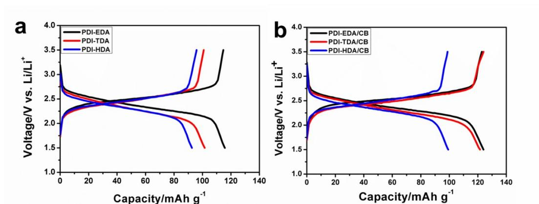
**Figure S8.** a) The galvanostatic discharge-charge profiles of PDI-DAs as the cathode materials in LIBs at 0.1 A g<sup>-1</sup>; b) The galvanostatic discharge-charge profiles of PDI-DA/CBs as the cathode materials in LIBs at 0.1 A g<sup>-1</sup>.
