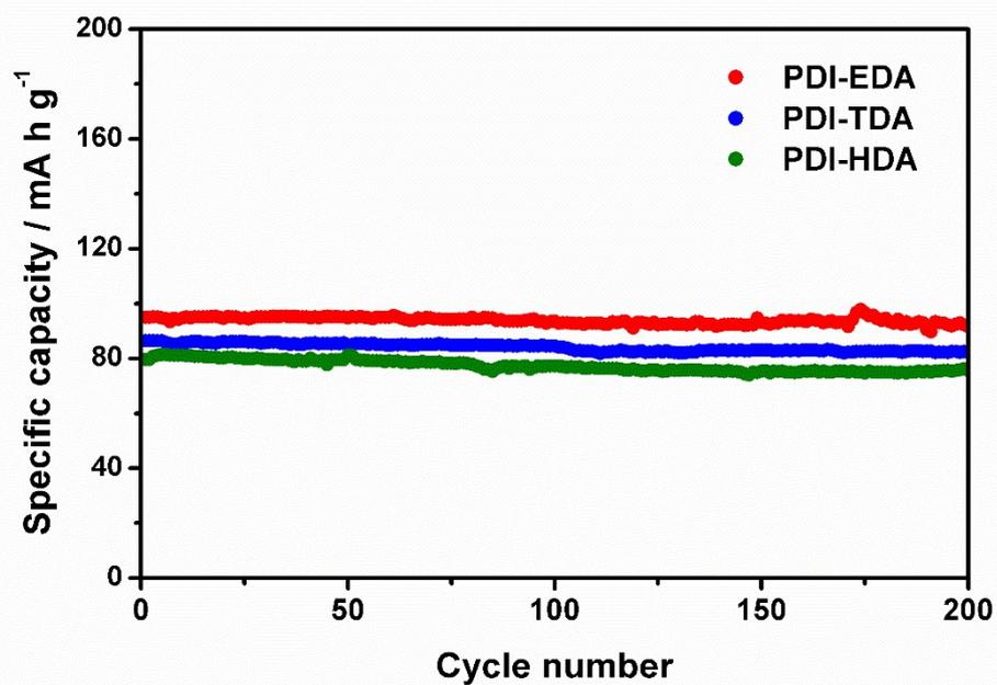
**Figure S13.** The cycling stabilities of PDI-EDA, PDI-TDA and PDI-HDA as SIB cathodes at the current densities of 1.0 A g<sup>-1</sup>. The initial capacities of PDI-EDA, PDI-TDA and PDI-HDA are 95, 86 and 79 mA h g<sup>-1</sup>, which decay to 92, 82 and 76 mA h g<sup>-1</sup>, respectively after 200 charge-discharge cycles.
