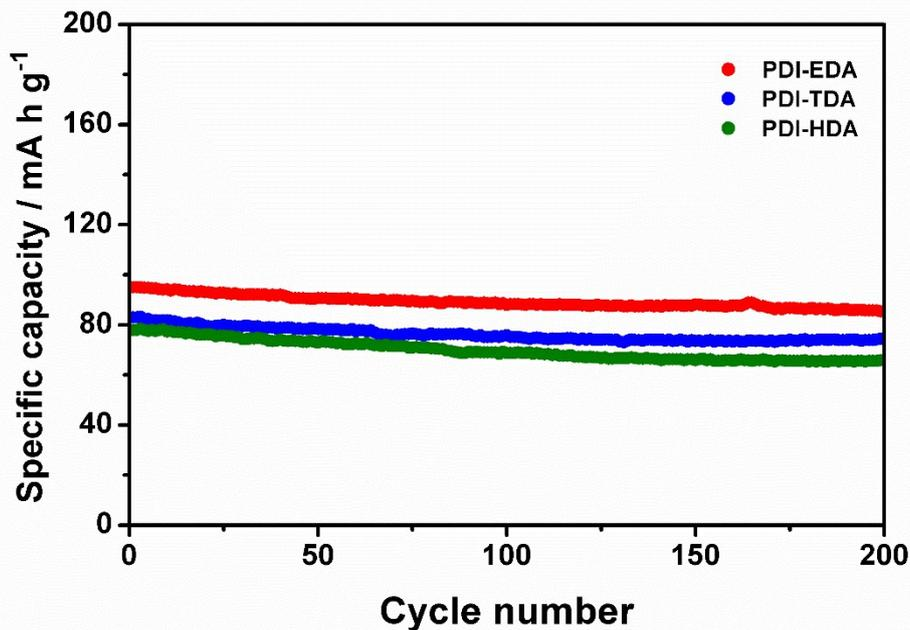
**Figure S10.** The cycling stabilities of PDI-EDA, PDI-TDA and PDI-HDA as LIB cathodes at the current densities of  $1.0 \text{ A g}^{-1}$ .
