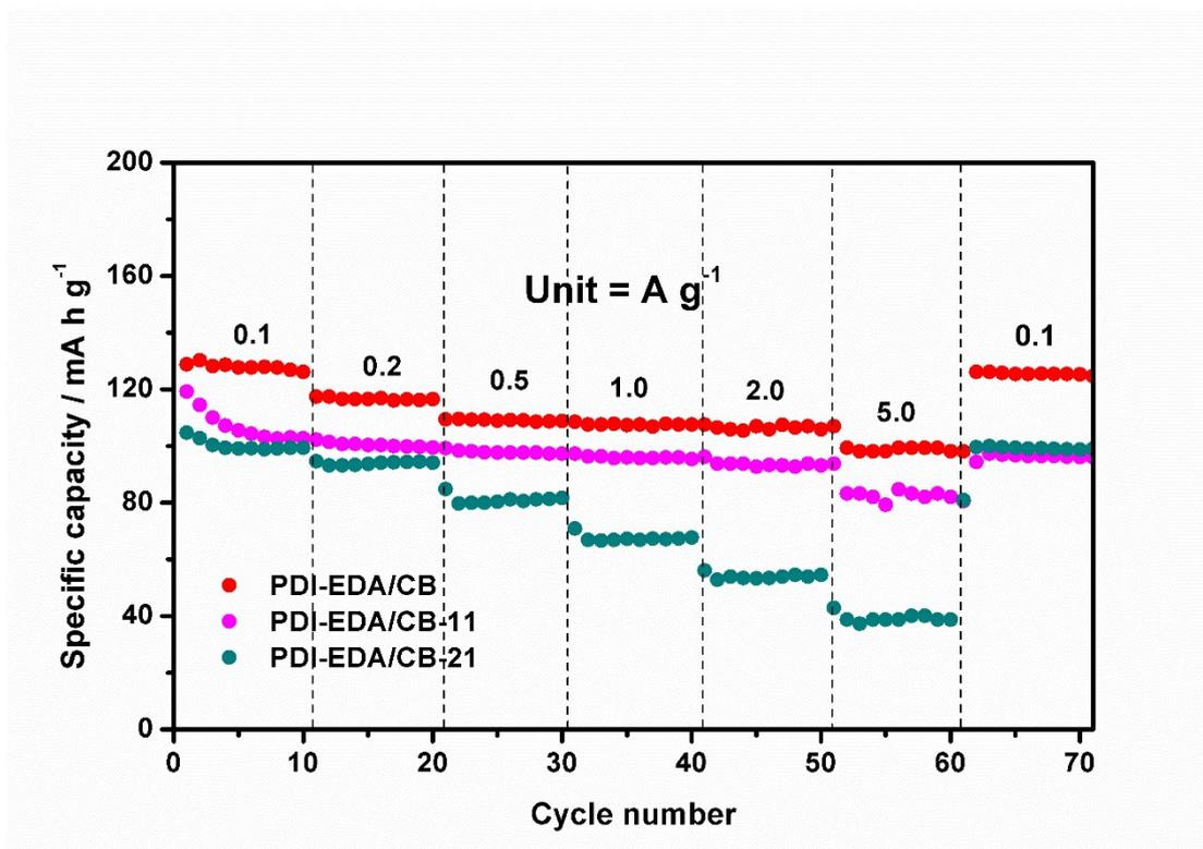
**Figure S1.** The rate capabilities of PDI-EDA/CB, PDI-EDA/CB-11 and PDI-EDA/CB-21 as the cathode in lithium ion battery with the charge-discharge current density varying from 0.1 – 5.0 A g<sup>-1</sup>.
