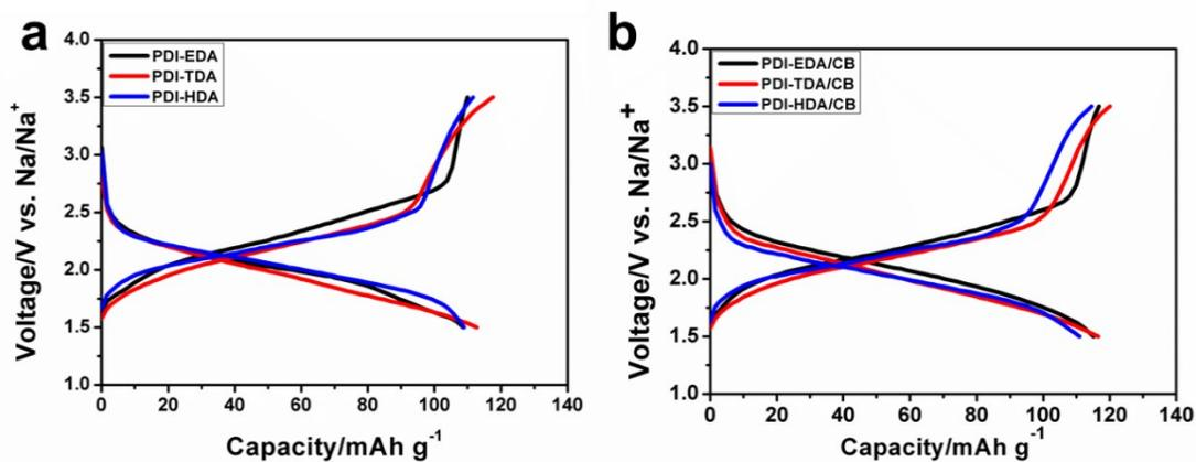
**Figure S11.** a) The galvanostatic discharge-charge profiles of PDI-DAs as the cathode materials in SIBs at  $0.1 \text{ A g}^{-1}$ ; b) The galvanostatic discharge-charge profiles of PDI-DA/CBs as the cathode materials in SIBs at  $0.1 \text{ A g}^{-1}$ .
