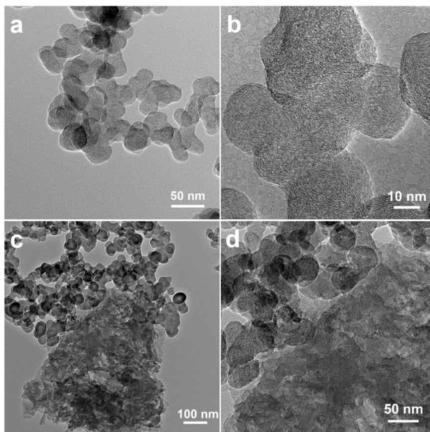
**Figure S4.** TEM images of a) and b) carbon black; c) and d) the mechanically mixed PDI-EDA and carbon black.
