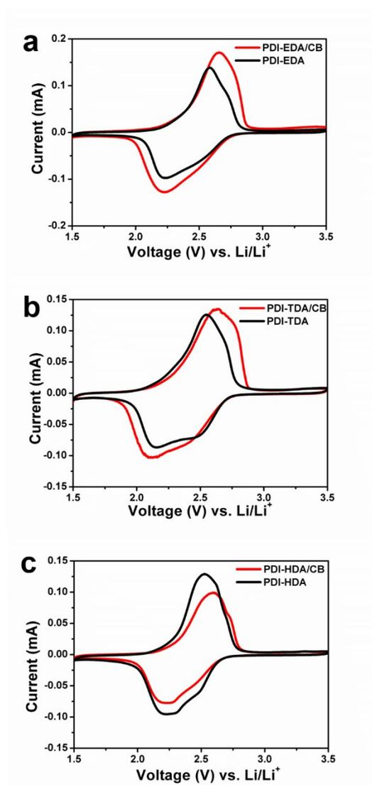
**Figure S7.** a) The CV curves of PDI-EDA and PDI-EDA/CB at  $0.5 \text{ mV s}^{-1}$ ; b) the CV curves of PDI-TDA and PDI-TDA/CB at  $0.5 \text{ mV s}^{-1}$ ; c) the CV curves of PDI-HDA and PDI-HDA/CB at  $0.5 \text{ mV s}^{-1}$ .
