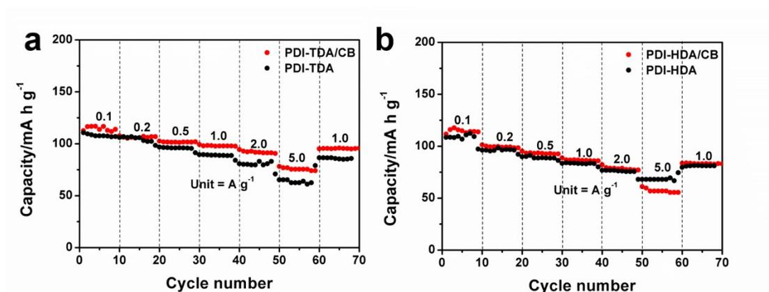
**Figure S12.** a) The rate capabilities of PDI-TDA and PDI-TDA/CB as SIB cathodes with the current density ranging from 0.1 – 5.0 A g<sup>-1</sup>; b) the rate capabilities of PDI-HDA and PDI-HDA/CB as SIB cathodes with the current density ranging from 0.1 – 5.0 A g<sup>-1</sup>.
