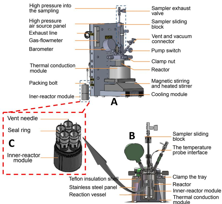
**Scheme S1.** (A) Over-view diagram, (B) section-view diagram, and (C) inner-reactor module diagram of the Wattecs Parallel Autoclave System (WPAS). The WPAS synthetic technique holds the advantages of high temperature and high pressure and allows the constant stirring under a nitrogen and argon gas protecting atmosphere in comparison with normal solvothermal synthetic approach.<sup>1</sup>
