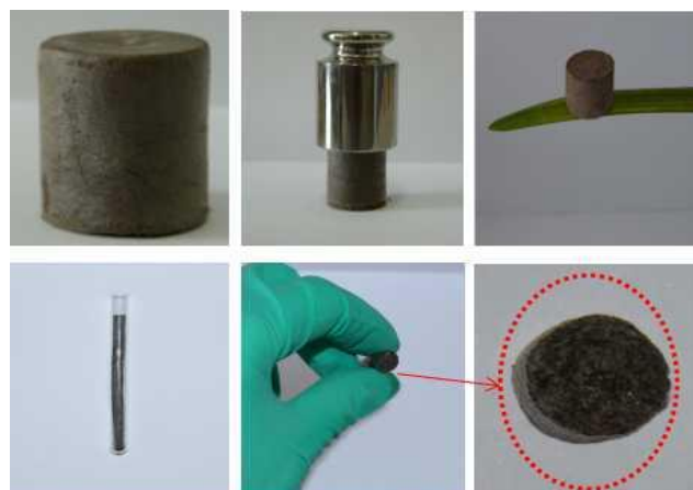
Fig. S31 The photo images of Pd@TpTe-1@chitosan aerogel. Top: cylindrical hybrid aerogel monoliths, Bottom: tubular cylindrical hybrid aerogel casting.
