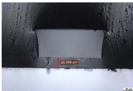
**Figure S4.** Cross section picture of PDMS channel with PDMS membrane.
