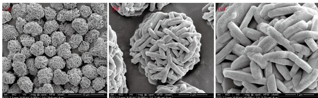
Figure S3 The SEM images of the normal \text{LiNi}_{1/3}\text{Co}_{1/3}\text{Mn}_{1/3}\text{O}_2 calcined at 900\text{ }^\circ\text{C} .
