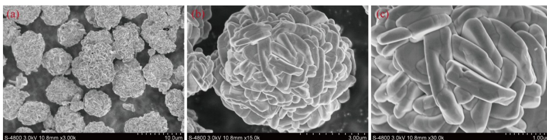
Figure S4 The SEM images of the normal \text{LiNi}_{1/3}\text{Co}_{1/3}\text{Mn}_{1/3}\text{O}_2 calcined at 1000 °C.
