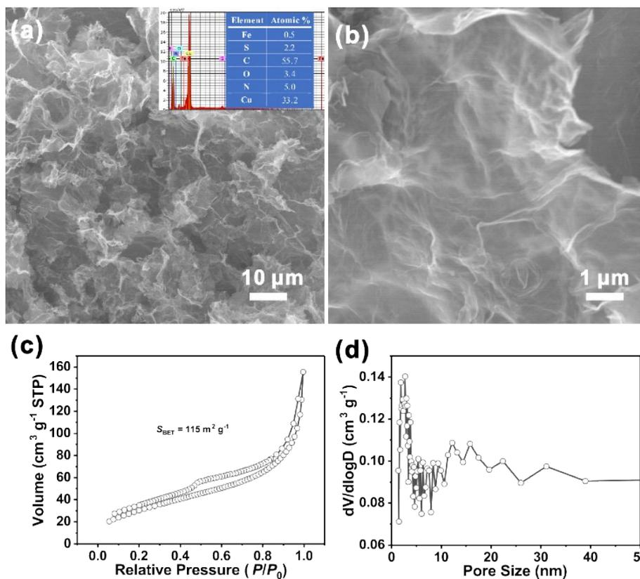
**Figure S3** Characterization of porous carbon that was obtained by removing  $\text{Fe}_{1-x}\text{S}$  component in  $\text{Fe}_{1-x}\text{S}@ \text{NC}@ \text{G}$  composite with aqua regia: (a, b) SEM images; (b) nitrogen sorption isotherm; (c) BJH pore size distribution curve.
