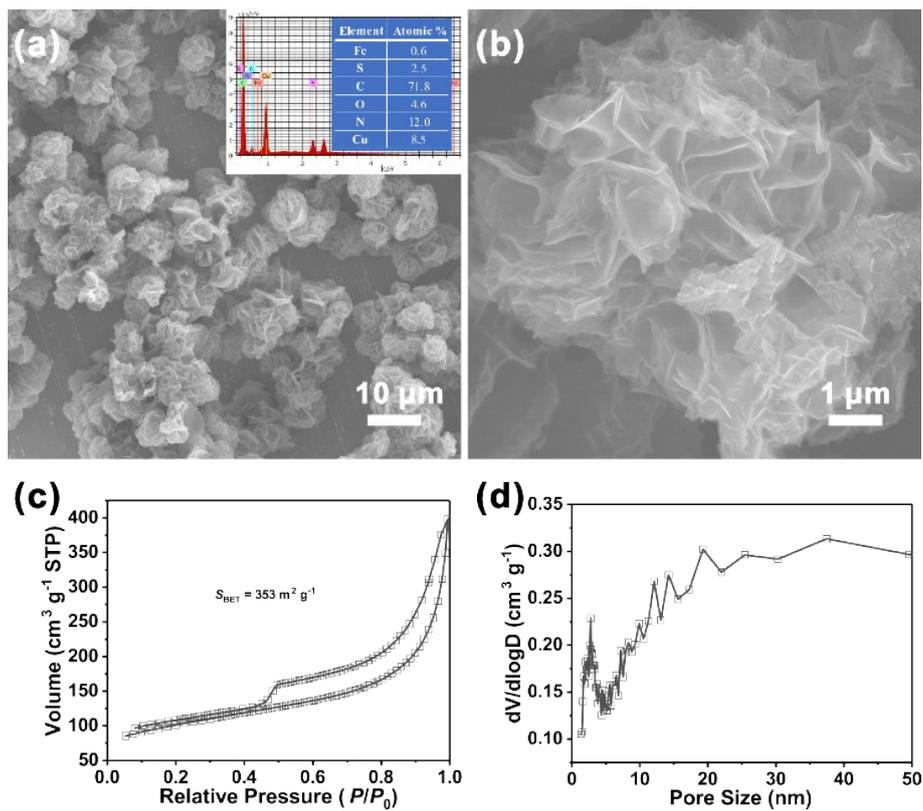
**Figure S2** Characterization of porous carbon that was obtained by removing  $\text{Fe}_{1-x}\text{S}$  component in  $\text{Fe}_{1-x}\text{S}@NC$  composite with aqua regia: (a, b) SEM images; (b) nitrogen sorption isotherm; (c) BJH pore size distribution curve.
