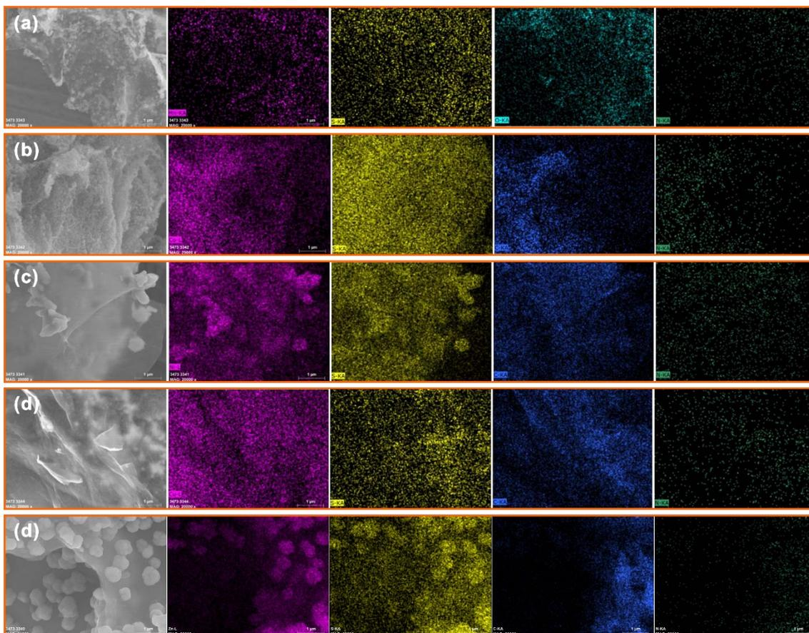
**Figure S11** SEM images and the corresponding elemental mapping images of (a) MnS@NC@G, (b) Co<sub>9</sub>S<sub>8</sub>@NC@G, (c) Ni<sub>3</sub>S<sub>2</sub>@NC@G, (d) Cu<sub>2</sub>S@NC@G, and (e) ZnS@NC@G.
