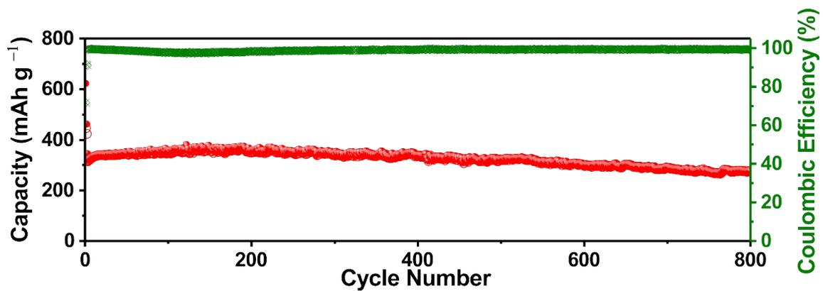
Figure S6 Cycling performance of Fe<sub>1-x</sub>S@NC@G electrode at 1 A g<sup>-1</sup> in SIB half-cell.
