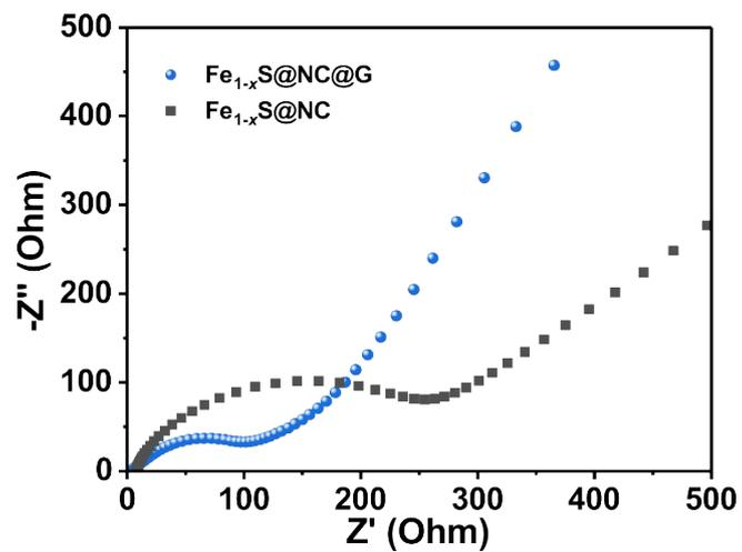
**Figure S7** EIS Nyquist plots of Fe<sub>1-x</sub>S@NC@G and Fe<sub>1-x</sub>S@NC electrodes after rate capability testing at desodiated state.
