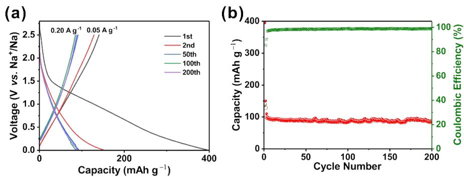
**Figure S4** Electrochemical Na storage performance of porous carbon that was obtained by removing Fe<sub>1-x</sub>S component in Fe<sub>1-x</sub>S@NC@G composite with aqua regia: (a) Representative galvanostatic discharge/charge profiles of the porous carbon at 0.2 A g<sup>-1</sup> after initial two-cycle activation at 0.05 A g<sup>-1</sup>; (b) cycling performance of the porous carbon.
