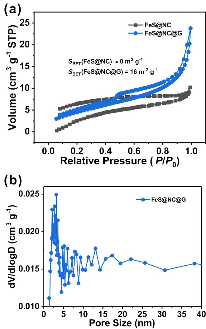
**Figure S1** (a) Nitrogen sorption isotherms of FeS@NC and FeS@NC@G composites. (b) The corresponding BJH pore size distribution of FeS@NC@G composite.
