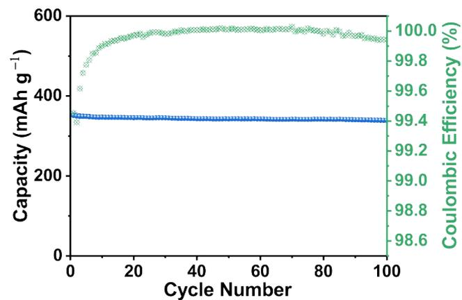
**Figure S9** Cycling performance of designed  $\text{Fe}_{1-x}\text{S}@\text{NC}@\text{G} // \text{Na}_3\text{V}_2(\text{PO}_4)_2@\text{C}$  SIB full cell (capacities are calculated based on the  $\text{Fe}_{1-x}\text{S}@\text{NC}@\text{G}$  anodic material).
