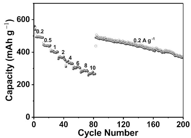
**Figure S5** Rate performance of Fe<sub>1-x</sub>S@NC electrode.
