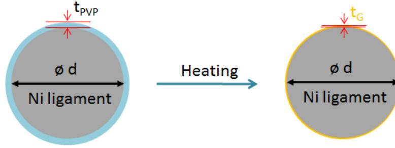
Fig. S3 Schematic of PVP coating on Ni ligament and converted to graphene (G) thin film.
