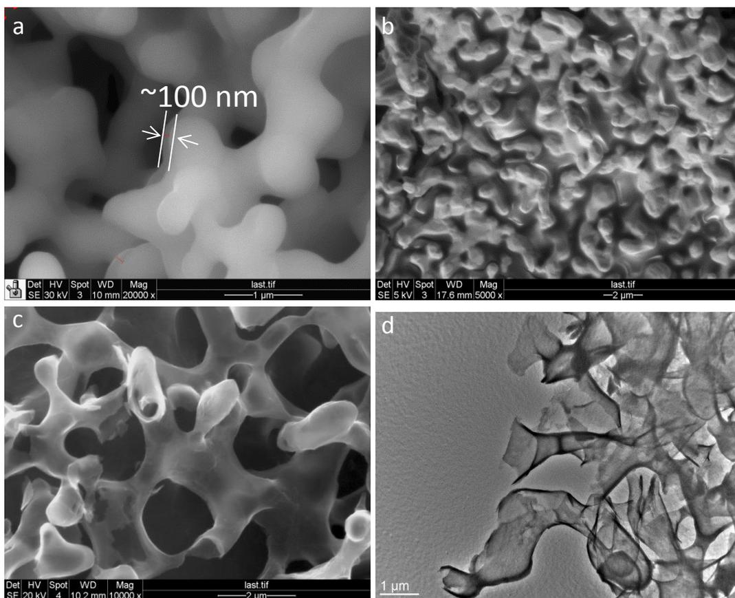
Fig. S4 (a) PVP coated nanoporous Ni by dipping the nanoporous Ni in  $0.25 \text{ g ml}^{-1}$  of PVP solution, (b) PVP coated nanoporous Ni by dipping the nanoporous Ni in  $0.4 \text{ g ml}^{-1}$  of PVP solution, (c and d) SEM and TEM of nanoporous graphene with thick walls obtained by using  $0.4 \text{ g ml}^{-1}$  of PVP solution.
