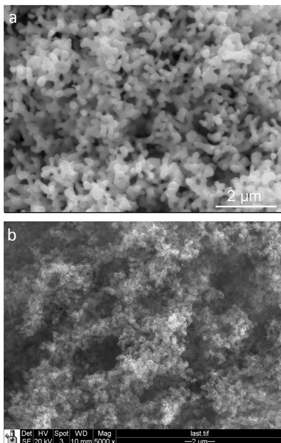
Fig. S7 (a) SEM of nanoporous Ni with average ligament size  $\sim 160$  nm, (b) low magnification SEM image of NPG-160.
