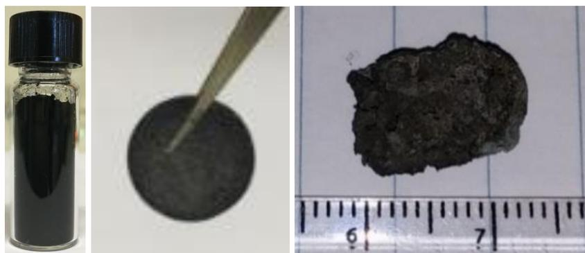
Fig. S1 Nanoporous graphene (NPG) in the forms of powder (left), chip (middle) and bulk (right).
