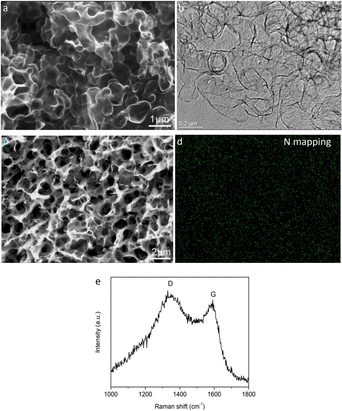
Fig. S5 (a and b) SEM image and TEM image of the NPG prepared by using sucrose as the precursor; (c and d) SEM and N mapping of NPG prepared by using PVP and dicyandiamide as carbon sources. (e) Raman spectra of N-doped NPG.
