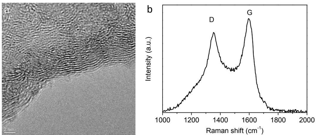
Fig. S6 (a) HR-TEM and (b) Raman spectrum of nanoporous graphene obtained at 700 °C, showing the disordered layer structure and low graphitization.
