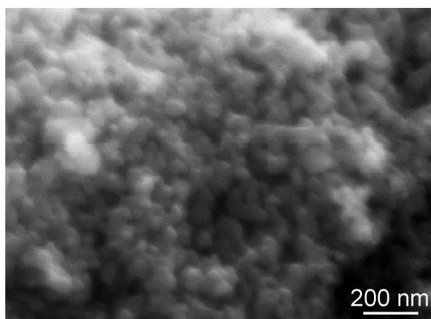
Fig. S8 SEM micrograph of nanoporous Ni with average ligament size 10-50 nm.
