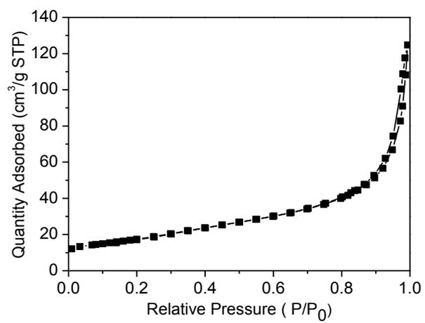
Fig. S9 Nitrogen adsorption- desorption isotherm of carbon black
