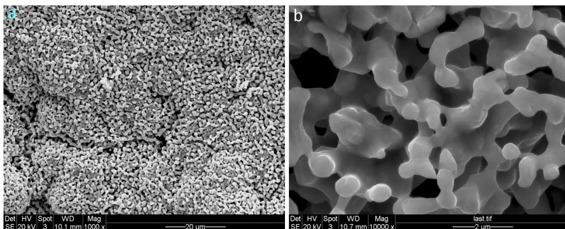
Fig. S2 SEM micrographs showing NPNi-1000 synthesized at 600 °C: (a) overview and (b) close view.
