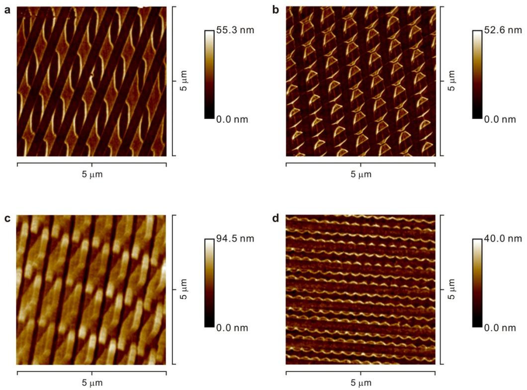
**Figure S2.** Morphologies of various patterned ZnO layers via two-step soft nanoimprinting technology under different stamping conditions. (a) 1500 nm × 1500 nm (30°), (b) 1500 nm × 1500 nm (60°), (c) 1500 nm × 1500 nm (20°), and (d) 800 × 1500 (90°).
