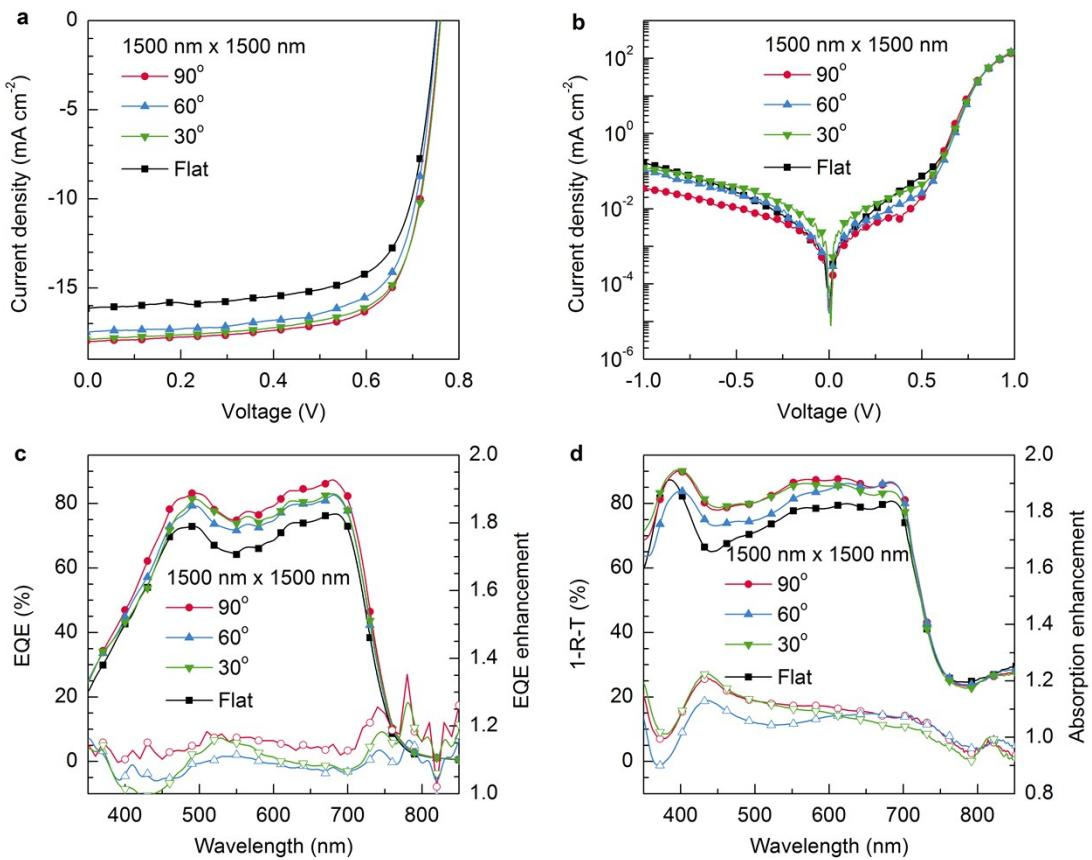
**Figure S6.** Photovoltaic characteristics of OSCs based on 1500 nm × 1500 nm dual-grating patterned ZnO layers with different angles. (a) J–V characteristics recorded under 100 mW cm<sup>-2</sup> AM 1.5G simulated solar illumination. (b) The dark J–V curves. (c) External quantum efficiency (EQE) spectra and relative EQE enhancement of patterned devices related to that of the flat one. (d) Absorption spectra and the absorption enhancement.
