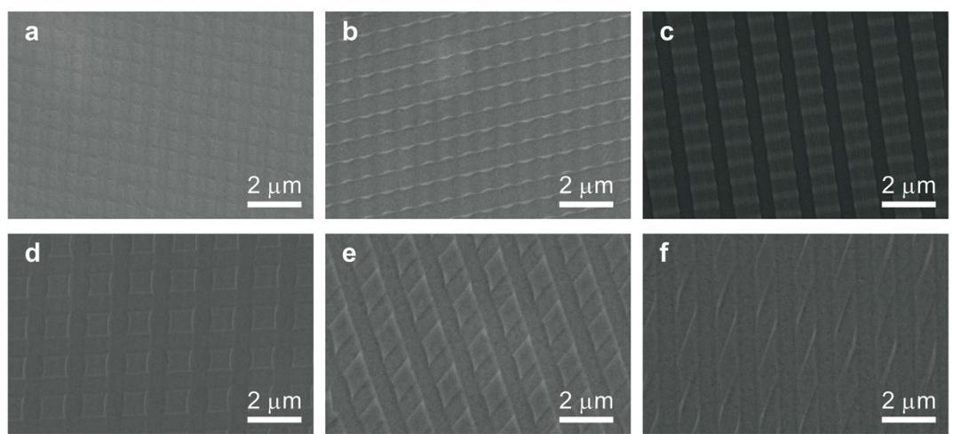
**Figure S3.** Scan electron microscope (SEM) images of PEIE-coated ZnO layers with various dual-gratings. (a) 800 nm × 800 nm, (b) 800 nm × 1500 nm, (c) 1500 nm × 800 nm, (d) 1500 nm × 1500 nm (90°), (e) 1500 nm × 1500 nm (60°), and (f) 1500 × 1500 (30°).
