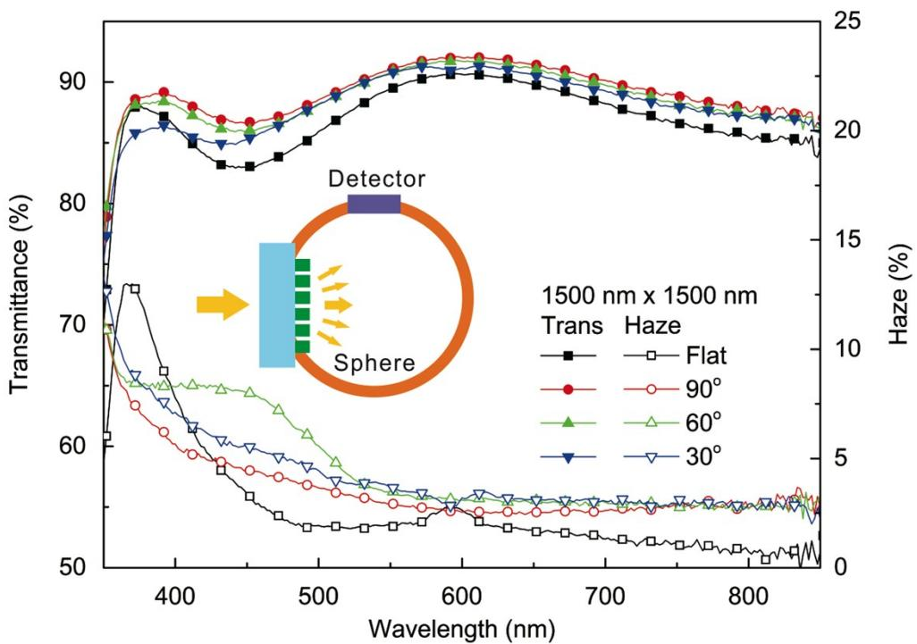
**Figure S5.** Total transmittance spectra and haze values of ITO glass substrates without and with dual-grating patterned ZnO layers, which were recorded with the incident light from the glass side. Inset depicts the optical measurement configuration using an integrating sphere.
