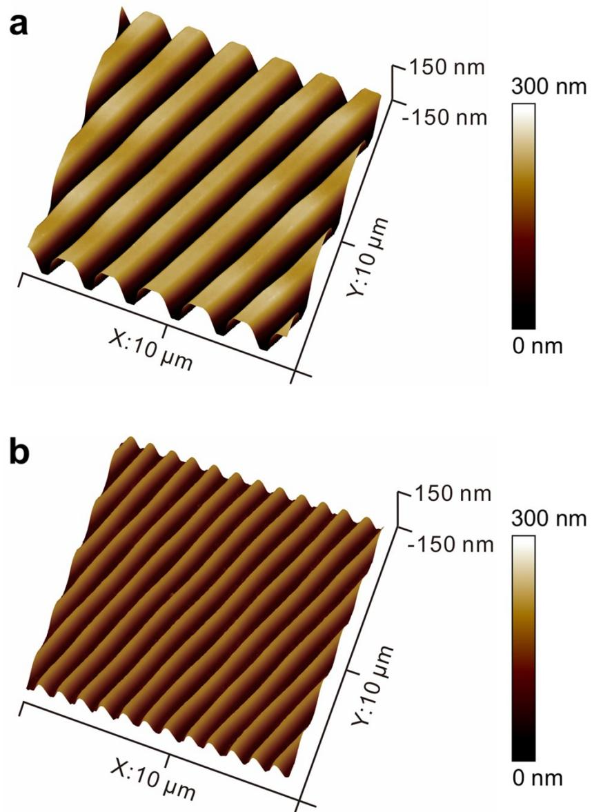
**Figure S1.** AFM images of (a) CD and (b) DVD disks used in this work.
