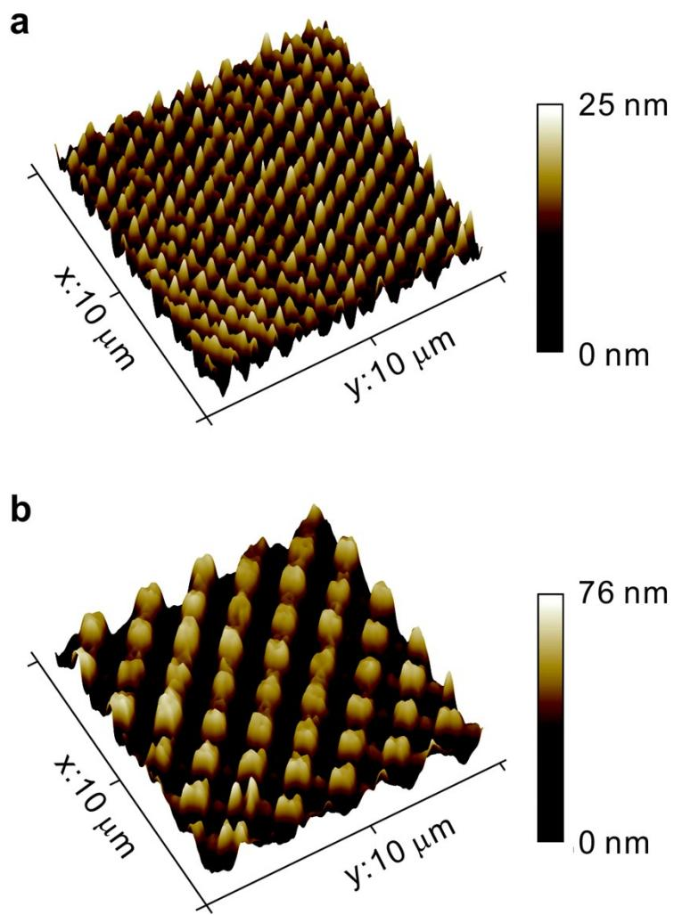
**Figure S4.** Morphologies of PTB7:PC<sub>71</sub>BM layers spin-coated on patterned ZnO layers with dual-gratings of (a) 800 nm × 800 nm and (b) 1500 nm × 1500 nm.
