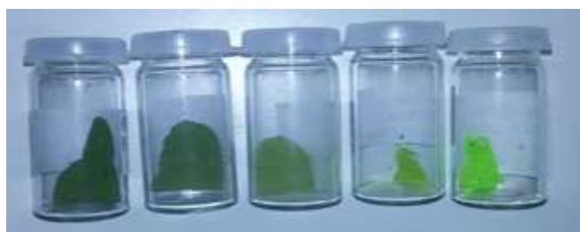
Figure SI-1. Digital image taken to display the colours of the Pt/CuClP materials depending on the Pt loading. From left to the right: 7, 5, 3 and 1 wt. % Pt/CuClP samples and the un-doped framework.
