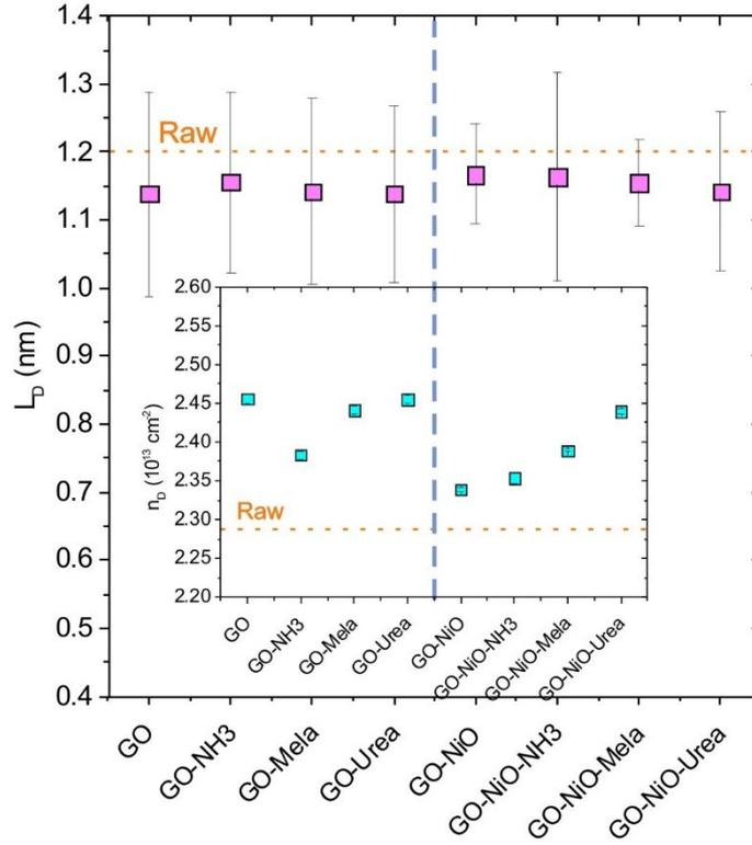
Figure S5. Mean distance between defects ( $L_D$ ) in GO-deposited materials. Inset: corresponding density of defects ( $n_D$ ).
