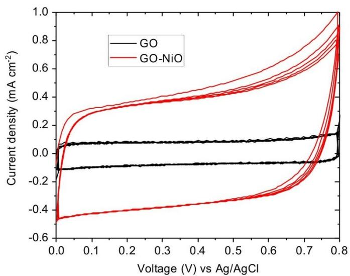
Figure S8. Additional voltammetry cycles measured at  $150 \text{ mV s}^{-1}$  scan rate of samples GO and GO-NiO.
