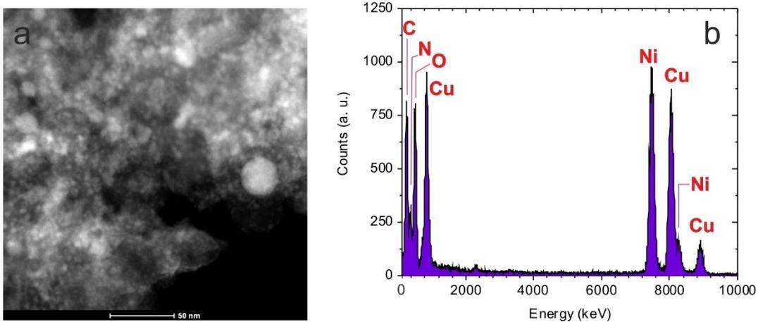
Figure S4. (a) HAADF-STEM image of GO-NiO-Melamine sample. (b) Typical EDAX spectrum of GO-NiO-Urea sample. The energy peaks are associated to their corresponding chemical elements.
