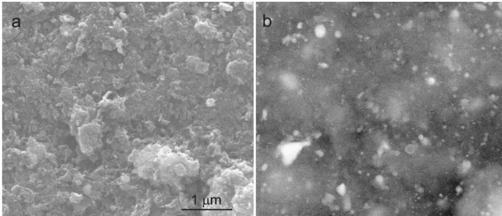
Figure S3. SEM images of GO-NiO-Melamine film. (a) Secondary and (b) corresponding backscattered electron images. The bright elements in (b) are attributed to Ni-rich regions (Ni has higher atomic number than C).
