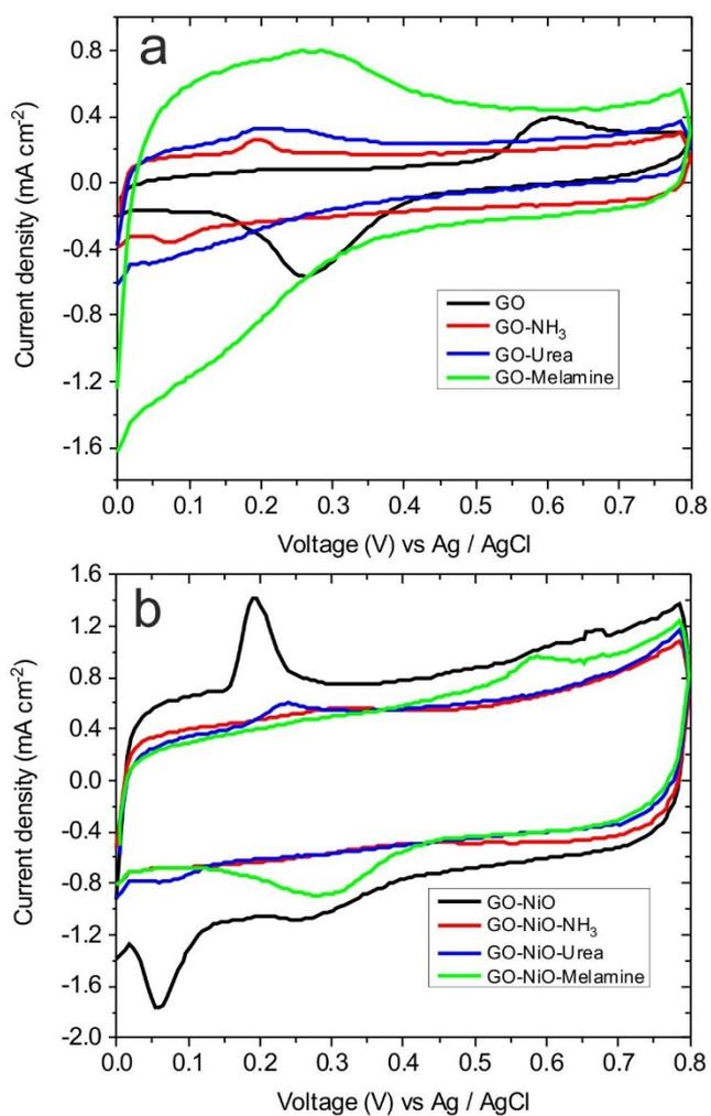
Figure S7. Cyclic voltammetry plots at a 150 mV s<sup>-1</sup> scan rate of samples deposited (a) without and (b) with NiO NPs.
