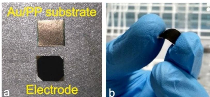
Figure S1. (a) Image of Au/Cr/PP substrate and GO/Au/Cr/PP electrode. (b) The electrodes are highly flexible.
