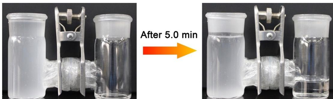
**Fig S5** Digital photos of an H-shaped separation device at  $t = 0$  and  $t = 5.0$  min after the addition of 50 mL of nanoemulsion NE1 into the left feed cell.
