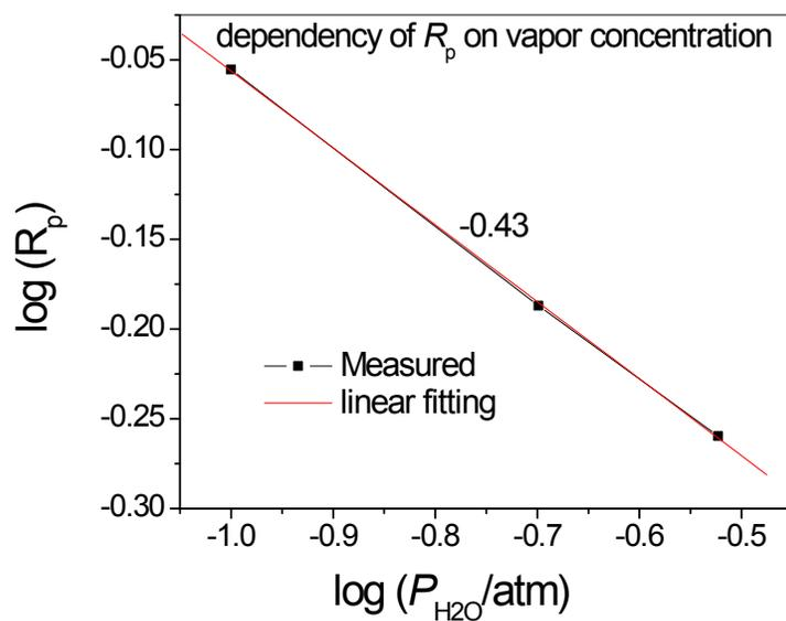
Fig. S5 Dependency of polarization resistance of PNO-BZCY anode on  $P_{H_2O}$  at 550°C measured at OCV.
