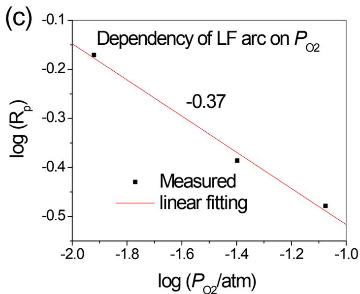
Fig. S6 (a) Measured and fitted EIS of PNO-BZCY anode in 60% vapor with varying  $P_{O_2}$  at 550°C under OCV, these spectra are fitted into a two-arc profile using the equivalent circuit in the inset; (b) reaction order of the fitted HF arc resistance on  $P_{O_2}$ ; (c) reaction order of the fitted LF arc resistance on  $P_{O_2}$
