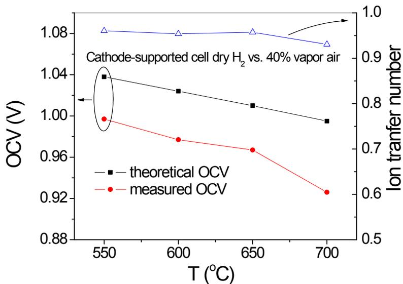
Fig. S4 Measured and calculated OCV of the cathode-supported full cell, the ion transport number is around 95%, proving negligible electronic and gas leakage through the thin BZCY electrolyte layer.
