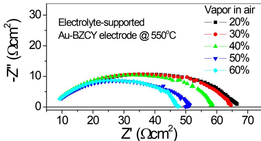
Fig. S3 Progressively decreasing polarization resistance of inert Au-BZCY electrode on BZCY electrolyte, measured in parallel experiment with PNO. No resistance saturation was observed.
