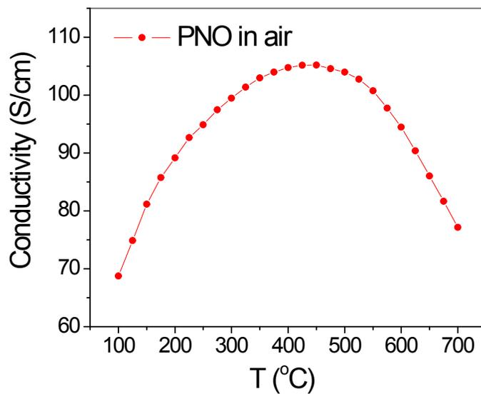
Fig. S2 electrical conductivity of PNO measured in dry air.
