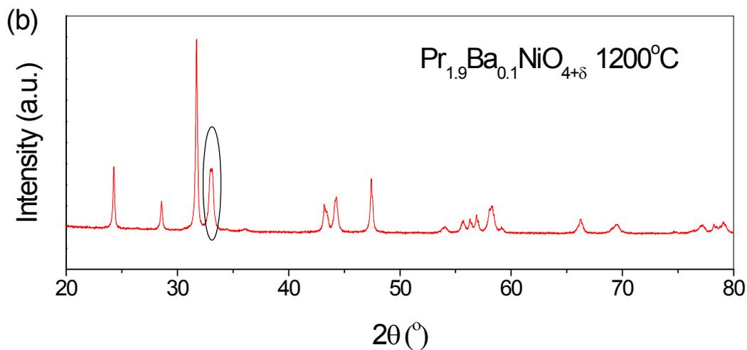
Fig. S1 (a) Interaction between PNO and GDC after heating at 800°C for 4h. Instead of symmetry change from orthorhombic to tetragonal, the  $\text{A}_{n+1}\text{B}_n\text{O}_{3n+1}$  RP phase evolves from low order to high order form, accompanied by release of simple praseodymium oxide, (b) orthorhombic to tetragonal symmetry transition when 5% Ba is doped at A site, note that the double peak at 33° in orthorhombic turns to single peak in the tetragonal symmetry.
