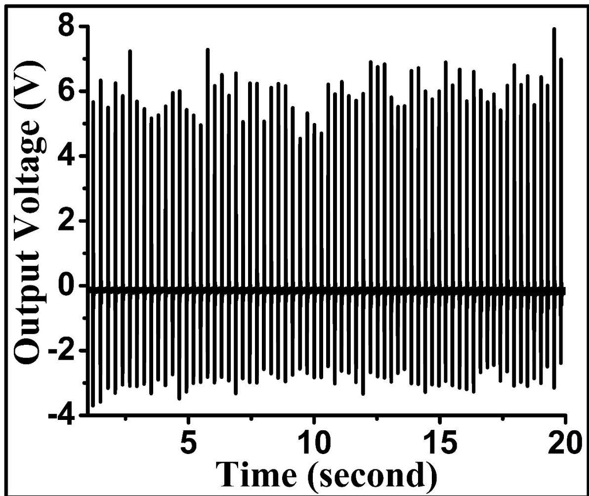
**Figure S2: Open circuit output Voltage of pure PVDF thin film based piezoelectric nanogenerator.**
