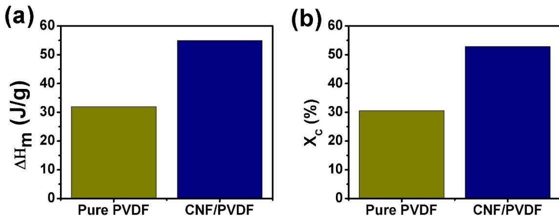
**Figure S1:** (a) Enthalpy of pure PVDF and CNF/PVDF composite thin films. (b) Crystallinity of pure PVDF and CNF/PVDF composite thin films.
