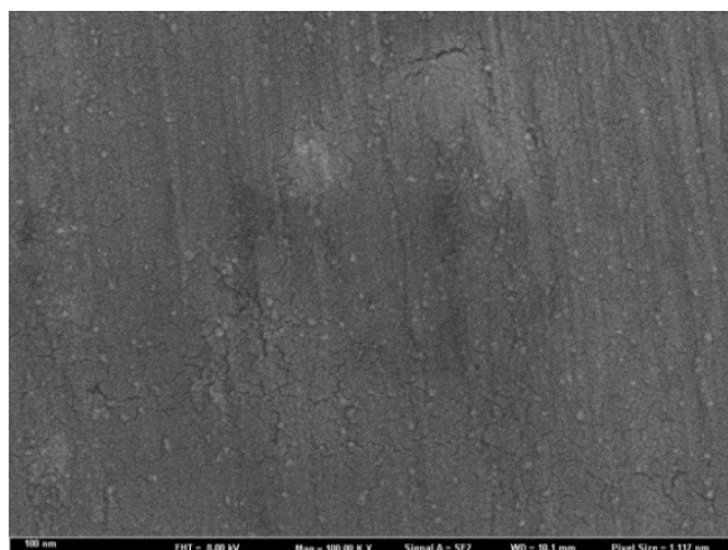
Figure S5. Surface morphology of CoAl-LDH composite membranes after wipe off. (Preparation conditions: \text{Co}(\text{NO}_3)_2 \cdot 6\text{H}_2\text{O} , 21 mmol/L; \text{Al}(\text{NO}_3)_3 \cdot 9\text{H}_2\text{O} , 7 mmol/L; urea, 70 mmol/L; and \text{NH}_4\text{F} , 100 mmol/L; reaction temperature, 110 °C; reaction time, 24 h)
