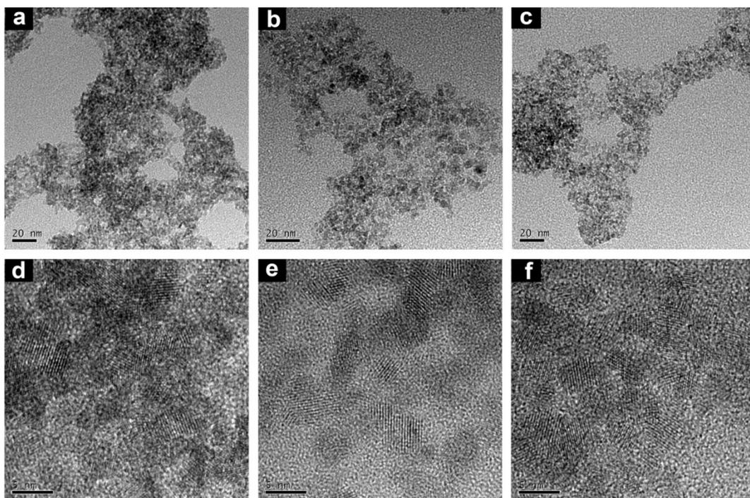
**Fig. S1.** TEM images of (a) n-SnO<sub>2</sub> nanoparticles, (b) fresh TMAH-modified SnO<sub>2</sub> nanoparticles and (c) TMAH-modified SnO<sub>2</sub> store for 12 hs. (d), (e) and (f) are the corresponding HRTEM images of (a), (b) and (c), respectively.
