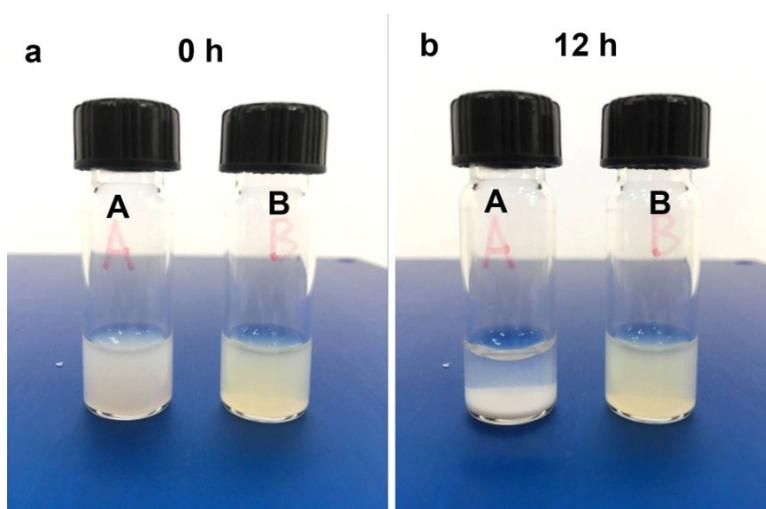
**Fig. S2.** Dispersion of SnO<sub>2</sub> nanoparticles at 0 h and 12 h. A without TMAH; B with TMAH modification.
