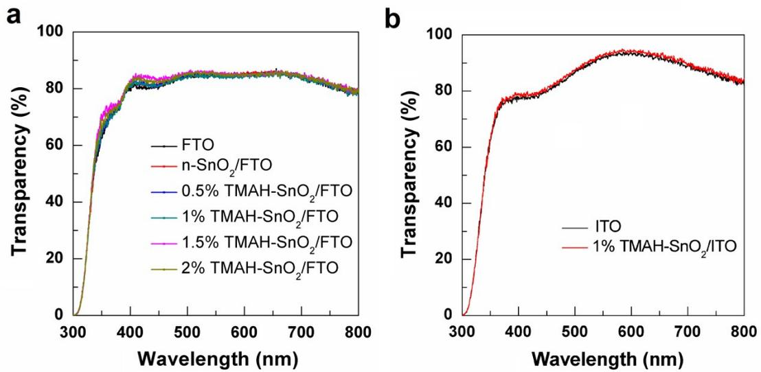
**Fig. S5.** Optical transmittance of the (a) bare FTO and SnO<sub>2</sub> coated FTO substrates, and (b) bare ITO and SnO<sub>2</sub> coated ITO substrates.
