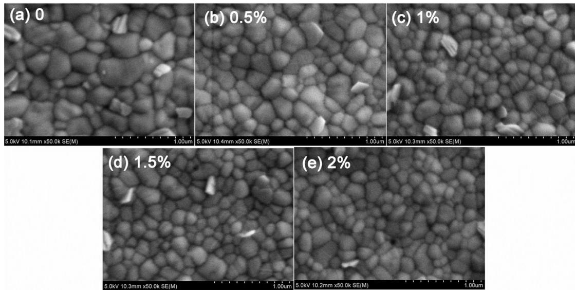
**Fig. S7.** Surface SEM images for perovskite deposited on (a) n-SnO<sub>2</sub>, (b) 0.5% TMAH-SnO<sub>2</sub>, (c) 1% TMAH-SnO<sub>2</sub>, (d) 1.5% TMAH-SnO<sub>2</sub> and (e) 2% TMAH-SnO<sub>2</sub>, respectively.
