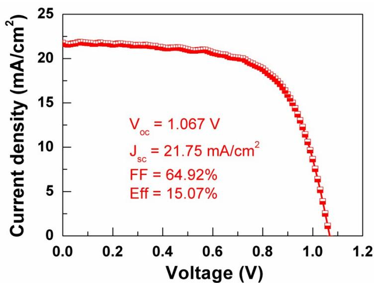
**Fig. S9.** *J-V* curve of a flexible TMAH-SnO<sub>2</sub> based device constructed on ITO/PEN substrate, showing an efficiency of about 15.07%.
