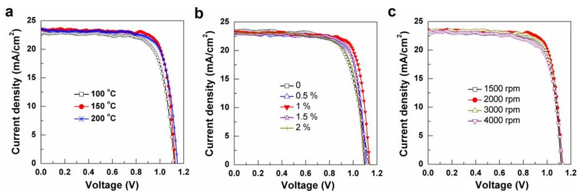
**Fig. S4.** Optimization of the ETL deposition process. The (a) annealing temperature, (b) TMAH concentration, and (c) spin-coating speed dependent performance of the PSCs. It can be learned that 1 % concentration of TMAH, 2000 rpm of spin coating rate, and 150 °C of annealing temperature is optimized for efficient devices.
