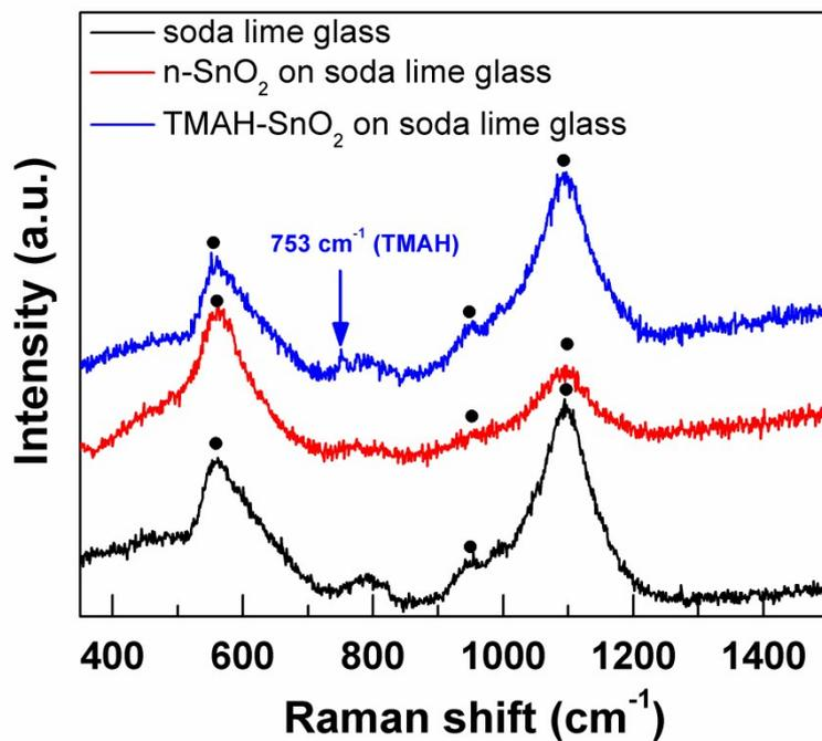
**Fig. S3.** Raman spectra of soda lime glass substrate (black line), n-SnO<sub>2</sub> on soda lime glass (red line), and TMAH-SnO<sub>2</sub> on soda lime glass. The dark dot indicate the Raman shift for soda lime glass. Peak located at about 753 cm<sup>-1</sup> is a signal of TMAH.
