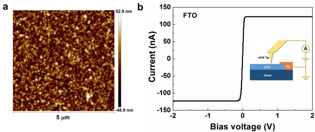
**Fig. S6.** (a) Morphology and (b) *I-V* curve of a FTO substrate from c-AFM measurement, showing ohmic contact between the tip and the FTO electrode.
