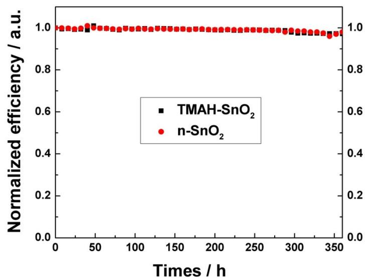
**Fig. S8.** Stability tests for n-SnO<sub>2</sub> based and TMAH-SnO<sub>2</sub> based devices sealed with resin. Devices were stored in desiccator under relative humidity of about 15%.
