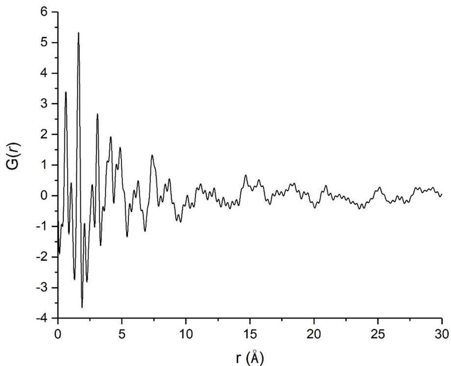
Figure 3.a. Pair distribution function,  $G(r)$  data for Ge-UTL after hydrolysing for 8 hr in water at 100 °C. No peaks are observed after 12 Å, due to a lack of long-range order.
