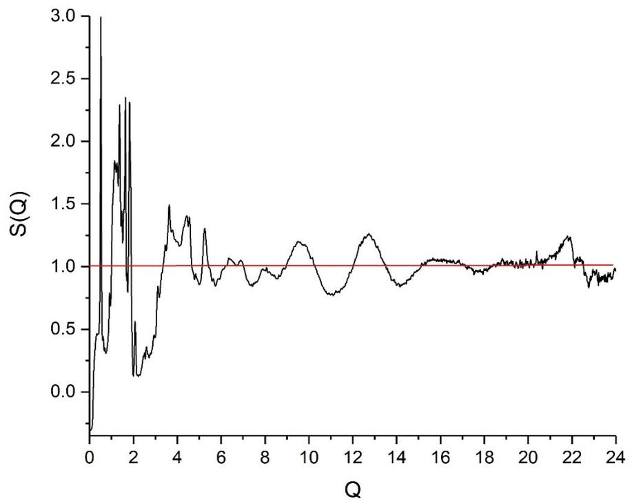
Figure 2.c.  $S(Q)$  data for Ge-UTL in 12 M hydrochloric acid after hydrolysing for 12 hr at 50 °C.  $S(Q)$  data oscillates around 1.
