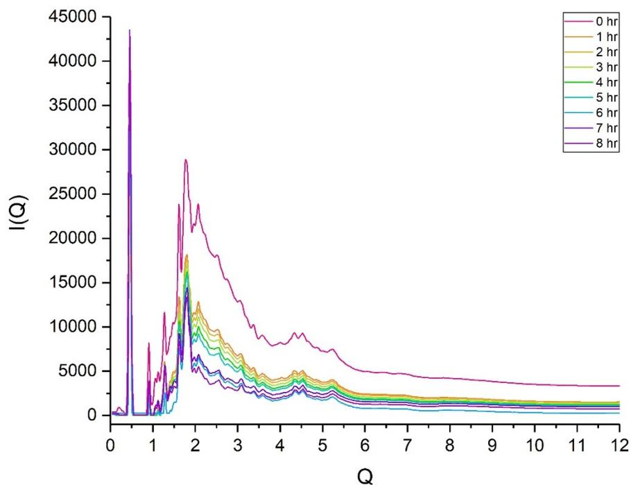
Figure 1.a. Initial  $I(Q)$  data for Ge-UTL in water after hydrolysing for 8 hr at 100 °C. Data cut to  $Q = 12$  to show the tail off of realistic data and key features  $<7$ . Where  $I(Q) = I_{\text{coh}}(q) + I_{\text{incoh}}(q)$ .
