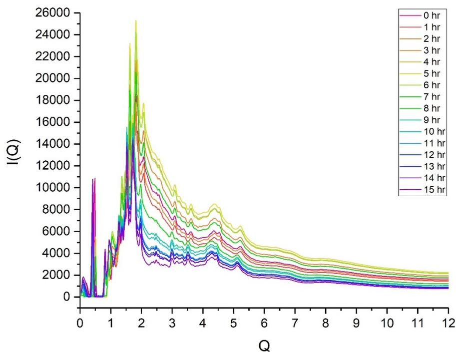
Figure 1.b. Initial  $I(Q)$  data for Ge-UTL in 6 M hydrochloric acid after hydrolysing for 15 hr at 100 °C.
