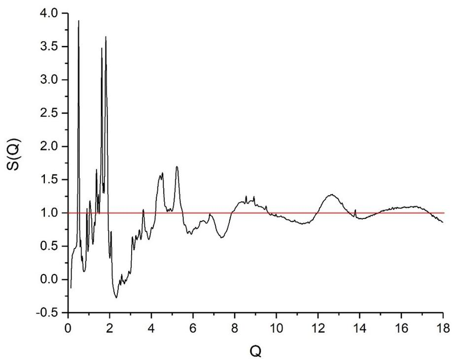
Figure 2.b.  $S(Q)$  data for Ge-UTL in 6 M hydrochloric acid after hydrolysing for 15 hr at 100 °C.  $S(Q)$  data oscillates around 1.
