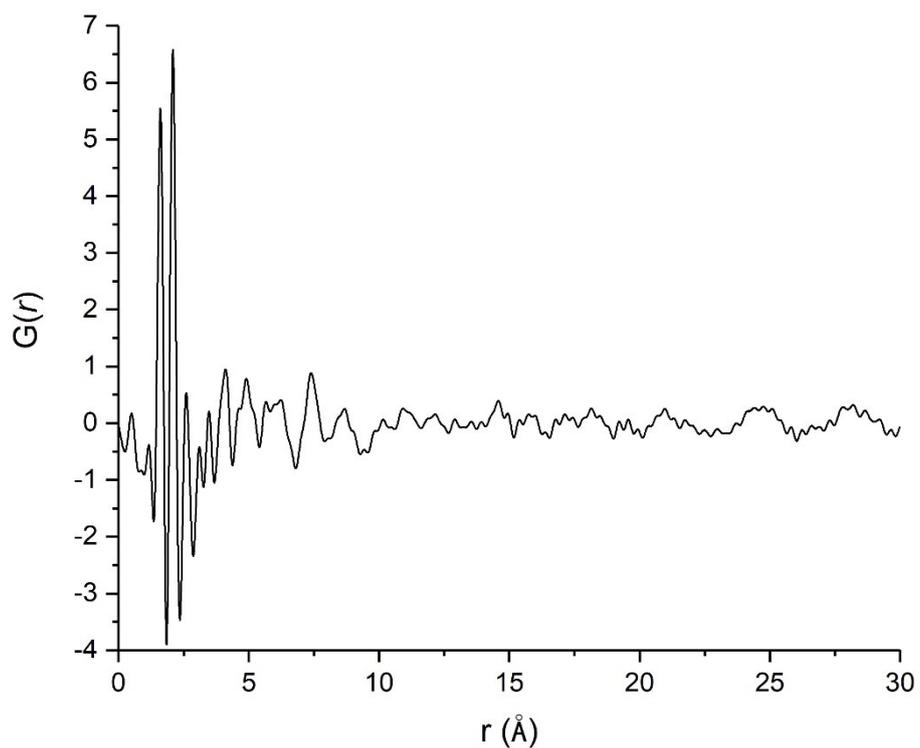
Figure 3.c. Pair distribution function,  $G(r)$  data for Ge-UTL after hydrolysing for 12 hr in 12 M hydrochloric acid at 50 °C. No peaks are observed after 12 Å, due to a lack of long-range order.  $G(r)$  has minimal features at unphysical distances ( $r < 1$  Å).
