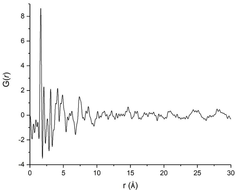
Figure 3.b. Pair distribution function,  $G(r)$  data for Ge-UTL after hydrolysing for 15 hr in 6 M hydrochloric acid at 100 °C. No peaks are observed after 10 Å, due to a lack of long-range order.  $G(r)$  has minimal features at unphysical distances ( $r < 1$  Å).
