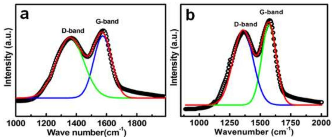
**Fig. S5** Typical Raman spectra of (a) H-ZFO-C and (b) H-ZFO-C@void@C products
