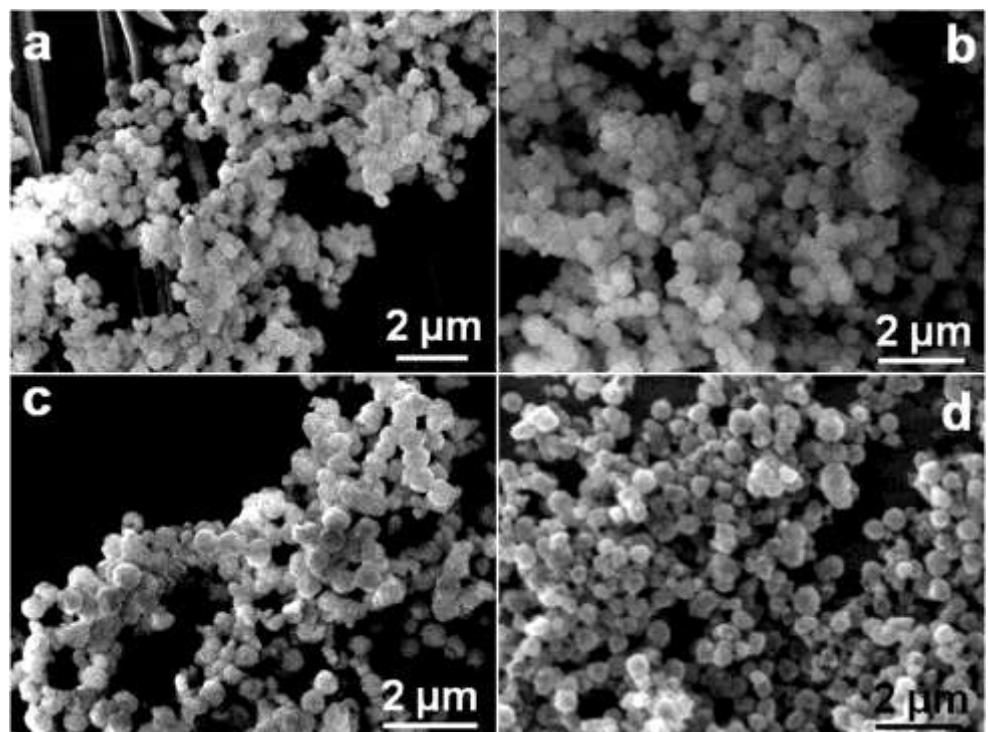
**Fig. S7** Typical FESEM images of (a) H-ZFO-O@SiO<sub>2</sub>, (b) H-ZFO-O@SiO<sub>2</sub>@PDA, (c) H-ZFO-C@SiO<sub>2</sub>@C and (d)H-ZFO-C@void@C products
