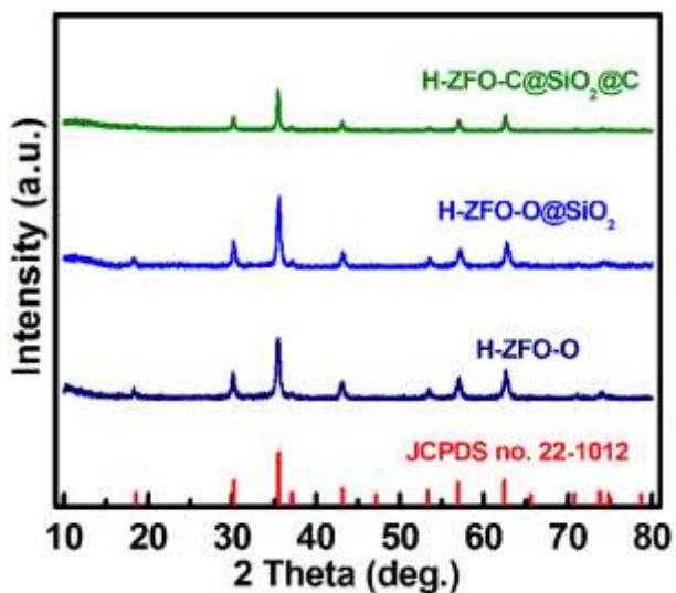
**Fig. S2** XRD pattern of the H-ZFO-O, H-ZFO-O@SiO<sub>2</sub> and H-ZFO-C@SiO<sub>2</sub>@C samples as indicated
