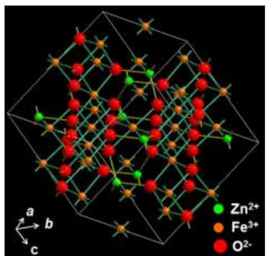
**Fig. S4** Crystallological structure of the spinel ZFO
