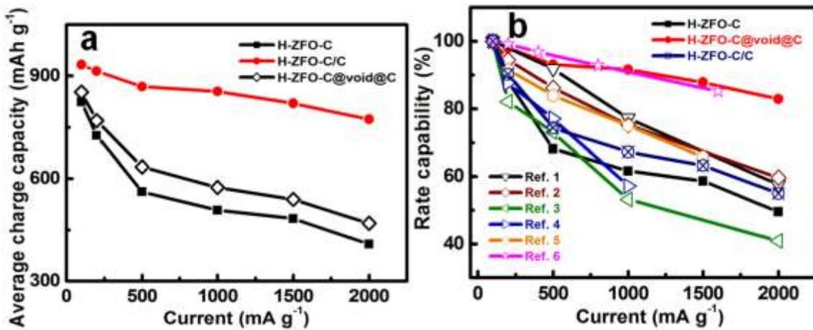
**Fig. S8** (a) Capacities of the H-ZFO-C, H-ZFO-C/C and H-ZFO-C@void@C anodes as a function of current density, and (b) comparison in rate capability of the H-ZFO-C, H-ZFO-C/C and H-ZFO-C@void@C with other ZFO/C composite anodes
