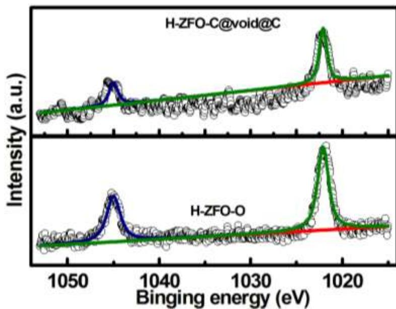
**Fig. S6** Zn XPS spectrum for the H-ZFO-O and H-ZFO-C@void@C products
