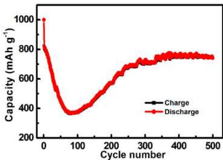
**Fig. S9** Cycvling performance of the H-ZFO-C/C electrode at a current density of  $1000 \text{ mA g}^{-1}$
